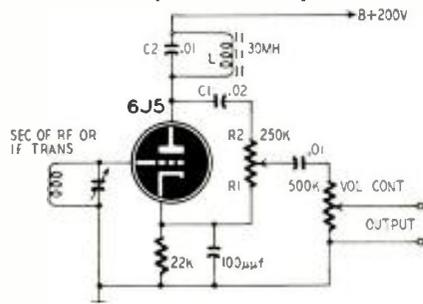
from a bridge composed of the internal resistance of the tube, C1, R1, and R2. At frequencies above and below the resonant frequency of L-C2, the plate-circuit impedance is low and most of the audio voltage is developed in the cathode circuit. If R1 and R2 are equal and the reactance of C1 is low, the output voltage will be half that developed in the cathode circuit. If the impedance
