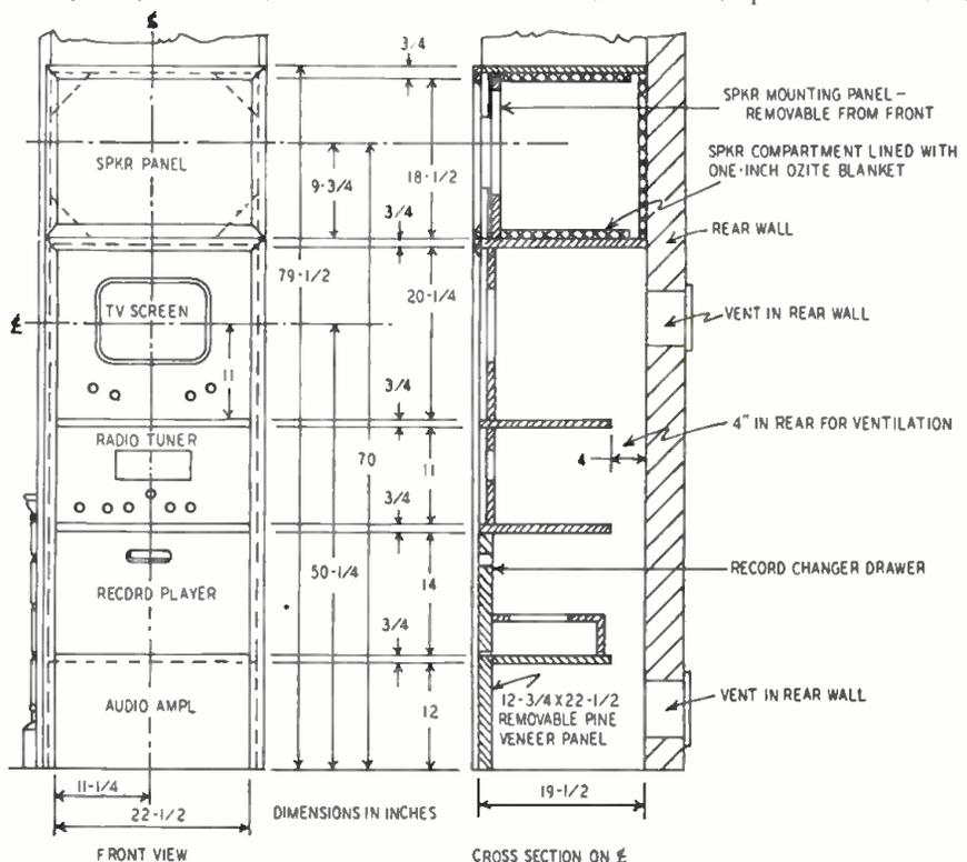
Fig. 2—A front-panel view and cross-section of the installation in Fig. 1.
