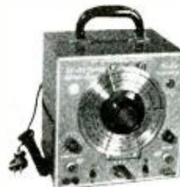
television and FM sweep generators. Calibration accuracy is within 1%. A self-contained crystal oscillator may be used simultaneously with the v.f.o. or by itself. A phasing control is included. An internal mixing circuit is arranged so that the output of a sweep generator may be fed to the TV-50 and the marker's output leads carry both signals.
