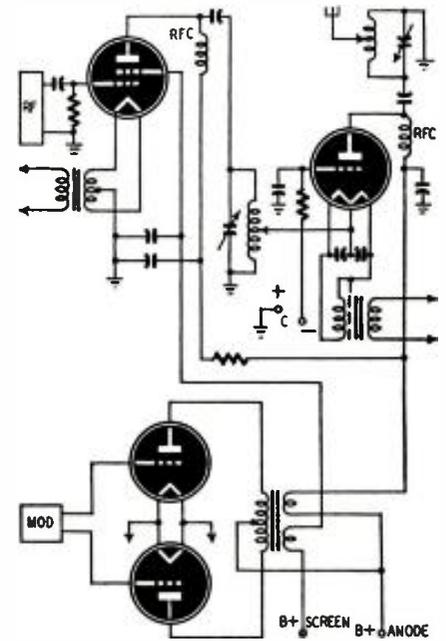
The modulation transformer has two secondaries. One modulates the exciter screen; the other modulates the plates. The audio voltages applied to the exciter elements should be proportional to their d.c. potentials for lowest distortion. The final filament transformer should have adequate shielding for low capacitance to ground, since the filaments are at an r.f. potential above ground.
