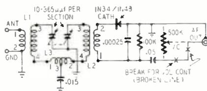
The 1N34 or 1N48 crystal diode detector develops between .05 and 0.5 volt on stations within a 20-25-mile radius when used with a good outside antenna 75 to 100 feet long. L1 and L2 are Miller 242-A antenna coils, and L3 is a type EL-55 negative mutual coupling coil.
