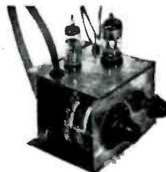
NEW 13 CHANNEL TUNER is a small compact unit with stage of R.F. Tunes all TV and ZFM channels. Made to conform with Telekit or any other TV set having video I.F. of 25.75 Mc. Complete with tubes, pre-wired pre-aligned; only three connections to make. See your jobber, or write to us for information. Your cost, \$19.95.
