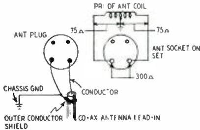
quality will be improved if the unused part of the coil is shorted out by grounding the remaining terminal. This connection can be made on the antenna plug by connecting the co-ax across the 300-ohm terminals and grounding the outer conductor to the chassis as shown in the drawings.
