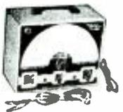
A top quality signal generator for every servicing need. Can be used for FM, AM alignment and to provide TV marker frequencies. Range 150 kc. to 100 mc in 6 bands, with fundamentals to 34 mc. Pure 400 cycle audio by a composite type audio oscillator. Easy to follow schematic diagrams included. Complete with tubes.
