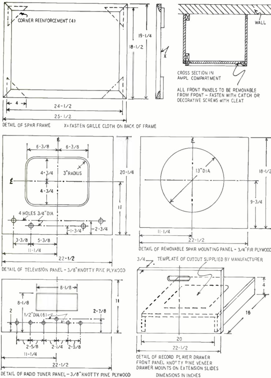
Fig. 3—Details of the panels on the individual compartments. The over-all dimensions and the positions of the holes will vary with different chassis sizes.
