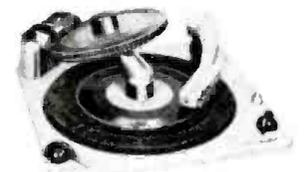
r.p.m. All records are changed by the edge-push-off method. Two spindles are furnished, one with the standard diameter for ordinary records and the other with a diameter of 1½ inches for RCA 45-r.p.m. discs. A two-stylus crystal cartridge with tilt adjustment plays all records with a stylus force of 6 to 8 grams. A velocity trip is used.
