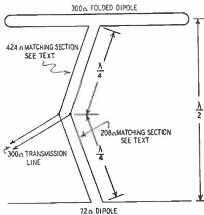
The electrical length of the quarter-wave section can be calculated from
