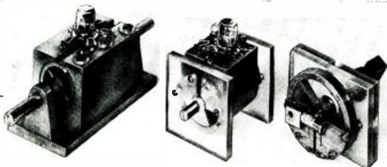
ture transmission. The Institute's Department of Electrical Engineering has developed three new u.h.f.-to-v.h.f. converters which are both simple and inexpensive. With such a converter, a standard receiver will need no internal modifications to receive u.h.f. programs.
