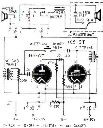
The circuit is given in the diagram. The TALK-LISTEN switch is a five-circuit three-position rotary. The center OFF position disconnects the batteries to save power. Note that if the remote buzzes the master when the three-position switch is not at OFF, the battery current will go through either the input or output transformer. It may burn up the transformer and will certainly discharge the buzzer battery. Between calls, therefore, the switch should always be set at OFF.—F. D. Crisp
