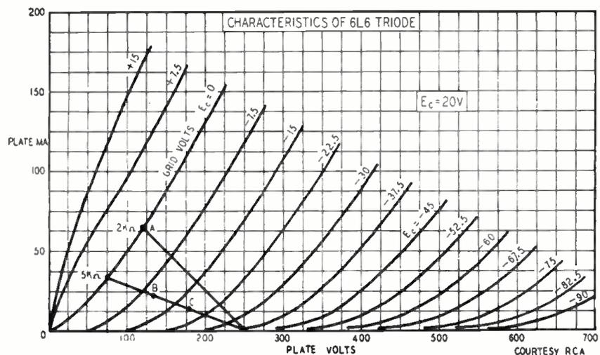
Fig. 4—Load lines compare performance of plate- and cathode-loaded amplifiers.
