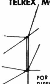
Bi-Directional Stacked Conical "V" Beam
