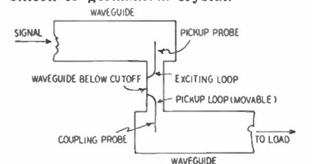
Fig. 2—Attenuator between waveguides.
