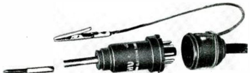
Fig. 3—Tubing is soldered to grid cap and a wire tip is slipped into tubing.
