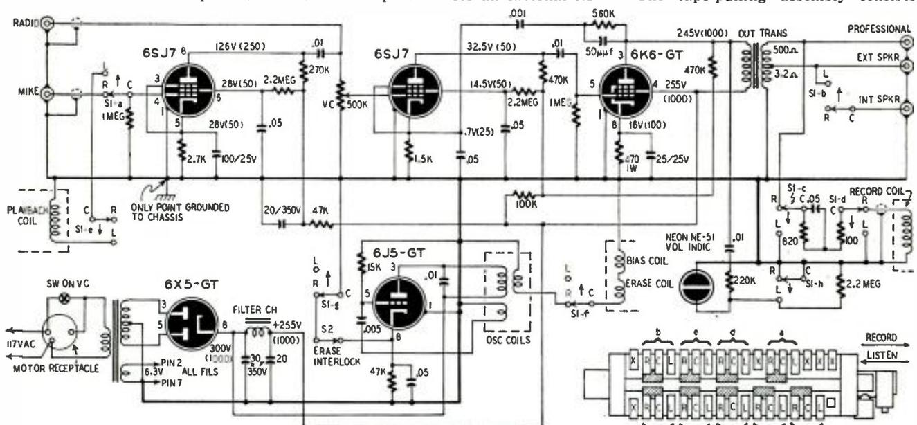
VOLTAGES MEASURED ON 20,000Ω PER VOLT METER SET TO RANGES INDICATED IN PARENTHESES THUS (1000)
