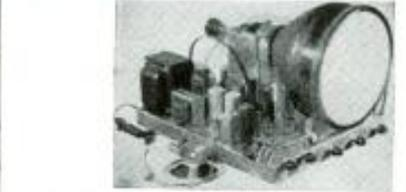
Note simple clean lay-out for easy assembly of new Telekit 10-B. Features 2 sound I. F. stages, a new pre-built, pre-aligned tuner that includes a stage of R. F. for distance reception. Easy-to-adjust horizontal lock circuits. Beautiful new model cabinets for 7-B and 10-B are heavily constructed of hand rubbed walnut.
