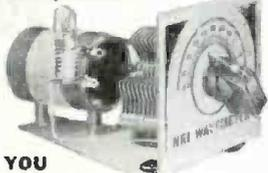
**YOU BUILD** this Wavemeter and use it to determine frequency of operation, make other tests on transmitter currents.
