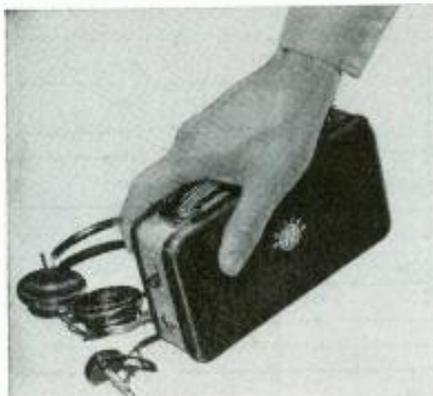
Nuclear "Sniffer" uses vibrator power supply.
