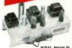
**YOU BUILD** this Transmitter Power Supply used in the basic experiments in RF and AF amplifiers, frequency multipliers, buffers, etc.
