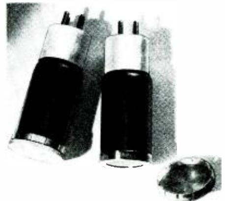
Tracerlab tubes with removable beta shields.
