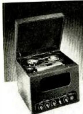
Model CL-10, which will accommodate messages from 4 seconds to 10 minutes, operates on the same principle, but utilizes a storage system with lower inherent friction, accomplished through the use of ball-bearing rollers.
