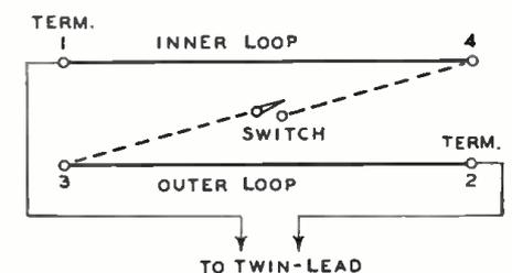
Fig. 4—Diagram of above with loops extended.
