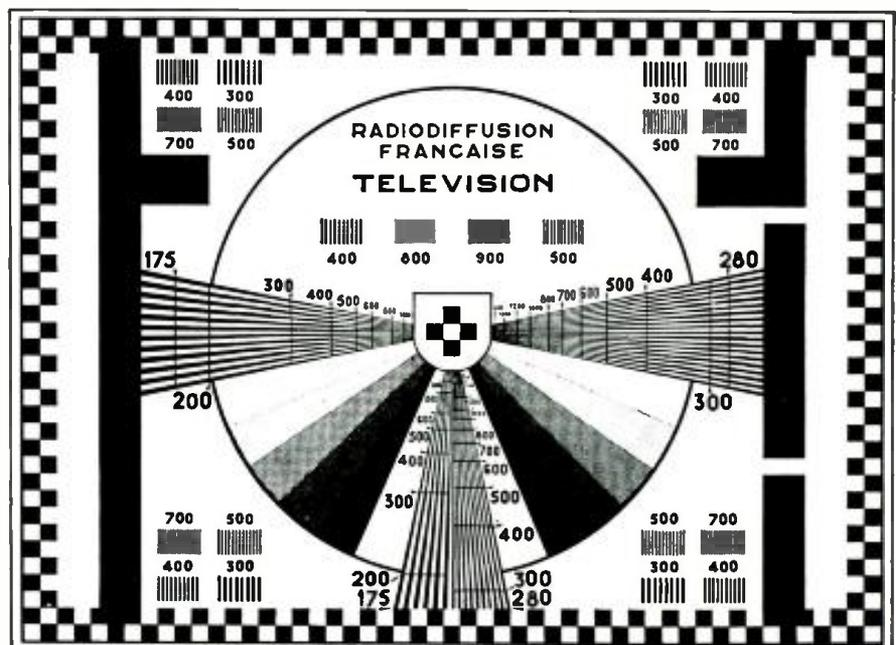
French test pattern is suitable for use with any system. Variety of markings aids testing.
