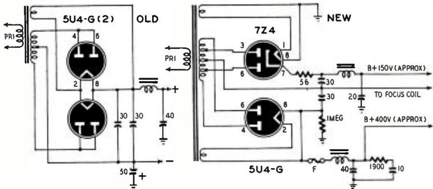
Fig. 4—Old Philco design used two similar rectifier tubes. New circuit appears at right.
