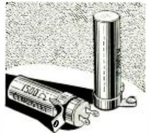
cement, and provided with bottom terminals and mounting bracket. The lugs are locked into the tube wall in addition to being sealed in cement. By having this power resistor mounted above the chassis, the problem of heat dissipation is neatly solved.
