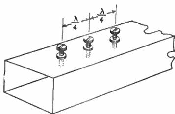
Fig. 4—Tuning screws for varying reactance.
