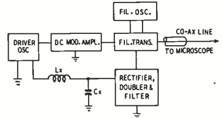
Fig. 5—Block diagram of 60-kv power supply.
