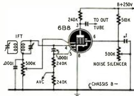
The screen voltage is supplied by a voltage divider consisting of a 240,000-ohm resistor and a 500,000-ohm potentiometer. This control can be adjusted to a point at which noise cannot exceed the signal level.
