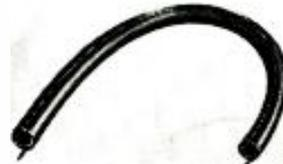
conductors. The new tubular 300-ohm Twin-Lead made especially for reception (like the tubular transmitting lines introduced by the company last year) has the conductors separated mainly by the enclosed air space within the tube. Thus dirt collecting on the outside of the tube does not lie between the conductors and has little effect on electrical characteristics. Additional features are lower wind resistance and greater strength.
