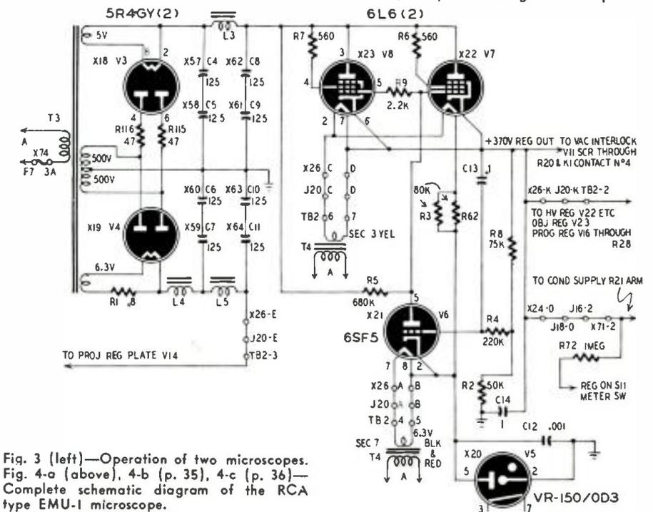
Fig. 3 (left)—Operation of two microscopes. Fig. 4-a (above), 4-b (p. 35), 4-c (p. 36)—Complete schematic diagram of the RCA type EMU-1 microscope.
