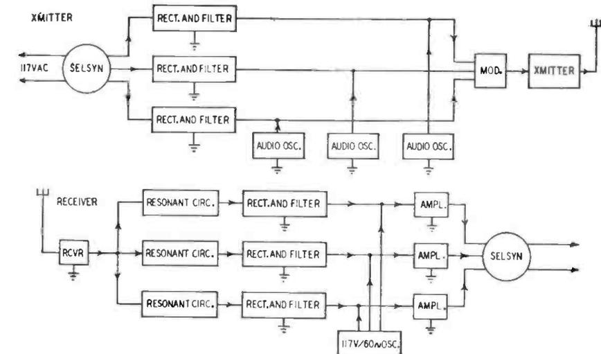
rate outputs from a 60-cycle oscillator. These three a.c. voltages are proportional to those obtained from the Selsyn at the transmitter. After amplification, they are fed to the second Selsyn which will assume the same angular position as the first.
