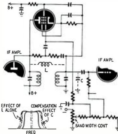
When the bandwidth control (see figure) is set near the grounded end, the gm of the reactance tube is high. This results in a higher  $I_p$  for a given  $E_g$  and is equivalent to a lower effective L and more loading across this effective inductance. The lower inductance increases the coupling between stages, but the double-hump response does not appear because of the added loading.
