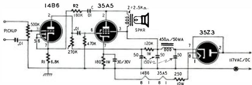
Feedback is applied from plate of the second stage to cathode of first through C and R2.
