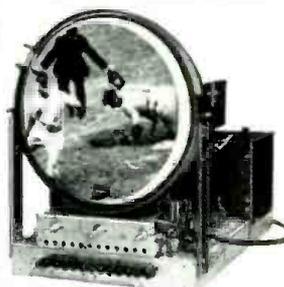
A complete direct-view chassis for 10 or 12-inch tubes. With new Dual-Focus switch—10" tube gives you choice of big 64 sq. in. view for dramatic closeups, or large 56 sq. in. full-range view. Features: 12 channel push-button tuning; RF amp; 3 IF amps; 2 video amps; improved sync circuits; AGC; static-free FM audio system. Complete with power supply, speaker, picture tube and 19 tubes, plus 3 rectifiers. For 105-125 v., 50-60 cy. AC. Shpg. wt., 60 lbs.
