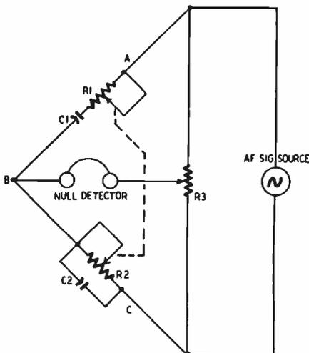
Fig. 1—Basic Wien frequency bridge circuit.
