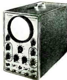
The Heathkit 5" Oscilloscope fulfills every servicing need. The husky cased power transformer supplies 1100 Volts negative and 350 Volts positive. Tubes supplied are two 6SJ7 amplifiers, 884 sweep generator, two 5Y3 rectifiers, and 5BP1 CR tube. Grey crackle aluminum cabinet and beautiful grey and maroon panel. Chassis especially designed for easy assembly.
