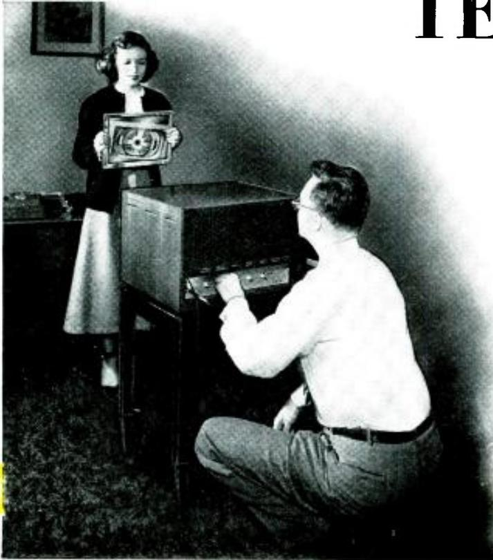
When you adjust the rear-panel controls, have someone hold a mirror so you can see how adjustments are affecting the picture. Large mirror is best.
