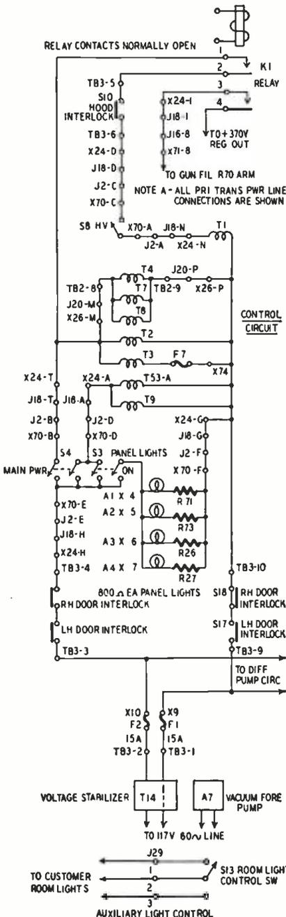
Fig. 4c—The microscope control circuits.
