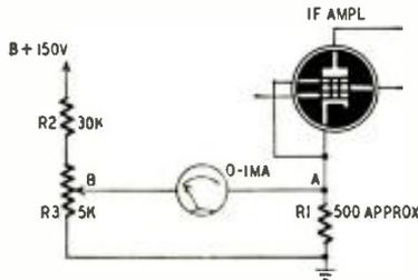
ing it read upward. Sensitivity can be controlled by adjusting the arm of the potentiometer. Values on the diagram are for an i.f. stage using a 6K7, 6SK7, or similar tube. The voltage for the bleeder should be taken from a 150-volt point in the receiver.
