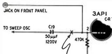
BREAK EXISTING CONNECTION AT X AND INSERT SWITCH
