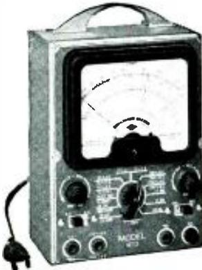
**SUPER METER.** A Combination VOLT - OHM - MILLIAMMETER plus CAPACITY REACTANCE, INDUCTANCE and DECIBEL MEASUREMENTS.
