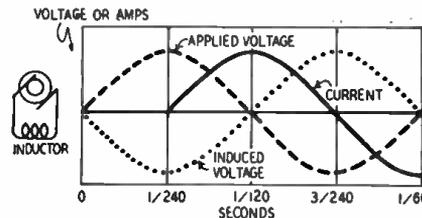
Fig. 2—Phase relations in inductive circuit.
