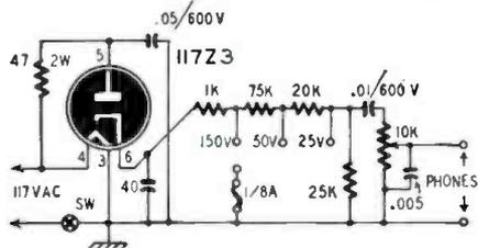
volume control all the way down until the electrolytic connections are made or else an annoying click jars your eardrums. If the hum diminishes the capacitor is good; if not, discard it. All ground returns for the electrolytics under test are made through 1/8 ampere fuse for protection against completely shorted capacitors.
