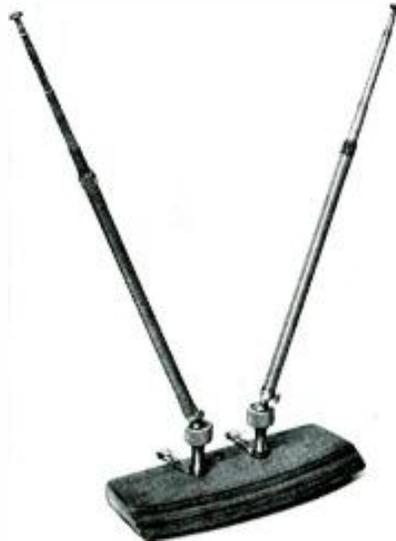
The antennas used are commonly available on the surplus market. However, if these are not obtainable, collapsible automobile antennas can be used. The ball-and-socket fittings, purchased from a hardware supply house, are similar to those used on some types of casement windows. We used hardwood for the base. Any insulating material will work just as well. The underside of the base should be covered with a layer of felt or fitted with small rubber feet.
