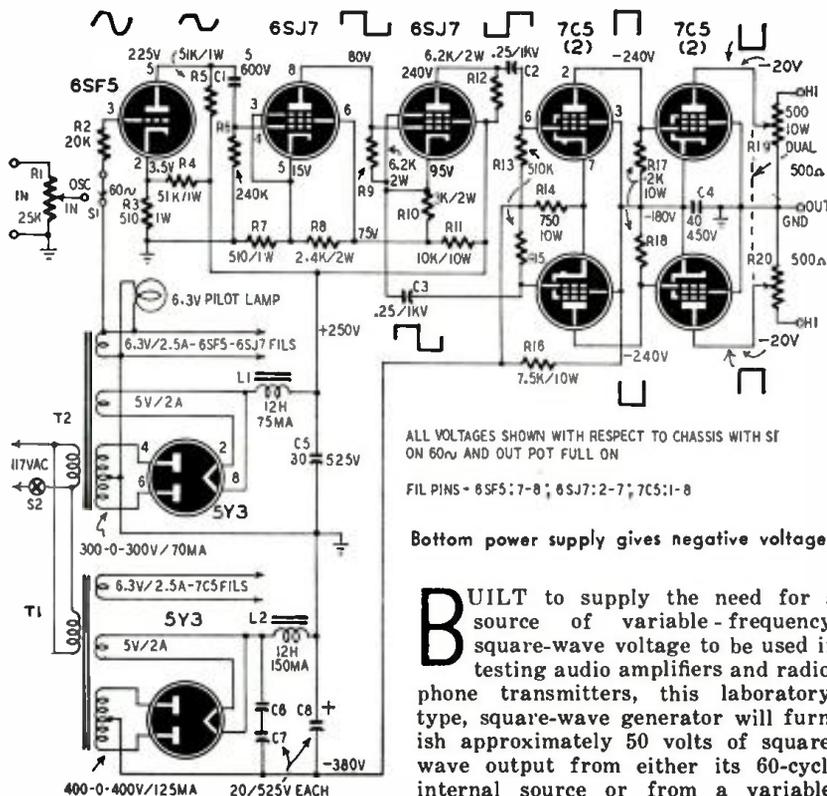
be coupled to the IN terminals to produce square waves as high as 50 kc. The voltage available from the OUT terminals may be varied by the OUT potentiometer when using 60-cycle input or from the IN or OUT potentiometers, or both, when using an external audio oscillator as the signal source.
