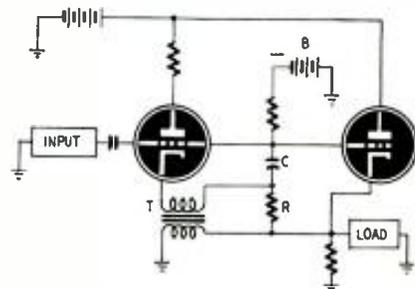
voltage drop is transmitted through C to both control grids. This voltage being positive, both tubes are saturated. When this condition is reached, capacitor C begins to charge; a negative charge collects on the grid and both tubes are quickly blocked, ending the cycle until the next signal arrives.
