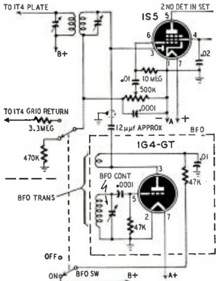
increase the tuning range to 36 mc if you desire 10-meter reception. A two-gang, 35- $\mu$ f capacitor can be connected across the main tuning capacitor to provide bandspread tuning.
