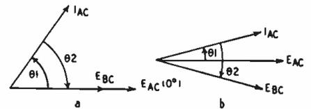
Fig. 2—Vectors show how the null is reached.
