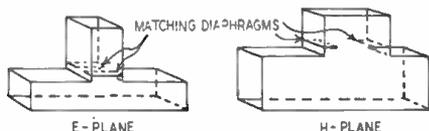
Fig. 3—Windows used in waveguide branch.
