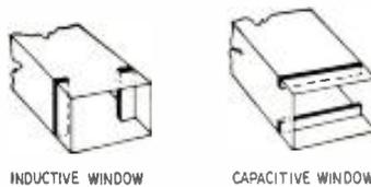
Fig. 2—The inductive and capacitive windows.
