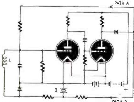
feedback voltage to the cathode. Therefore, at the crystal frequency, there is no negative feedback and the circuit oscillates only at this frequency.
