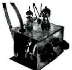
**NEW 13 CHANNEL TUNER** is a small compact unit with stage of R.F. Tunes all TV and ZFM channels. Made to conform with Telekit or any other TV set having video I.F. of 25.75 Mc. Complete with tubes, pre-wired, pre-aligned; only three connections to make. See your jobber, or write to us for information. Your cost, \$19.95.
