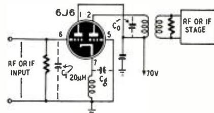
put transformer, tuned by Co to the center of the passband, is shunted by a resistor to lower its Q for wider band response.
