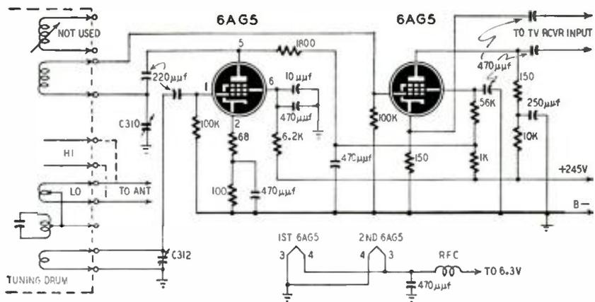
Fig. 2—Circuit of booster. Oscillator-a.f.c. tube was removed and mixer made output stage.
