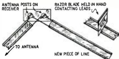
Fig. 3—Add piece of line and test with blade.
