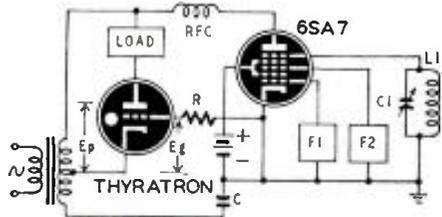
The current which flows in the plate circuit of a thyratron is greatest when the plate voltage  $E_p$  is in phase with the grid voltage  $E_g$ . It is zero when these voltages are out of phase.
