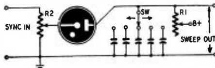
Fig. 3—R2 controls amplitude of sync signal.
