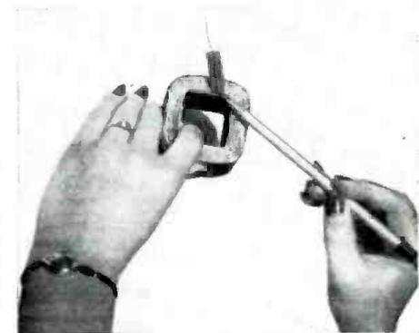
Finished job, showing method of attaching lead wires. These connections are usually
