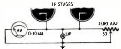
for zero adjustment. The switch bypasses the meter and reconnects the cathodes directly to ground when no meter indication is desired.
