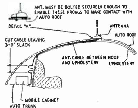
Fig. 1—How antenna is installed in car roof.
