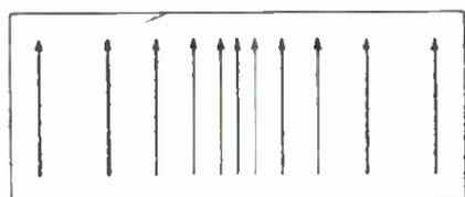
Fig. 5—Cross-section of guide, TE<sub>10</sub> mode.
