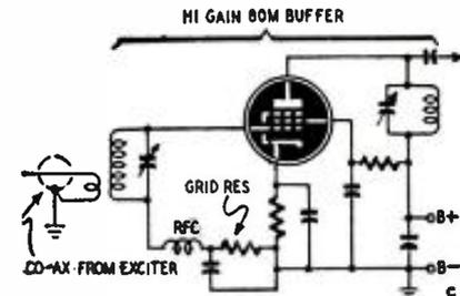
Fig. 3-c—The exciter works into a buffer.
