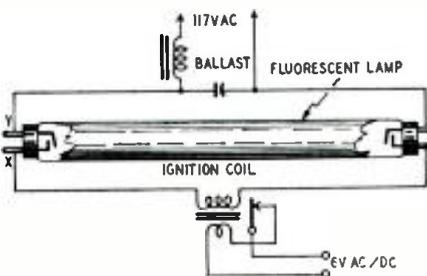
high-voltage a.c. This ionizes the gas sufficiently to allow the 117-volt line current to keep the tube lit. After the lamp is started, the coil can be removed.
