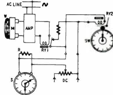
watch then stops and indicates the speed of the test watch. If W runs correctly, this happens exactly 30 seconds later. If it is too slow, it occurs later, and if too fast, the beats coincide earlier. The stop watch indicator travels around once every 30 seconds, and its face is calibrated in seconds per day to show the speed of the watch, W.
