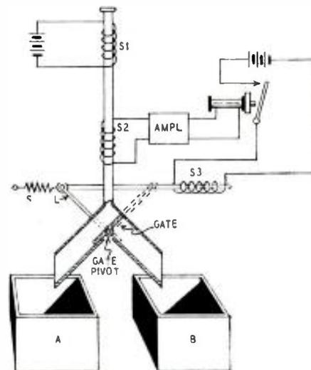
The pivoted gate is fixed to a lever L at right angles to it. Normally L is forced to the left by a spring S. This position is shown by full lines in the drawing. When L is forced towards the solenoid S3, the lever and gate take the position shown by dotted lines. Note that in the
