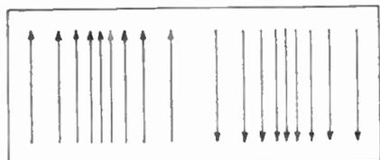
Fig. 6—An electric field of the TE<sub>20</sub> mode.
