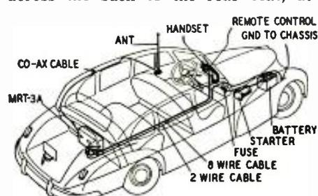
Fig. 2—Installation of components and leads.
