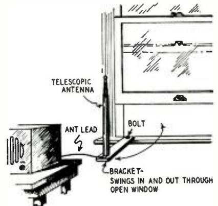
The antenna is a 10-foot collapsible rod type, obtained from surplus. It is mounted on a strip of wood. The other end of the strip is bolted to the window sill.
