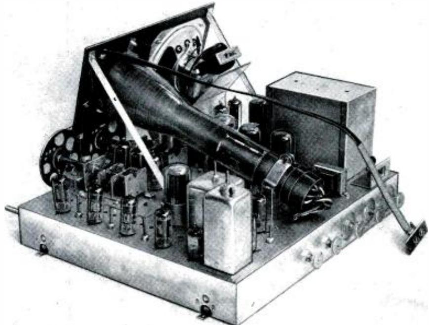
Fig. 1—This set employs separate tuning condensers for high- and low-band TV channels.
