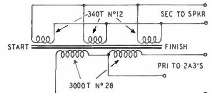
Schematic and specifications of the windings.
