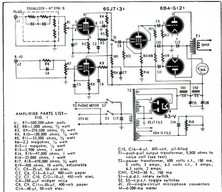
ter condensers—that were selected for the power supply were on the hefty side, allowing a generous margin for safety and making for trouble-free operation. R19, the 6B4-G biasing resistor, should be adjusted to give a 45-volt drop across it.
