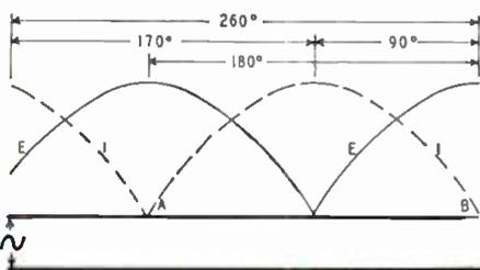
Fig. 2—Voltage and current on an open line.
