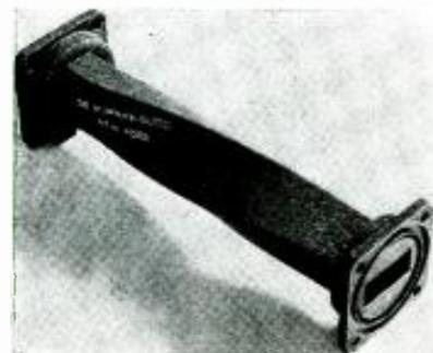
Fig. 16—This section changes polarization. precision-cut so as to absorb any leakage power and cause a minimum of reflection at the junction.
