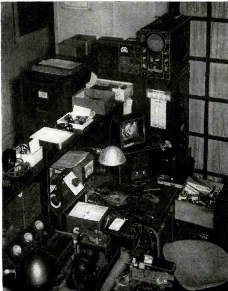
Intercoms, hearing aids, and amplifiers are tested and repaired on Audiphone's bench.
