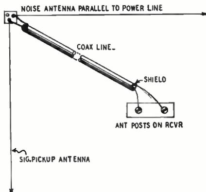
siderably by using the out-of-phase bucking principle.
