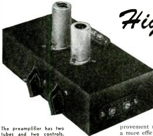
The preamplifier has two tubes and two controls.
