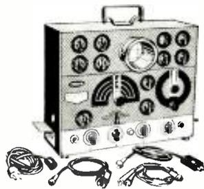
Output is controlled by a shielded attenuator. To compensate for the loss in gain usually present at the higher frequencies, output of all generators increases about five times at the high frequencies over that at the low end of
