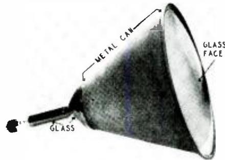
is used for the face. Advantages include: lighter weight (the new tube weighs only about one-sixth as much as a 15-inch all-glass tube); larger viewing area (144 square inches, compared with 115 for a standard 15-inch glass tube); and better shielding from ambient light.
