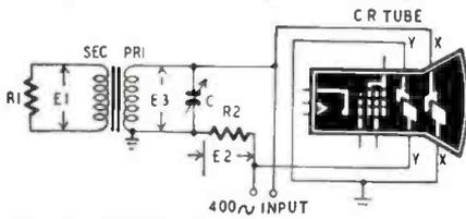
veloped across it when power is applied to the primary. The power in watts is equal to the square of the voltage divided by the resistance. Measuring power input is not as simple because leakage inductance of the transformer causes the input voltage and current to be out of phase, thus producing false readings. If a capacitor of proper value is shunted across the primary, the leakage inductance will be balanced out and current and voltage will be in phase.
