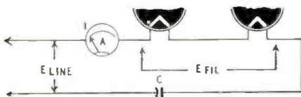
itor for a device using two tubes, each with a 12.6-volt filament drawing 0.15 amp, with a 120-volt line,
