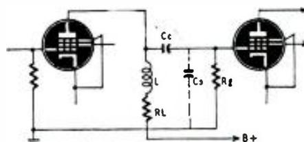
Fig. 1— $L$  and  $C_s$  are parallel tuned circuit.
