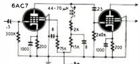
Fig. 4—Peaker gives flat response to 2.5 mc.
