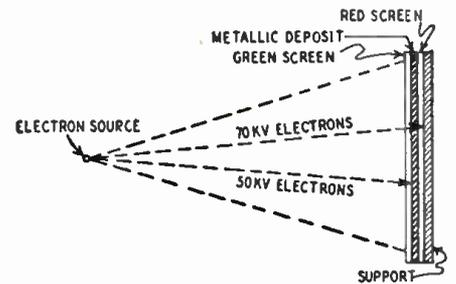
In the presence of 50 kv electrons the green screen becomes dark after developing. If the entire plate is then held to a light these areas will look red. When the plate is exposed to 70 kv electrons, the red screen becomes dark. Therefore the plate looks green when held to a light. Different color shadings correspond to slightly different electron velocities.
