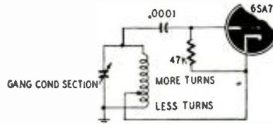
Fig. 3—Grid-cathode winding is the largest.
