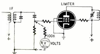
Fig. 1—Meter placement for aligning i.f.'s. a band width of 200 kc. Two basic methods are used to obtain wide-band response: overcoupled transformers and single-peak transformers.
