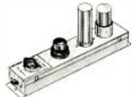
of clipping can be accomplished. A low-pass filter attenuates the harmonics created by the clipping action. A 6SC7 and a 6H6 are used. B-plus (150 volts at 5 ma) and 6.3 volts at 0.6 amp for the filaments must be furnished from an external supply.
