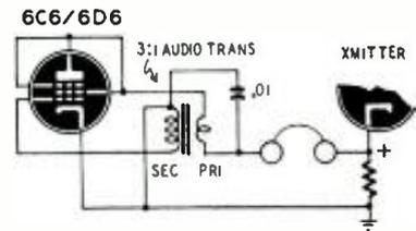
of the resistor should be chosen to give about 6 volts, though a somewhat higher voltage will be as satisfactory. The transformer is any 3:1 audio unit.
