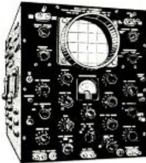
Other features include a vertical amplifier band width of 6 mc, recurrent sweeps of from 5 to 500,000 per second, and driven sweep rates of 0.25 microsecond per inch to 200 microseconds per inch. An internal trigger generator is also provided, as well as a variable delay circuit which may be used to provide delayed triggers or a delayed sweep either internally or externally triggered. A calibration device provides measurement of deflection sensitivity through the amplifier.
