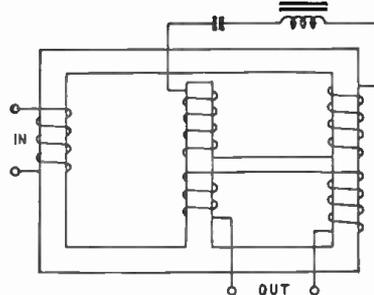
The output voltage is due mainly to the winding around the right-hand leg. This is opposed and stabilized by the voltage induced in the center leg winding which is more sensitive to load changes. A third winding is connected to a series condenser and iron-core inductance which resonate at the third harmonic of the line frequency. The harmonic is greatly reduced, leaving a pure output wave.
