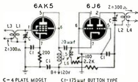
Fig. 1—Unit is a cascode with double tuning.
