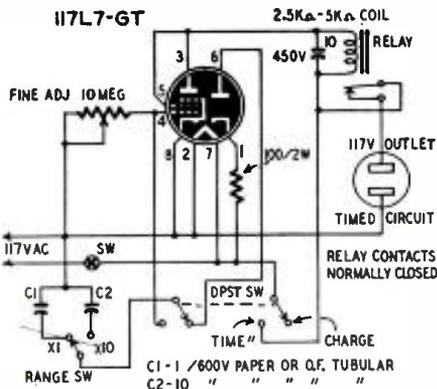
components. The maximum time can be increased somewhat by adding a third position to the range switch, with a 20- to 40-uf paper capacitor.
