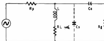
Fig. 2—Equivalent circuit of that in Fig. 1.
