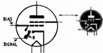
plate current from flowing until the filament is fully heated. To do this the inventor has included a thermal delay relay in the grid circuit of an otherwise normal tube.
