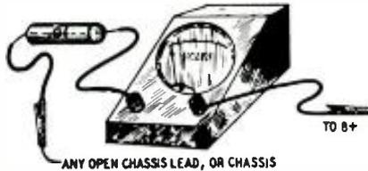
the voltage does not exceed the condenser's rating. (Caution: make sure the B-plus voltage falls within the voltmeter range.)
