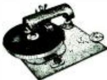
The mechanism is enclosed to prevent dust and record chip from fouling the gears. An automatic safety feature raises the cutter when it reaches the inside of the disc, preventing damage to record and stylus. The mechanism, available separately, is adjustable to fit almost any 12-inch turntable.
