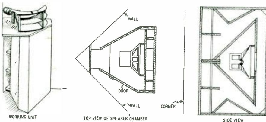
Construction of Klipsch speaker. Low-frequency sound comes from the vertical side slots.
