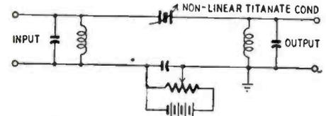
there is negligible power loss. Its nonlinear transmission produces harmonics.
