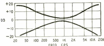
Graph shows maximum possible tone variations. the equalizer response is flat when control shafts are at mid-points in their arcs. At these settings, the insertion loss of each channel is 20 db. The losses are compensated by 20-db triode amplifiers following each network.
