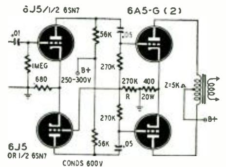
Fig. 2—R should be large for best balancing.
