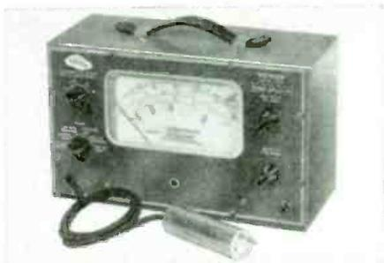
**MODEL 900-A "VOMAX".** The new "VOMAX" is the truly universal v.t.v.m. — makes TV, FM and AM measurements accurately — at highest meter resistance. Giant meter, non-breakable glass; 45 ranges; new single probe for a.c., d.c., a.f., r.f., volts, ohms, db. and current measurements. Advancing far beyond its predecessor, the overwhelming choice of experts, "VOMAX" equips you with the world's newest and finest meter for only \$68.50 net.
