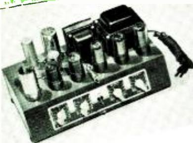
Below is the Ward voltage amplifier. One or two of the power amplifiers may be added.
