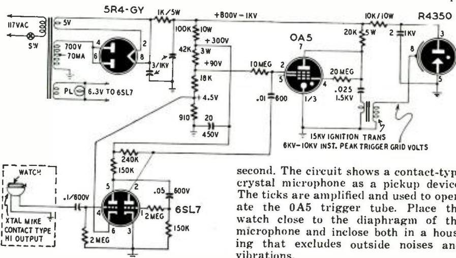
second. The circuit shows a contact-type crystal microphone as a pickup device. The ticks are amplified and used to operate the OA5 trigger tube. Place the watch close to the diaphragm of the microphone and enclose both in a housing that excludes outside noises and vibrations.
