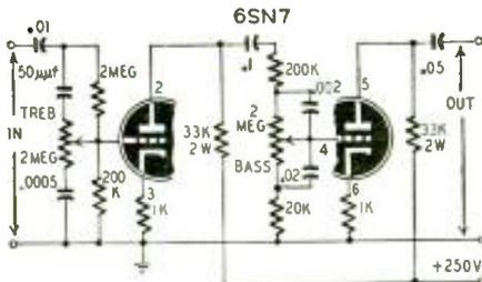
The equalizer controls both treble and bass. sufficient reserve voltage gain.
