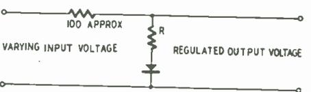
Fig. 10—Voltage regulator circuit. Germanium crystal is used. R is the limiting resistance.
