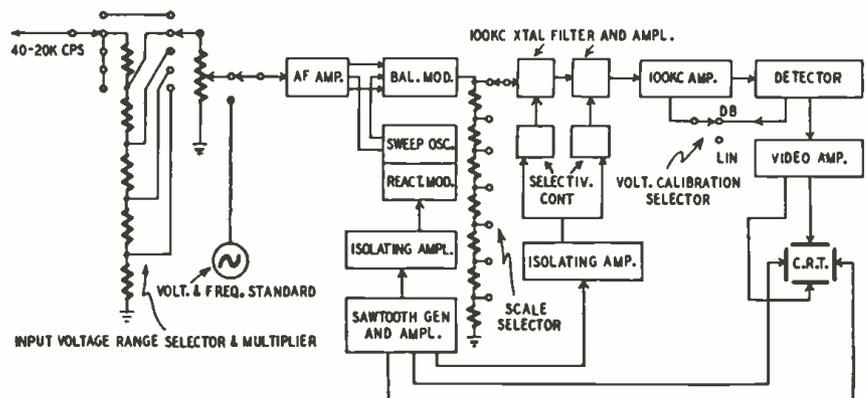
Fig. 2—Block diagram of the Panoramatic Sonic Analyzer's main chassis (upper section in photo).
