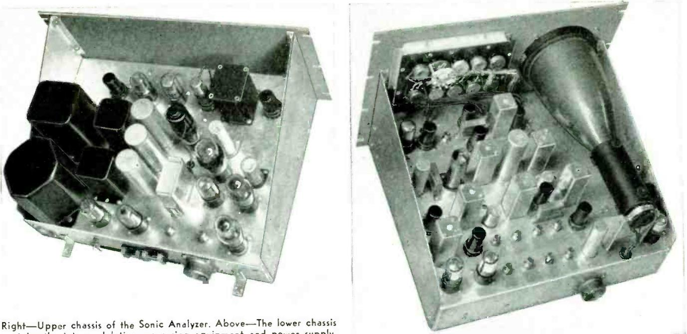
Right—Upper chassis of the Sonic Analyzer. Above—The lower chassis contains the intermodulation measuring equipment and power supply.
