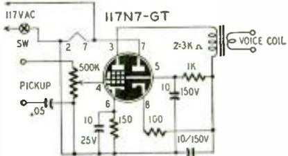
is used. No tone control was found necessary, but if one is desired, a capacitor and 1-megohm variable resistor may be placed in series between the amplifier grid and common negative.
