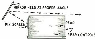
picture tube. This not only speeds up the installation process but also makes for more accurate adjustments than the usual method of going around to the front of the set after each trial setting of the controls.
