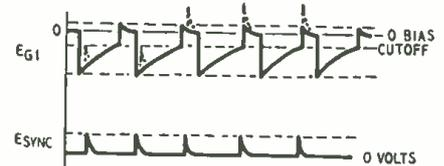
Fig. 3—Effect of superimposed sync signal.
