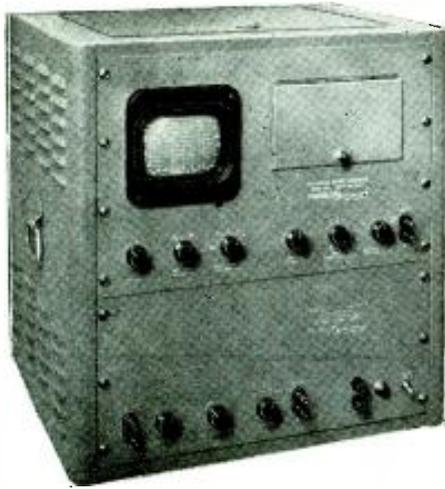
**P**ANORAMIC analysis of radio-frequency signals became familiar during the last war. A receiver was electronically or mechanically tuned continuously over a given band of frequencies and its output fed into the vertical amplifier of a cathode-ray oscilloscope. A signal on any part of the band being covered would cause a pip to appear on the oscilloscope trace. By synchronizing the horizontal sweep of the oscilloscope with the tuning apparatus,
