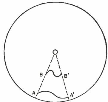
Fig. 3—Pinch Effect cause near disc center.
