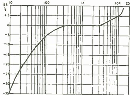
Fig. 2—British discs are recorded this way.
