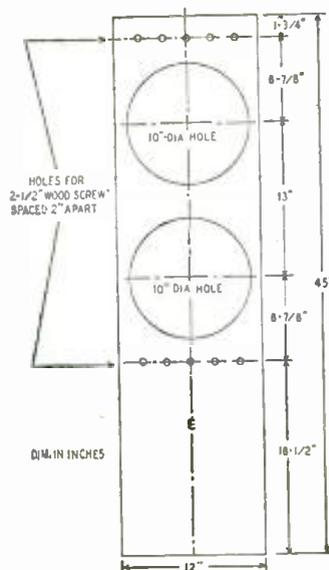
Fig. 3—Detail of one of the speaker boards.
