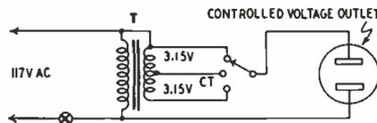
Connect a 6.3-volt filament transformer as shown in the diagram. The secondary should be rated at 1.2 amperes or higher and should be center-tapped. Rotating the selector switch will give three different voltages, the line voltage and two higher values. If the other values are lower than the line voltage reverse the connections to the secondary.
