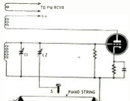
Fig. 2—One method of using FM for piano.
