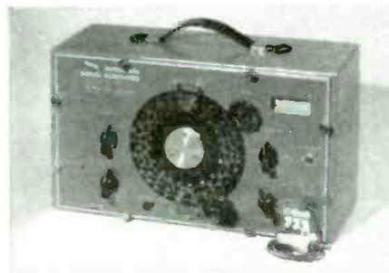
**MODEL 906 FM-AM SIGNAL GENERATOR.** Similarly the choice of the big engineering laboratories plus thousands of service technicians, 906 stands out as maximum value. 90 kc. thru 210 mc. in 8 ranges,  $\pm 1\%$  accuracy; less than ½ microvolt, including strays to over 1 volt v.t.v.m.-metered output; multiple shielding; adjustable 0 to 100% amplitude modulation; adjustable 0 to 1,000 kc. FM sweep. Net price only \$116.50.
