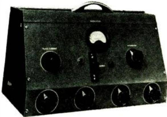
A preamplifier-mixer permits the recordist, PA operator, or remote-broadcasting engineer to control and monitor programs
