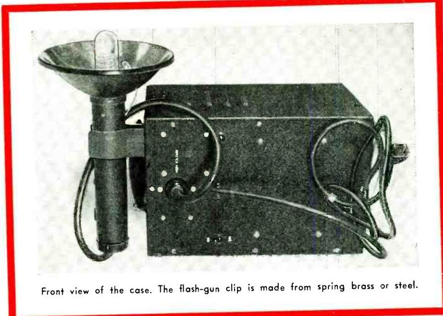
Front view of the case. The flash-gun clip is made from spring brass or steel.
