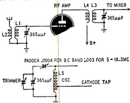
For the 5.8-18.3-mc. band, L1 is 9 turns of No. 18 enameled or s.c.e., 1 inch long. L2 and L3 are 3 to 4 turns of No. 18, close-wound, with L2 spaced about 1/8 inch from L1. L4 is about 4 turns of No. 18 wire, close-wound, about 1/8 inch from L3. L5 is 10 turns of No. 18 enameled or s.c.e., 1 inch long. The tap is about 4 turns from the ground end.
