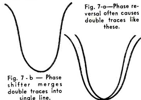
Fig. 7-b — Phase shifter merges double traces into single line.
