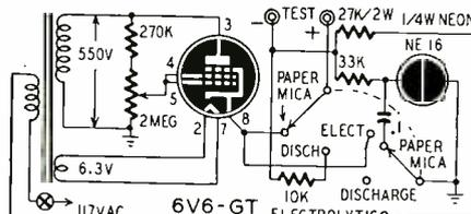
Fig. 1—Dual tester is relaxation oscillator.
