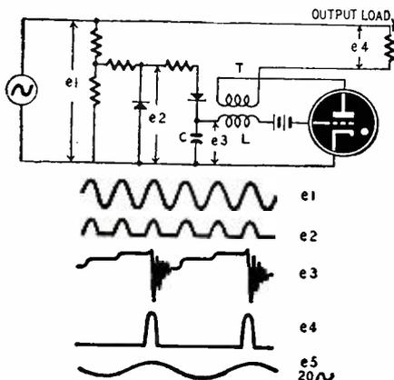
The sine-wave, 60-cycle supply is shown as e1. After the first rectifier it becomes e2, across the second rectifier and condenser C. Current can flow through the second rectifier to charge the condenser. The charge takes place in steps as each half-wave adds its current. At some critical value, the voltage across C is sufficient to overcome the negative bias on the gas-filled tube. It then breaks down and current flows in the
