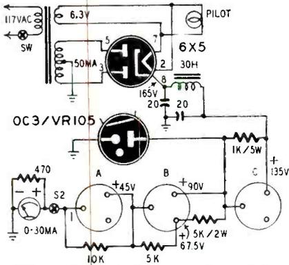
The outlet sockets were salvaged from old B-batteries. Sockets from portable batteries often have holes for different types of battery plugs. When plugging in a set, be sure that the battery plug with the negative lead goes into socket A. If the set uses 135 volts, the plug with the negative lead goes in A, the one with the positive lead in C, and the plug connected to the others with jumpers goes in B.
