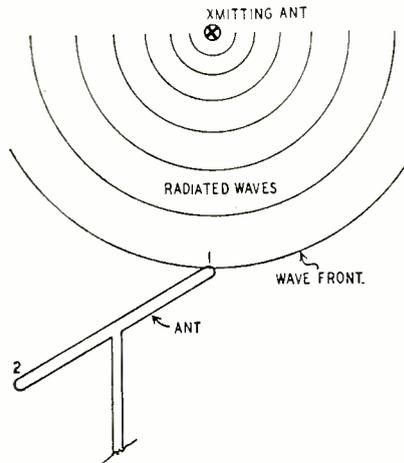
Fig. 2—Dipole is not parallel to wave front.
