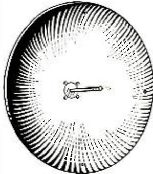
920-960-mc band. They are available in three sizes, 2, 4, and 6 feet in diameter, with gains of 10, 15, and 20 db over a half-wave dipole. The antennas are to be used in pairs—one at the transmitter and one at the receiver—to provide gains of 20, 30, and 40 db over a line-of-sight path. Transmission line should be 52-ohm co-axial cable. The parabolas are made of aluminum.
