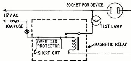
not go on at all, the thermostat switch (or the device itself) is inoperative. Do not test a device that draws more than 1,200 watts.
