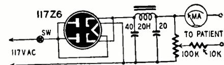
Fig. 6—Simple instrument for iontophoresis.
