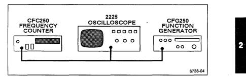
Figure 2-3. Output Test Configuration.
