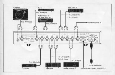
Establish connections to other system components as shown in the above example. While making connections, be sure to set the power switches of all components to "OFF"
