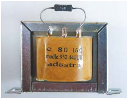
Fig.14. When measuring the impedance of transformers it is essential they are loaded with the correct load resistance
