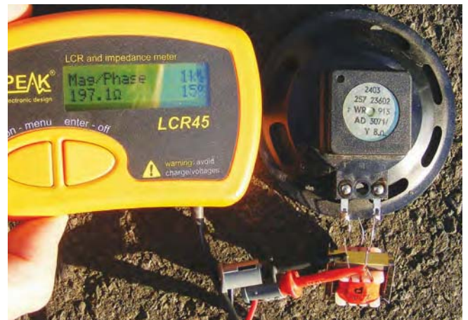
Fig.13. Measuring the impedance of an 8Ω speaker reflected through the Xicon output transformer. Your delicate germanium transistors will be safe
