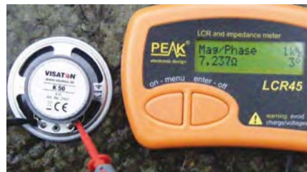
Fig.3. Using the LCR45 to measure the impedance of a loudspeaker. Note it is slightly below the specified 8Ω. This is a standard trick to boost the apparent sensitivity at the expense of increased current draw
