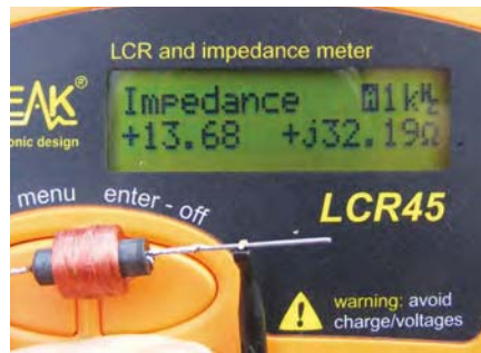
Fig.6. With each push of the 'enter' button, the unit goes onto the next measurement. Complex impedance is now displayed
