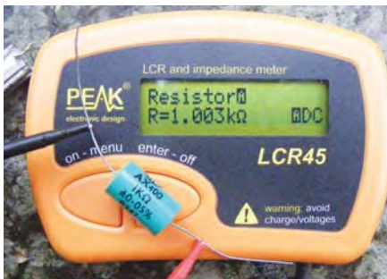
Fig.2. A simple task – measuring a 0.05% tolerance precision resistor
