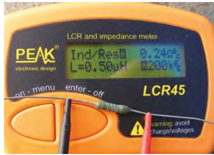
Fig.10. 0.22Ω wire-wound resistor with unusually high parasitic inductance. These resistors caused problems when used as source/emitter resistors in audio power amplifiers
