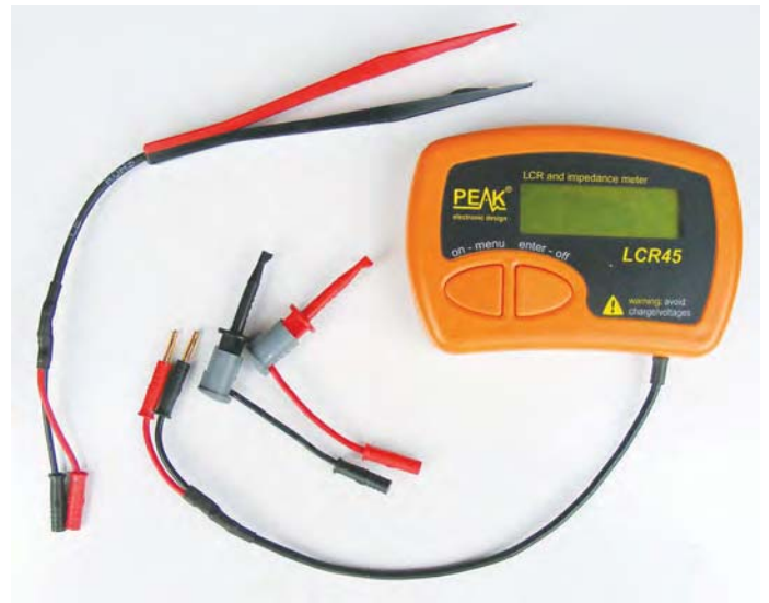
Fig.1. The LCR45 impedance analyser and LCR meter. The attachable surface-mount tweezers are an optional extra
