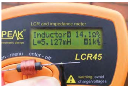
Fig.5a (top). Connecting a small radio frequency choke to the LCR45. Just before turn-on. Fig.5b. (bottom) Stepping through the measurement sequence on automatic with a small inductor. This shows the inductance, the DC resistance and the frequency at which the measurement was made
