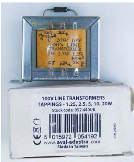
Fig.15. This Adastra 20W 100V line transformer is ideal for small valve amplifiers. It gives an 8kΩ anode-to-anode load with a centre tap. Stock code 952.440UK. Order code from CPC is DP33221, £7.50 plus VAT
