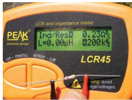
Fig.12. A fusible metal-film resistor exhibits negligible inductance
