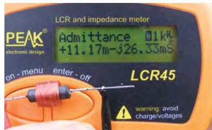
Fig.7. Admittance – reciprocal of impedance
