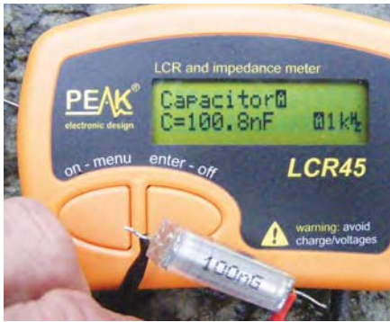
Fig.9. Measuring a 2% tolerance 100nF polystyrene capacitor
