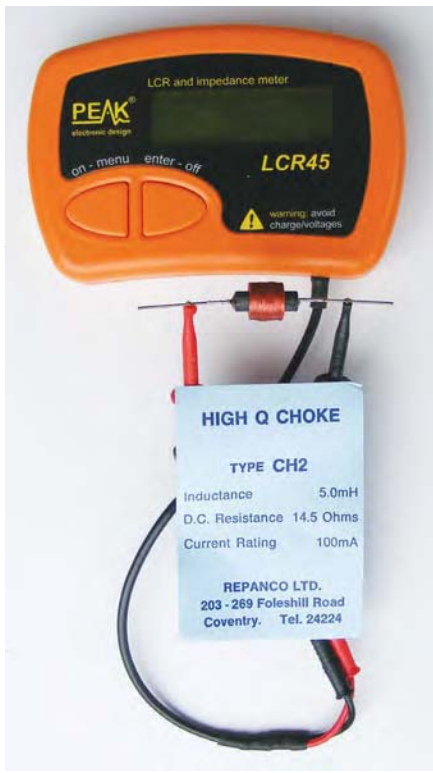
Fig.6. With each push of the 'enter' button, the unit goes onto the next measurement. Complex impedance is now displayed
