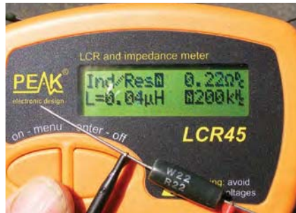
Fig.11. 'Normal' wire-wound resistor inductance
