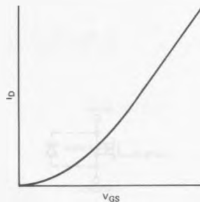
Transfer Characteristics of VMOS Showing Linear I_D/V_{GS} Relationship Figure 3
