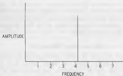
FIG. 1—A representation of a single radio frequency, shown by plotting amplitude against frequency. A steady signal by itself takes up no room in the spectrum.
