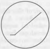
FIG. 16—Effect of inadequate response of vertical amplifier.
