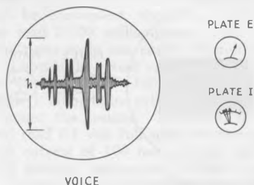
FIG. 2—Voice-modulated s.s.b. signals look something like this on a scope. Here the height h represents the maximum amplitude that the amplifier can handle without distortion. Since the signal hits these high peaks only occasionally, the indicated power input will be low. The syllabic nature of the signal is indicated by the jumpy plate milliammeter.
