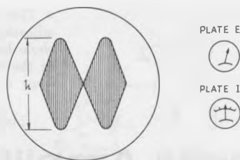
FIG. 3—The two-tone test signal applied to the linear of Fig. 2. The maximum permissible amplitude h is the same, but now the indicated power input bears a definite relationship to the peak envelope input.
