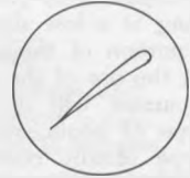
FIG. 17—Double trace caused by audio phase shift.
