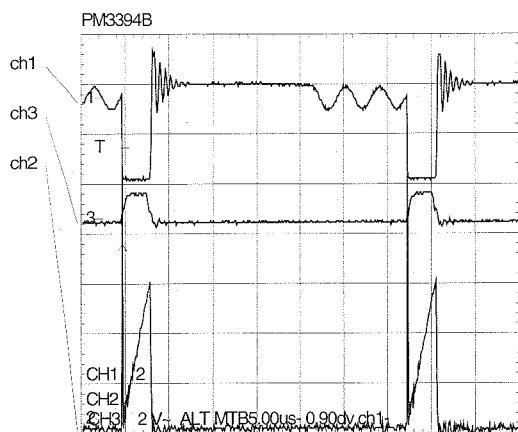
ch1 : Drain voltage at testpoint T632 ch2 : Drain current ch3 : Gate voltage at testpoint T669
