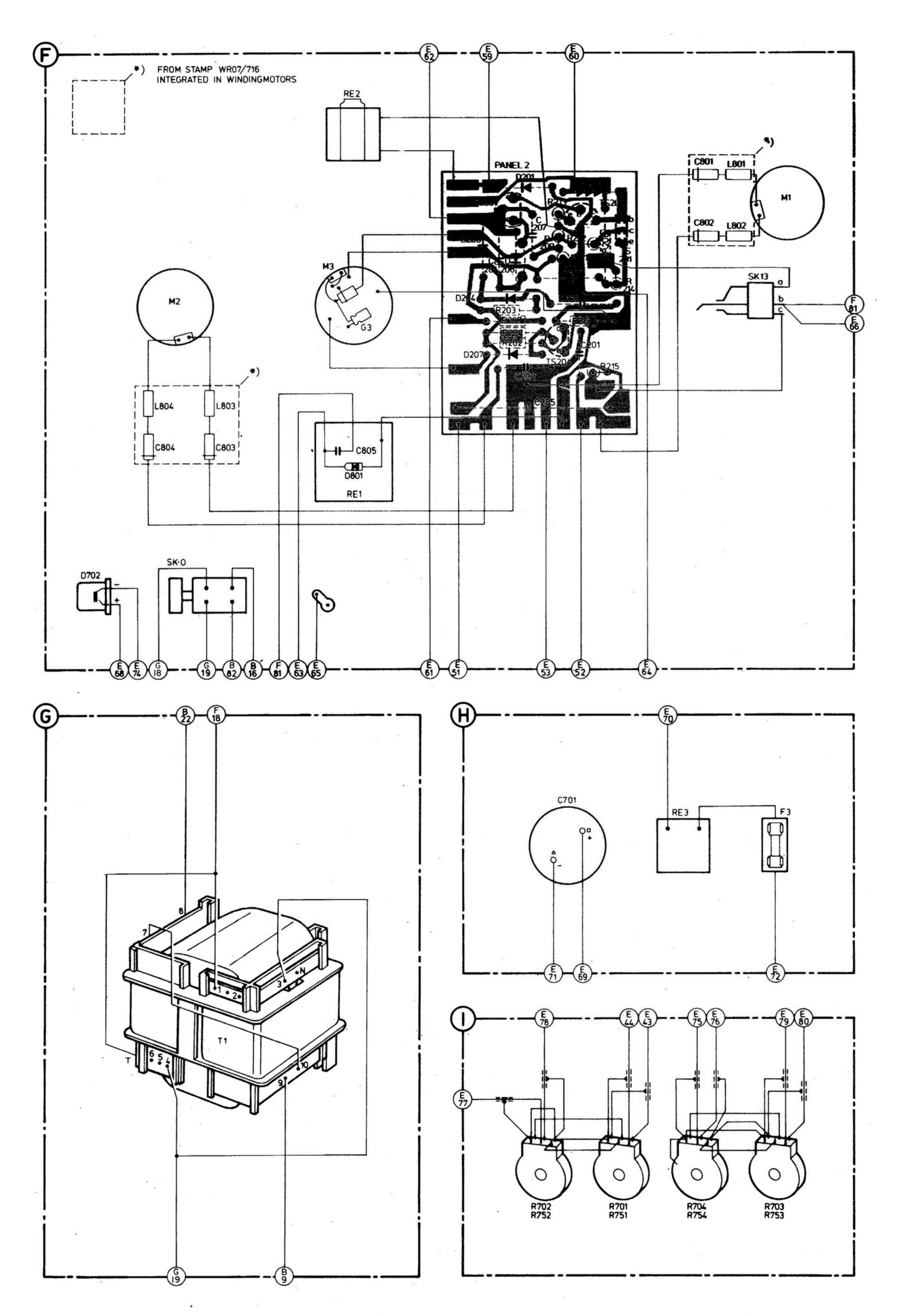
Figure 24 N4504 WIRING DIAGRAM (BOTTOM VIEW OF TACHO BOARD)
