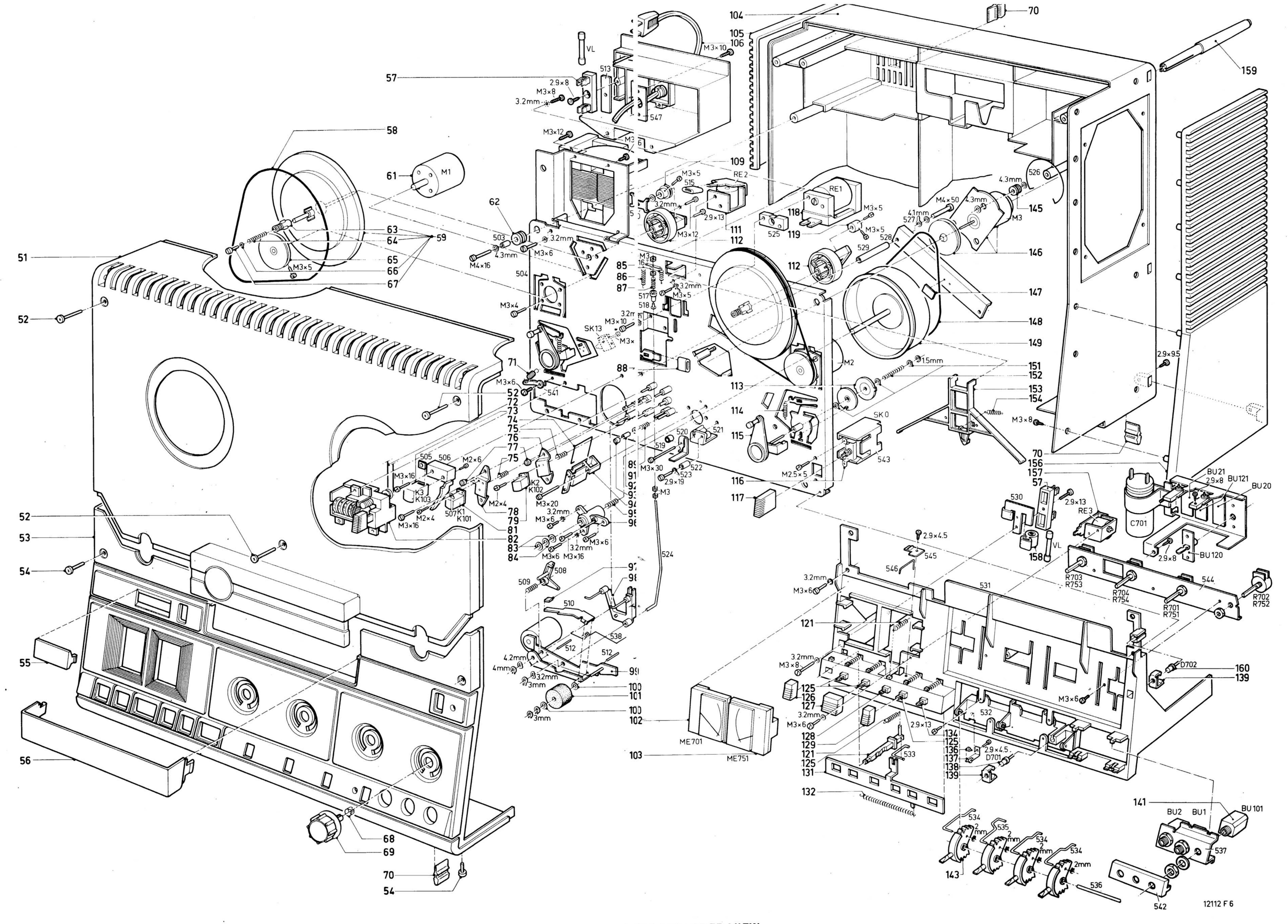
Figure 19 N4504 EXPLODED VIEW
