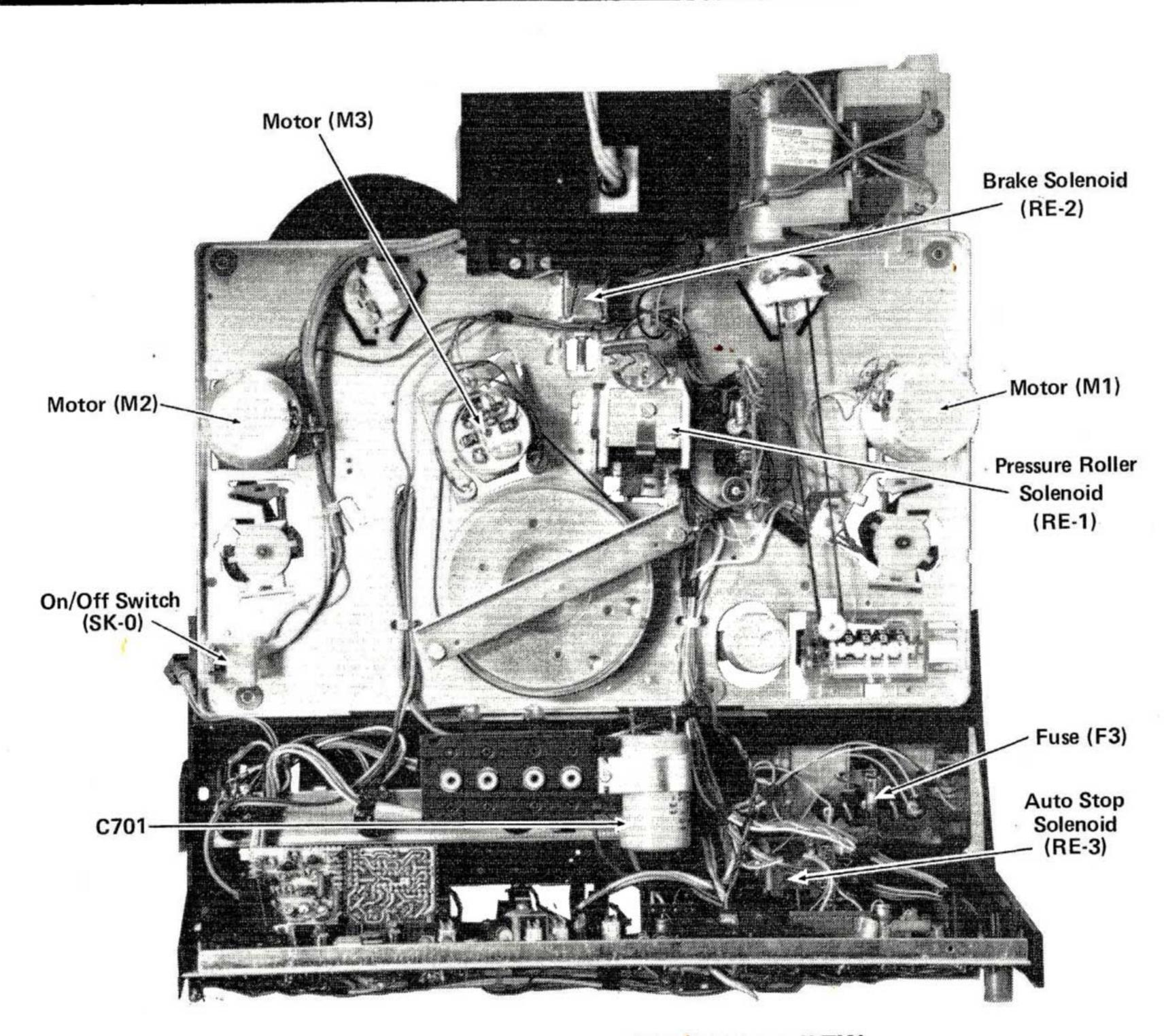
Figure 5 N4504 CHASSIS REAR VIEW
