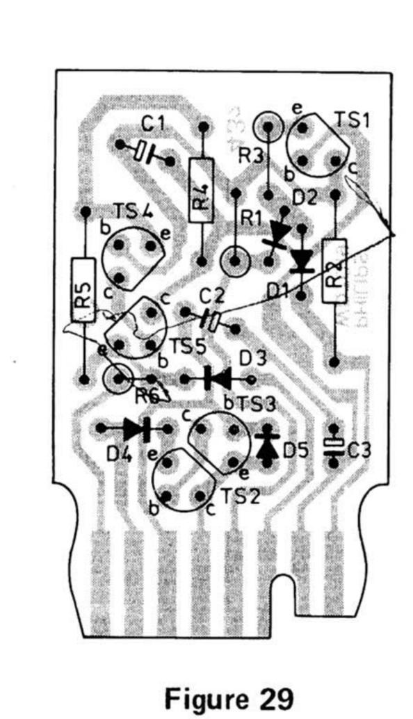
TAPE TENSION BOARD (TOP VIEW)
