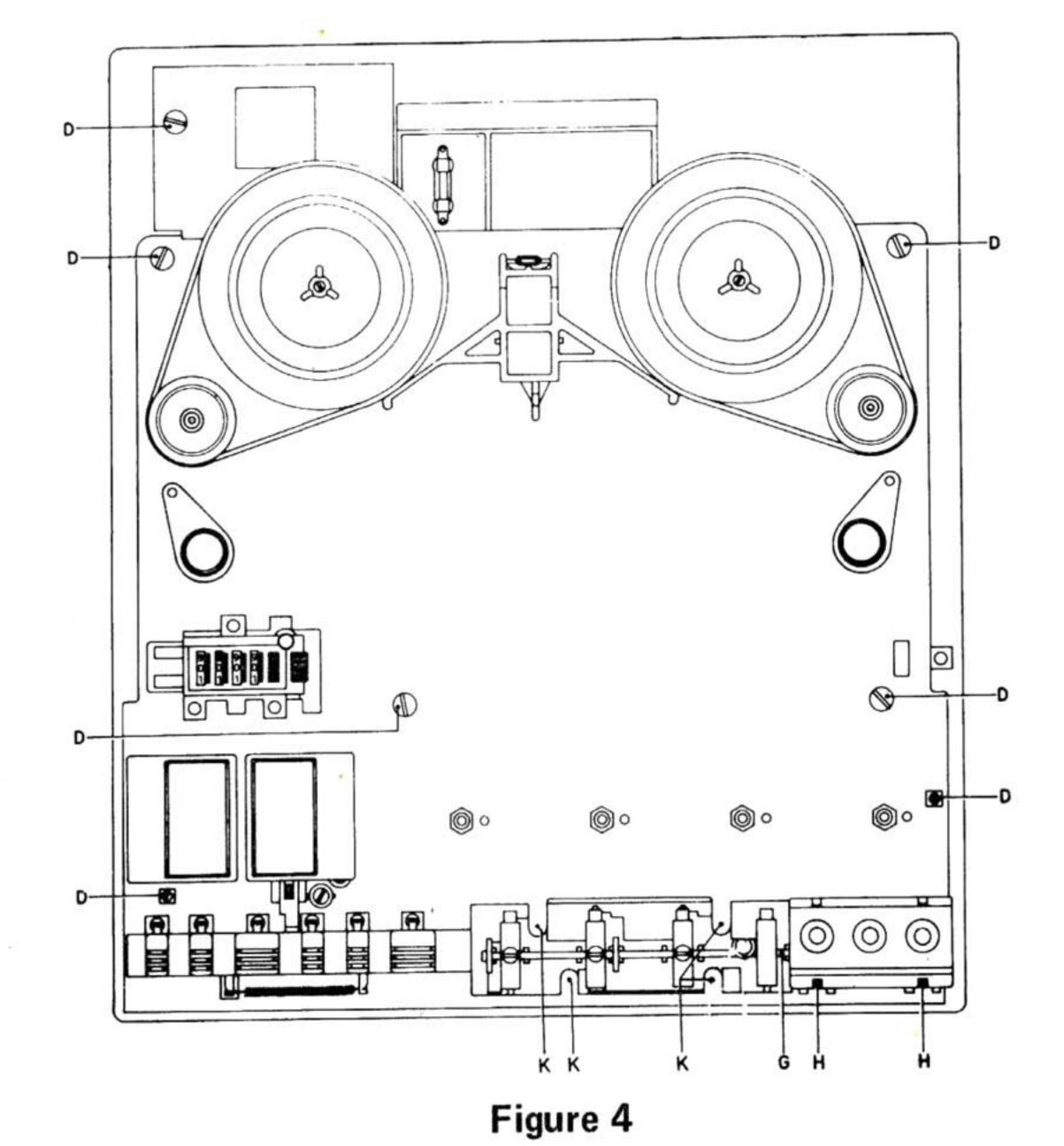
3. Pull shaft (G) to the right far enough to allow the removal of the defective switch lever. (Note: for removal of levers 22 and 24 the chassis must be removed from the cabinet back.
