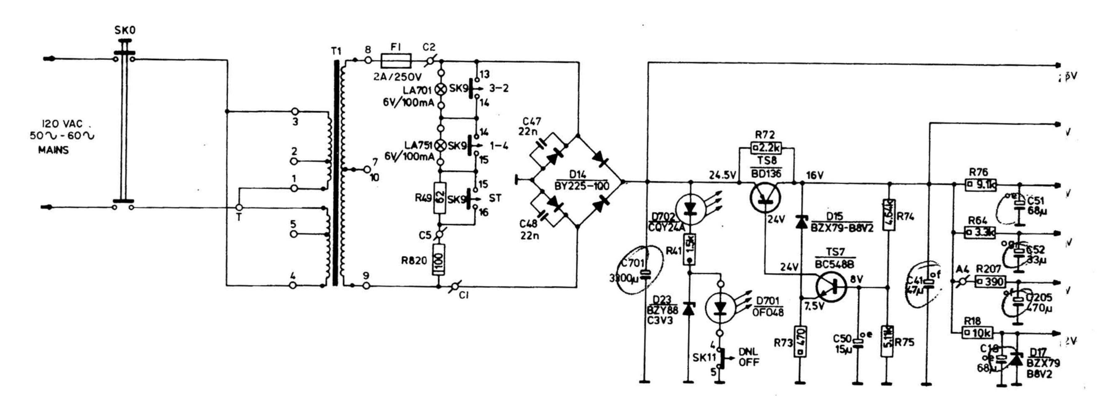
Figure 22 N4504 POWER SUPPLY SCHEMATIC DIAGRAM
