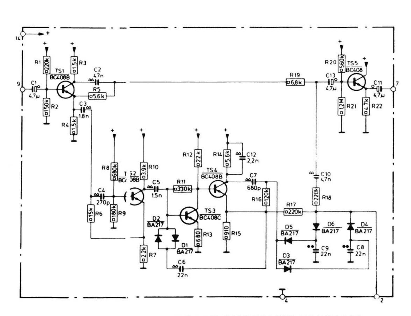
FIGURE 31 DNL BOARD SCHEMATIC DIAGRAM
