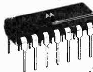
From Motorola, a monolithic dual stereo preamplifier
