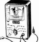
Made by Mallory but suitable for all batteries made by Ever Ready and others, most of which are zinc carbon types but also mercury manganese—nickel—silver oxide and alkaline batteries may be tested. The tester puts a dummy load on the battery and the meter scale indicates the condition depending upon which section the pointer rests. The section reads "replace", "weak" or "good". The tester is complete in its case, size 3 1/2" x 6 1/2" x 2" with leads and prods. Price £2-25 plus 20p postage.
