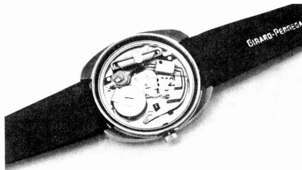
the mechanical vibrator 170 times per second. This correction is carried out by a relatively simple circuit employing only 14 transistors, 19 resistors and seven capacitors. The logical deductions made by this circuit are fed to the motor as correction signals. This watch is said to be the first cybernetic watch, since it employs a comparison circuit or "brain".
