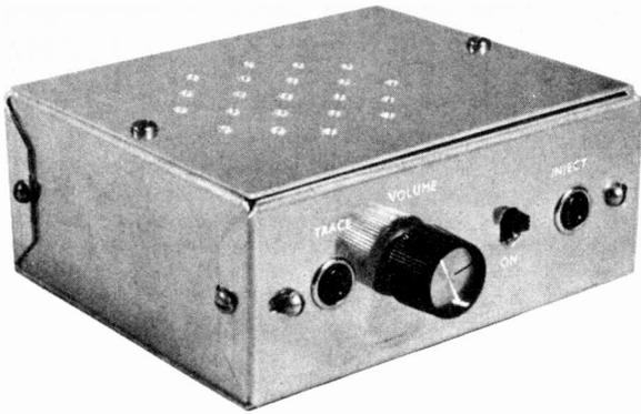
Photograph of the completed signal injector and tracer unit showing the layout of the front panel. The box is built using universal chassis members
