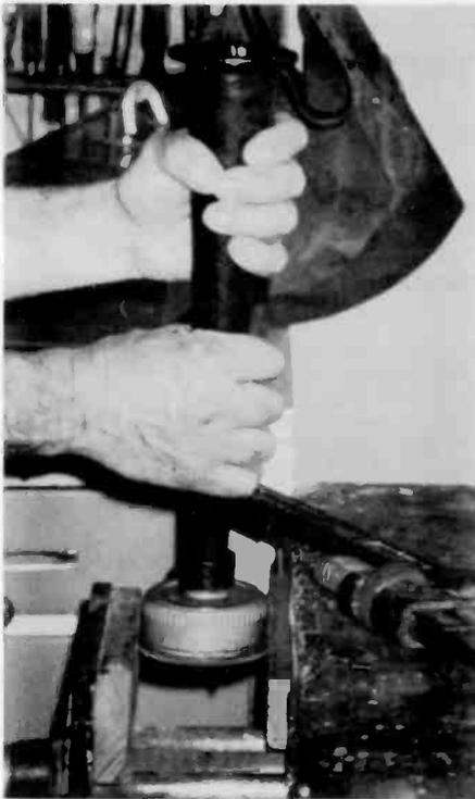
Figure 3. The milled edge of the driver base held in soft wood, but nothing budges.
