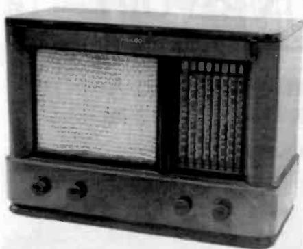
**PHILCO TROPIC, MODEL 42-761** – This set appears to be from the same family of radios made for New Zealand distribution. It has permeability tuning and 8 separate broadcast bands. Found in an old storage trailer in a salvage yard, it is in remarkably good condition. (Barry Siembar – Woodinville, WA)
