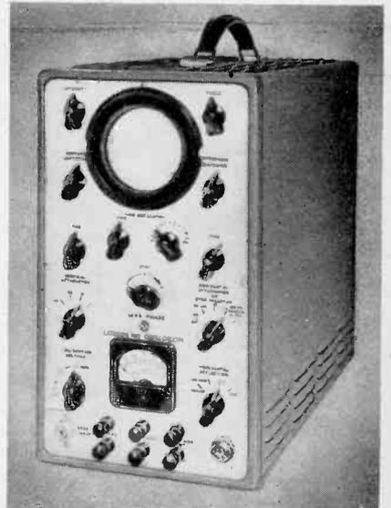
vision signal expansion for checking square-wave time, and for checking irregularly timed pulses. The intensifying amplifier increases the brilliancy of the waveform after the time-base generator is triggered, permitting examination and photography of small, otherwise, faint, and extremely short pulses. Signal-triggered deflection, line frequency deflection, and blanking are some of the other unusual features of this new RCA oscilloscope.
