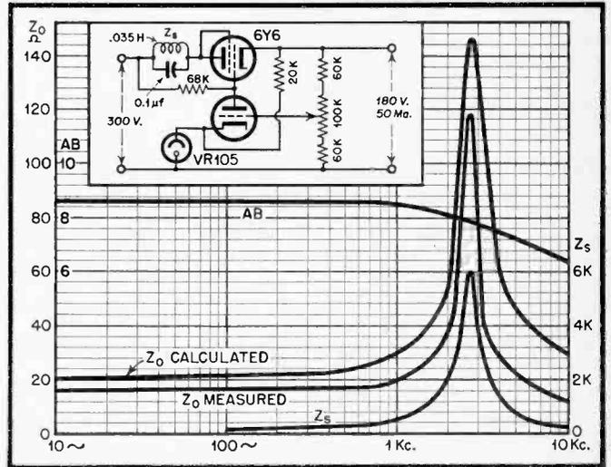
the power supply oscillate, it is recommended that a sufficiently large value of C<sub>o</sub> be used that any capacity in the load will not result in a total capacity which will produce the conditions required for oscillation. Experiments indicate that approximately 2.0 μf is about the minimum value that will effect a reasonably sure cure for this trouble. This has the added advantage of maintaining a low output impedance at high frequencies.
