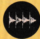
SSB signal voice input correctly adjusted.
