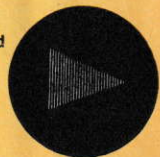
RF trapezoid Good linearity. Desirable pattern.
