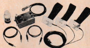
Bioelectric. IMPSCOPE shows bioelectric phenomena in plants (175 mv action potential of Nitella internode).
