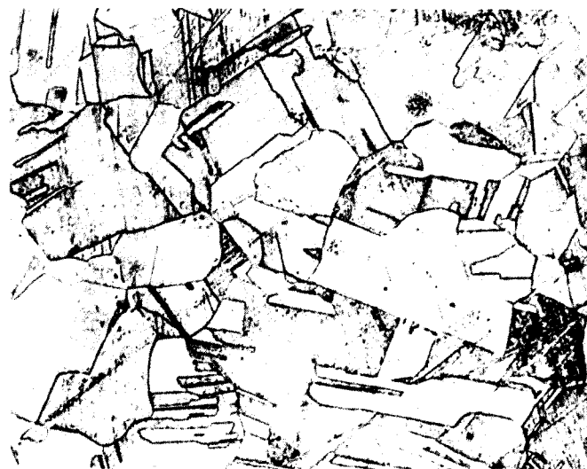
Figure 2. Grain Structure of Nickel (200 X)
