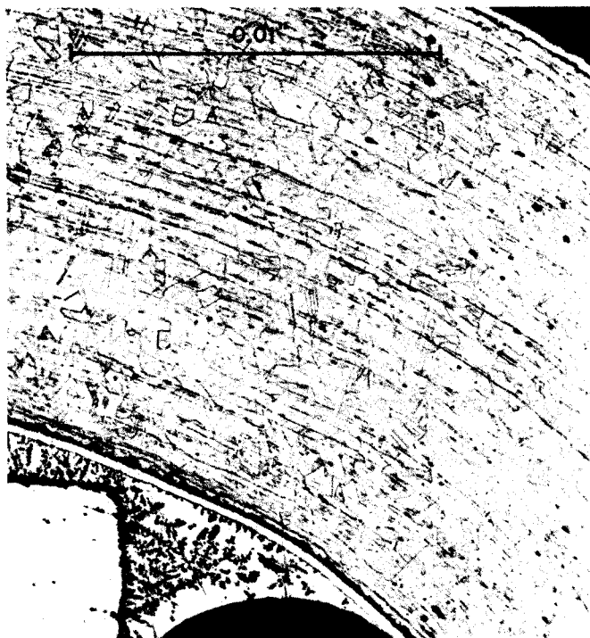
Figure 5. Cobalt-Nickel-Iron Alloy (structure similar to that of Figure 4) Protected by Nickel Plating
