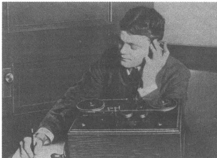
Fig. 5.22 A Marconi hysteresis detector in use [Collins, A.F. 'Manual of Wireless telegraphy', (Wiley/Chapman & Hall, 1906) p.165]
