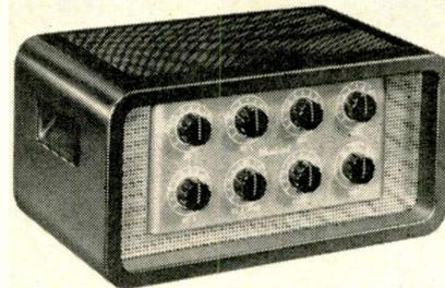
Output of the preamp, measured at 100, 400, and 5000 cycles, is 300 mw, two percent at 600 ohms. Microphone gain is 109 Db on high impedance and 96 Db on low. Phonograph channel gain is 73 Db at 0.5 megohm. Output impedance is 150 or 600 ohms. Hum level is 47 DB below rated output on microphone, 60 Db below rated output on phono. Frequency response is plus or minus one Db, 40 to 20,000 cps.
