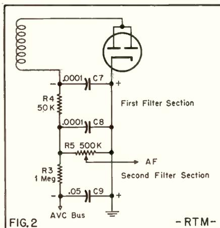
Two-section AVC filter, designed to prevent feedback of audio signal with control voltage.
