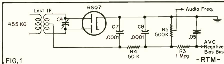
Note similarity of this AVC circuit to that of a full-wave rectifier.
