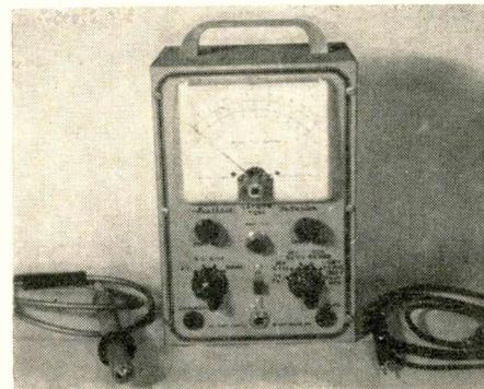
The author's VTVM with high-voltage probe at left and crystal RF probe at right
