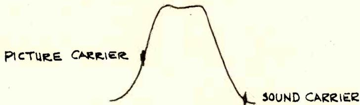
Fig. 3. RF response curve used for alignment of local oscillator.
