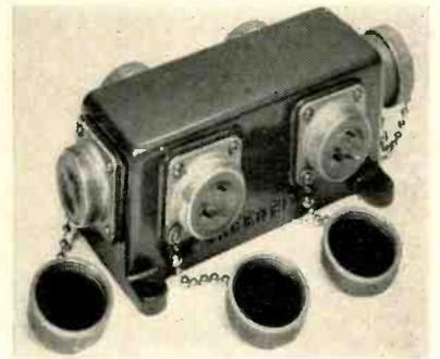
Input to the unit handles 6000 watts, while the five outputs will each handle 1500 watts. Sockets fit standard two-prong 110 v. plugs.
