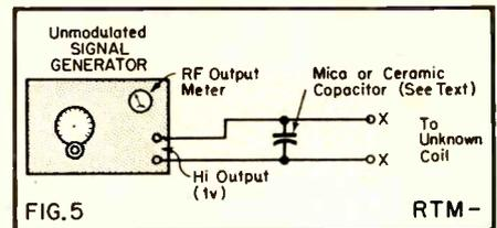
generator output circuit, effectively is in parallel with the tuned circuit under test and will influence the resonant frequency of the latter. Therefore, the measured frequency will be somewhat lower than the true resonant frequency unless care is taken to keep all stray capacitance low with respect to the circuit capacitance.
