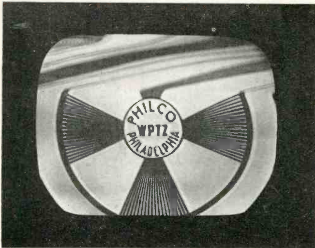
Fig. 4 Top distorted, horizontal hold control needs adjustment
