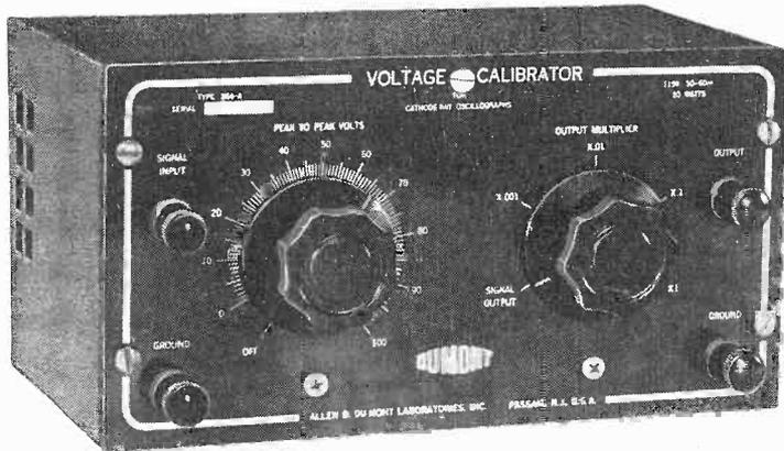
for peak-to-peak voltage measurements
