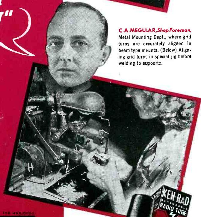
**C.A. MEGULAR, Shop Foreman,** Metal Mounting Dept., where grid turns are accurately aligned in beam type mounts. (Below) Aligning grid turns in special jig before welding to supports.
