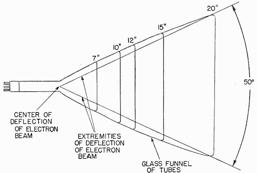
Fig. 9 Relative sizes of magnetic type television tubes.
