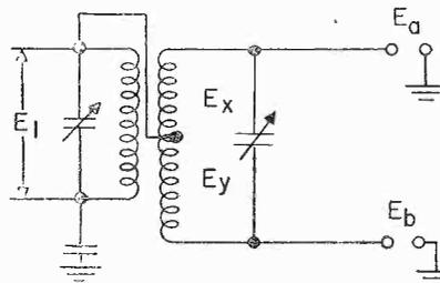
Fig. 4 Showing how two voltages  $E_A$  and  $E_B$  are produced for application to the plates of the diodes.  $E_A$  and  $E_B$  vary in magnitude as the frequency of the input changes.
