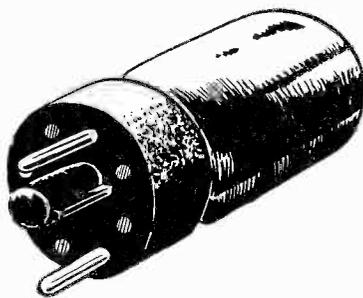
connected to the filament. If we remove a tube with similar filament rating and replace it with the dummy, that circuit has been made dead and we can test accordingly.
