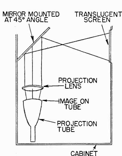
Fig. 10 Projection system using refractive lens.
