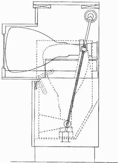
Fig. 6 Lift mechanism for 20" tube.
