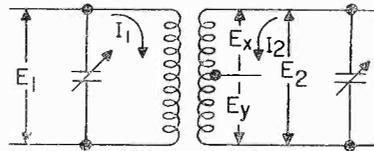
Fig. 3 Schematic of an IF coil with a center-tapped secondary winding such as used with Foster-Seeley and ratio discriminators.
