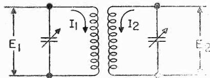
Fig. 2 A diagram of a double-tuned IF coil showing currents and voltages discussed in the text.
