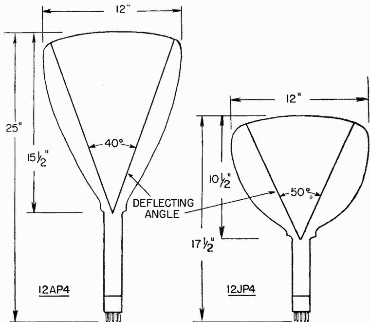
Fig. 8 Showing relative size and shape of old type 12AP4 and new type 12JP4 cathode-ray tubes. Though the screen diameters are the same, the new tube is approximately 7 1/2" shorter.
