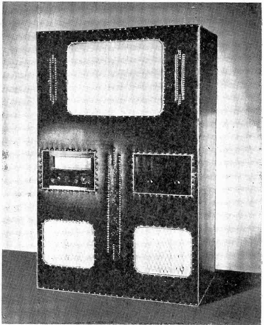
Fig. 13 New U.S. Television tavern type receiver using projection system. The picture size is 25 x 19 inches.
