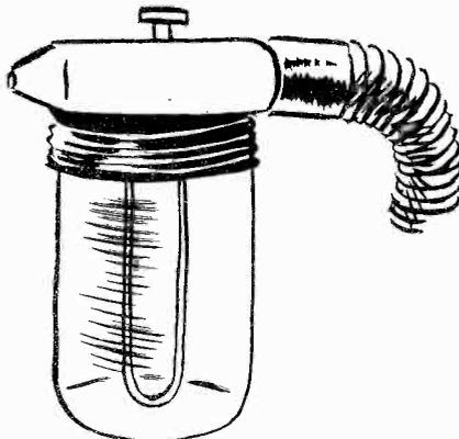
the sprayer head by means of the flexible cable to that point where the dust bag had been attached. The flexible cable is a part normally supplied with the machine and, therefore, does not represent any additional expense. A push-button affair on top of the sprayer head controls the flow of paint.
