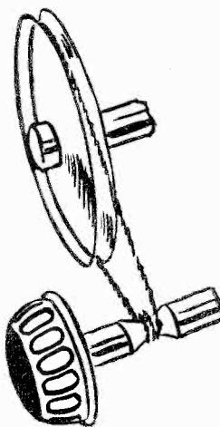
are used, trouble is experienced with the cord slipping off the drive shaft. This trouble can usually be eliminated by filing a slight groove around the shaft. A small rat tail file can be used for this purpose.
