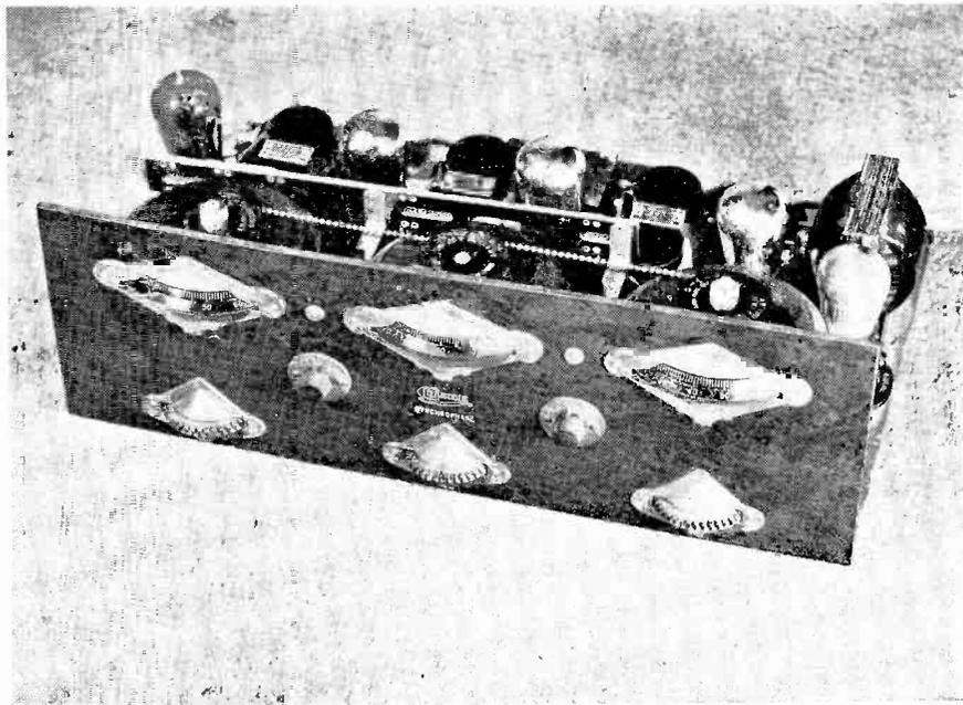
Fig. 3 The famous Grebe "Synchrophase," a battery-powered TRF receiver. This is one of the first receivers employing gang tuning, which was accomplished by a chain drive visible in the photograph.
