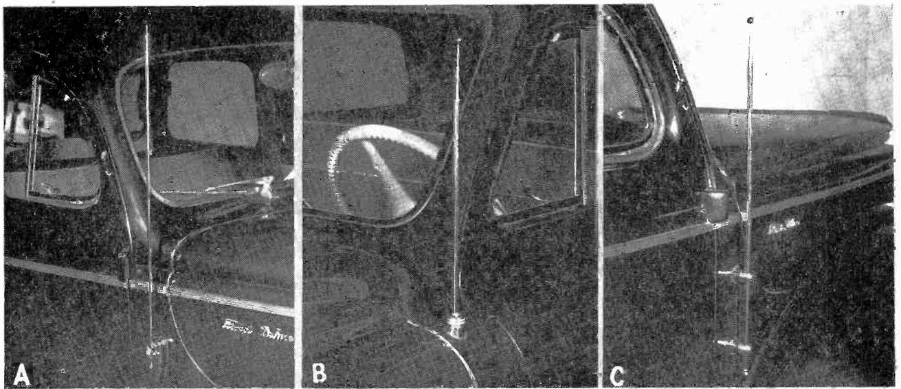
**Fig. 3 Three different types of auto antenna mountings: A, Adjustable side cowl; B, Concealed type installation with mast about two-thirds withdrawn from hidden shield tube; C, Non-adjustable side cowl type.**
