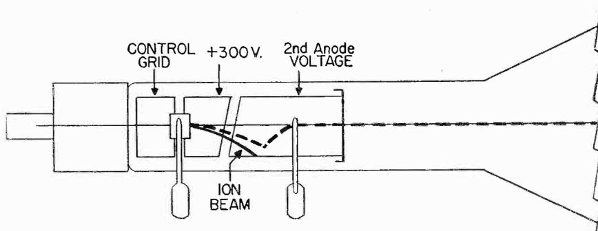
Fig. 2 This diagram shows the operation of the ion trap.
