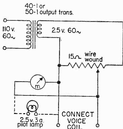
coil of the speaker being tested. Advance the wire wound resistor until the 60 cycle hum is heard in the speaker. This hum should be steady and the bulb should not flicker. Otherwise, an intermittent condition is indicated.
