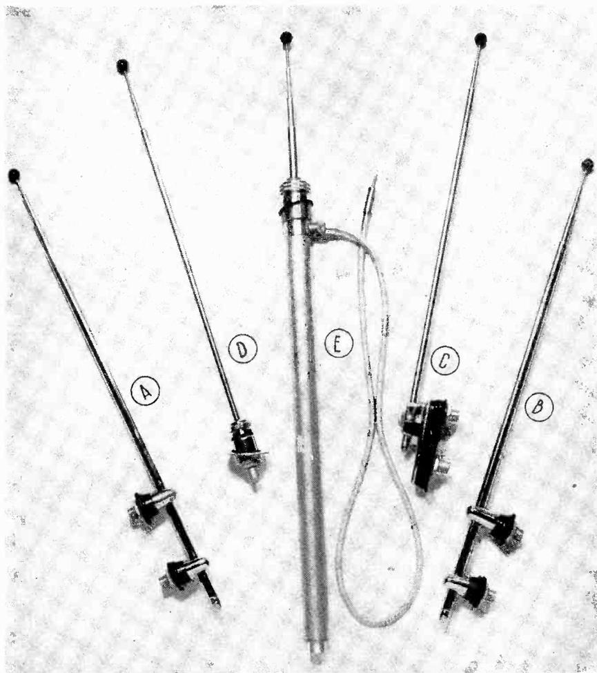
**Fig. 2** Some typical automobile antennas: **A**, Two-insulator type for vertical side cowls; **B**, Two-insulator type for torpedo or slanting side cowl; **C**, Adjustable side cowl type; **D**, Adjustable top cowl or top fender type; **E**, Concealed type.
