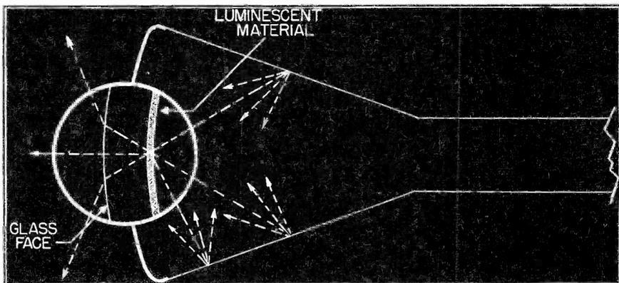
Fig. 3 Conventional cathode-ray tube showing typical distribution of light from a spot.
