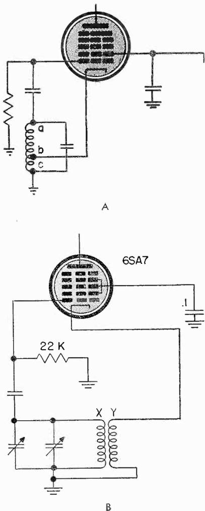
**Fig. 4** Similarity between the conventional "tapped coil" (Hartley) oscillator and the type used in the receiver described in the text.
