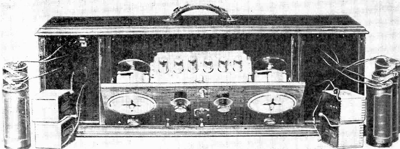
Fig. 6 A definite step forward was marked by the development of this Radiola battery powered superheterodyne.
