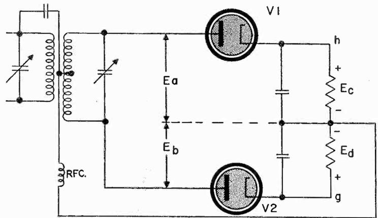
Fig. 6 Basic circuit of the Foster-Seeley discriminator. In practice, point g is usually grounded. Then the audio output appears at point h and AVC or tuning eye voltage can be obtained from the center tap of the resistor.
