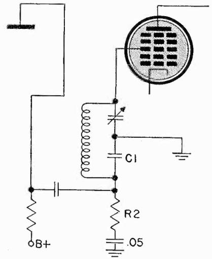
Fig. 3 Impedance coupling used in the RF section of the Buick Model 980744-5.
