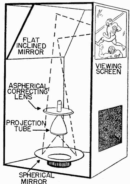
Fig. 12 Schmidt system in which picture is projected on opaque screen.
