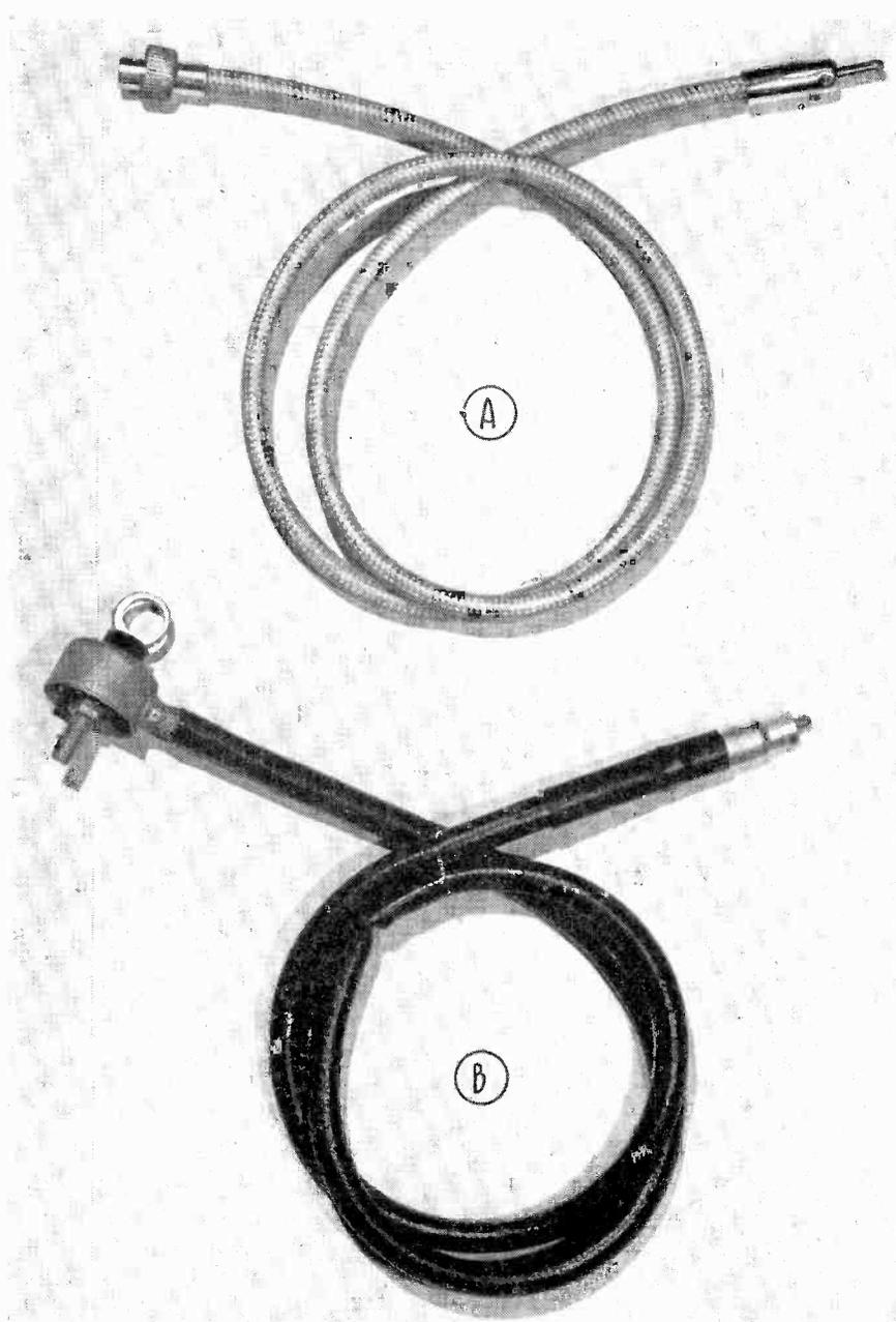
**Fig. 1 Two types of antenna lead-in cable for automobile use: A, Polyethylene insulated type; B, older type using paper loom construction and shield can fitting. Choice of lead-in cable can have an important effect on efficiency of the automobile receiver.**
