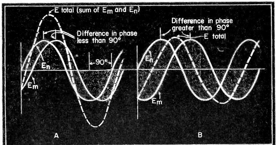
Fig. 5 Graphs of sine waves showing how two AC voltages can produce a sum voltage whose amplitude varies with a change of phase between them.
