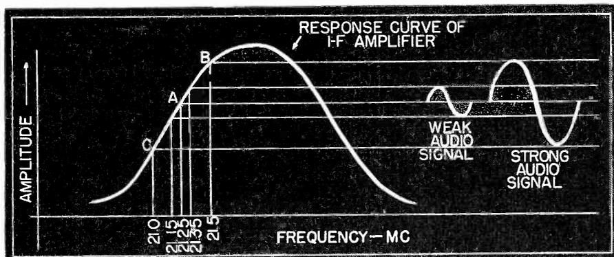
Fig. 1 How slope detection may be used to receive FM signals on an AM receiver. The frequencies shown are those used in the sound channel of a television signal.
