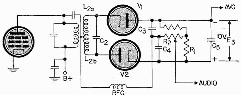
Fig. 8 The ratio discriminator. Below: Schematic diagram, Above: equivalent circuit discussed in the text.
