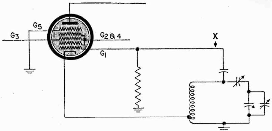
Fig. 7 6SA7 pentagrid converter.
