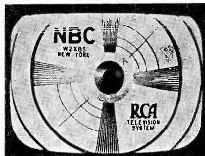
Fig. 11 A test pattern showing fold-over resulting from improper peaking of the vertical saw-tooth voltage.
