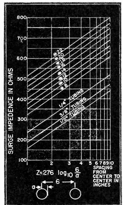
Fig. 4 A chart giving the impedance of two wire parallel transmission line (air dielectric) using various combination of spacing and conductor size.
