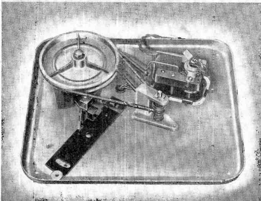
**Fig. 1 A toggle post drop type record changer. This type of record changer is rapidly gaining in popularity.**
