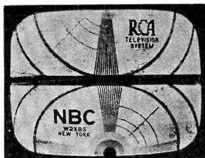
Fig. 9 A test pattern showing the loss of vertical synchronization.
