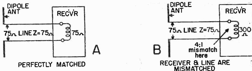
Fig. 6 Correctly and incorrectly matched antenna systems. In (A) the 75-ohm line matches at both the antenna and receiver ends; and, therefore, the match is correct. In (B) the 75-ohm line matches the antenna but does not match the input of the receiver.
