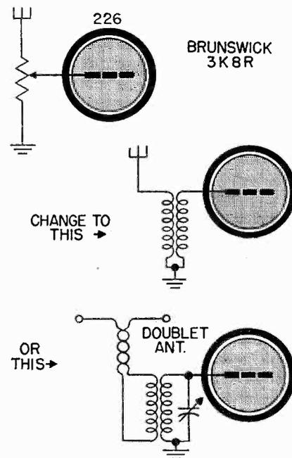
Fig. 2 Either one of the above methods of coupling the antenna is an improvement over the original.
