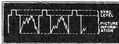
**Fig. 2** A video signal showing the combined sync pulse and picture information.
