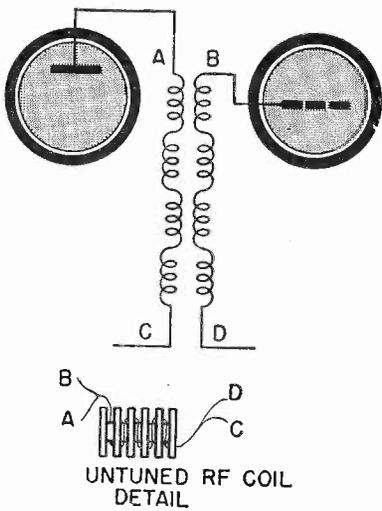
**Fig. 3** The construction of an untuned RF coil used in the older receivers.
