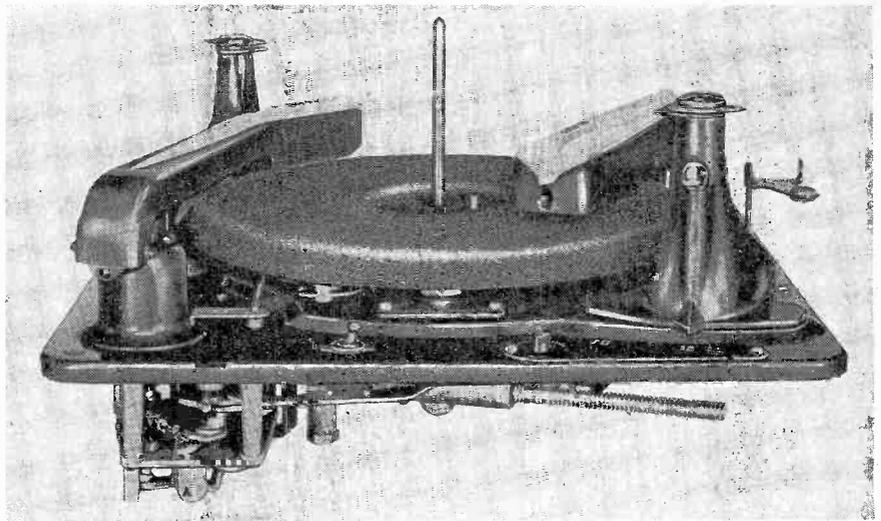
Fig. 2 The slicer type record changer. This changer is equipped with a recording as well as a playing head.
