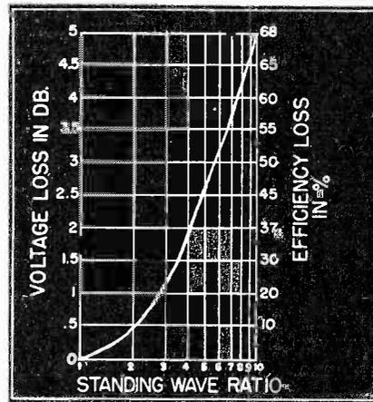
Fig. 2 A curve showing the voltage loss in db and the efficiency loss in per cent for various standing wave ratios.
