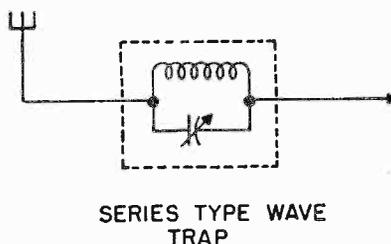
Fig. 6 A series type wave trap which can be constructed from an RF choke and a trimmer condenser.
