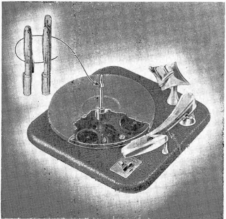
Fig. 3 A toggle post changer with an enlarged view of the spindle. The spindle on the left is in normal position; the spindle on the right is in position to drop a record onto the turntable.
