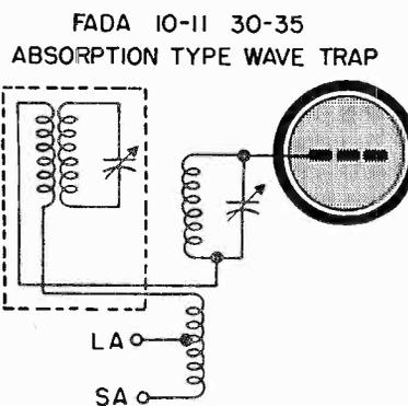
Fig. 5 An absorption type wave trap.
