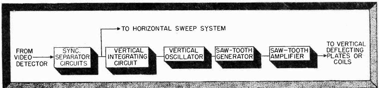
**Fig. 1** A block diagram of the vertical sweep system used in a television receiver.
