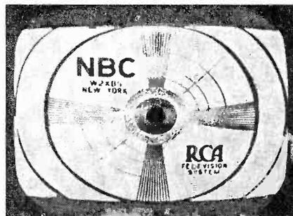
Fig. 10 A test pattern illustrating the effect of an incorrectly set vertical size control.
