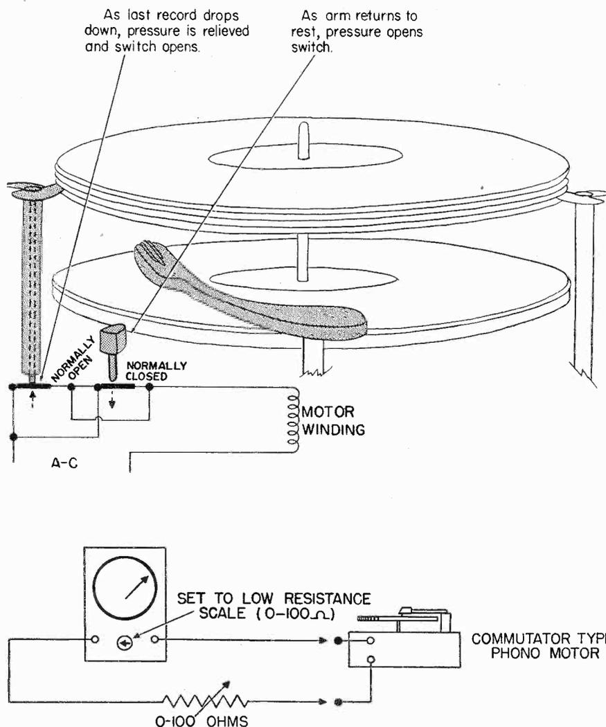
Fig. 5 A resistor and ohmmeter connected across the commutator as shown above is used to check brush contact as described in the text.
