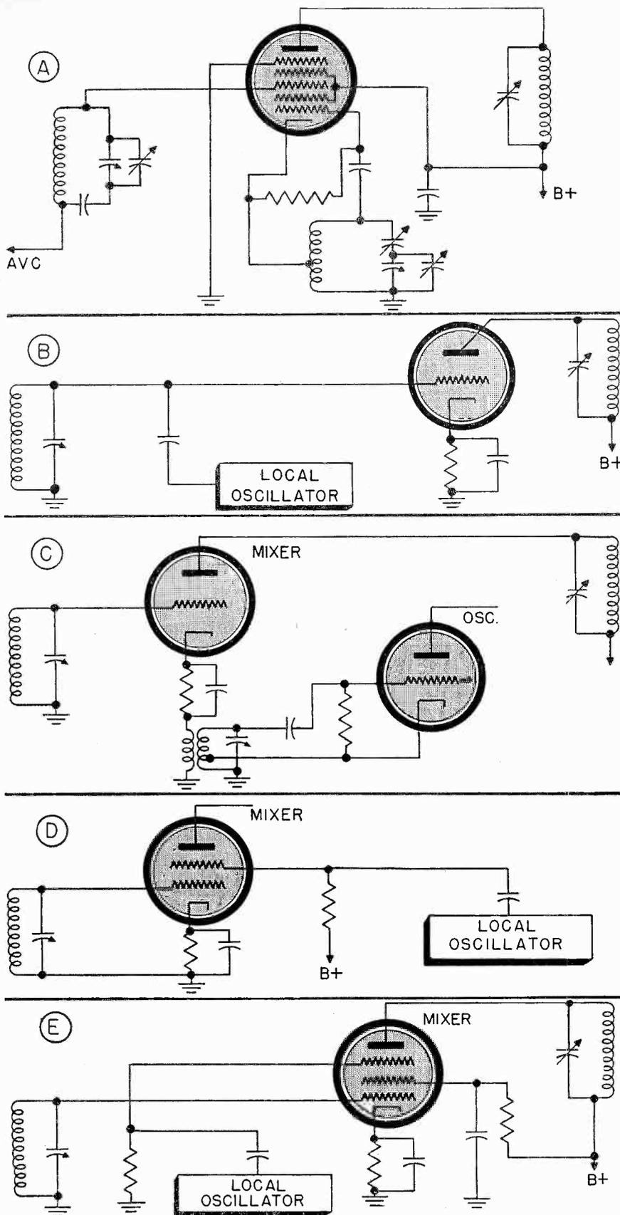
**Fig. 4** Five types of converter circuit: A, the pentagrid converter using electron coupling; B, control grid injection, capacitive coupling; C, cathode injection, inductive coupling; D, screen grid injection, capacitive coupling; E, suppressor grid injection, capacitive coupling.
