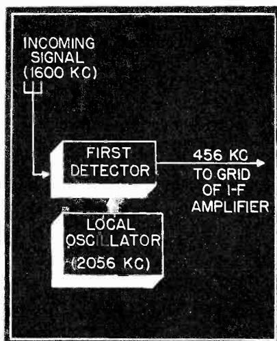
Fig. 1 A partial block diagram of a superheterodyne receiver showing the first detector and local oscillator.
