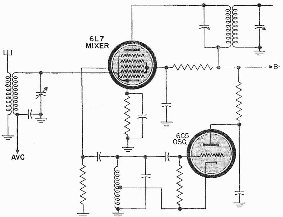
Fig. 5 A, the internal construction of a pentagrid vacuum tube. B, a schematic diagram showing a 6L7 pentagrid mixer.
