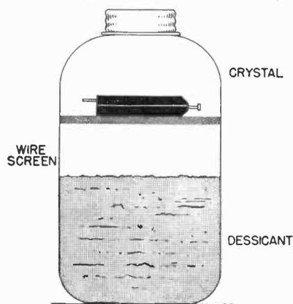
Fig. 8 A crystal cartridge may be stored in this way in humid climates to prolong its life. The desiccator consists of a jar with a piece of ordinary wire screen fitted into it to hold the cartridge above the desiccant liquid. The top should be closed tightly.
