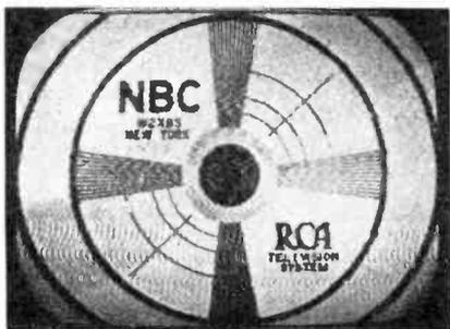
Fig. 19 A test pattern showing the effects of excessive diathermy interference.
