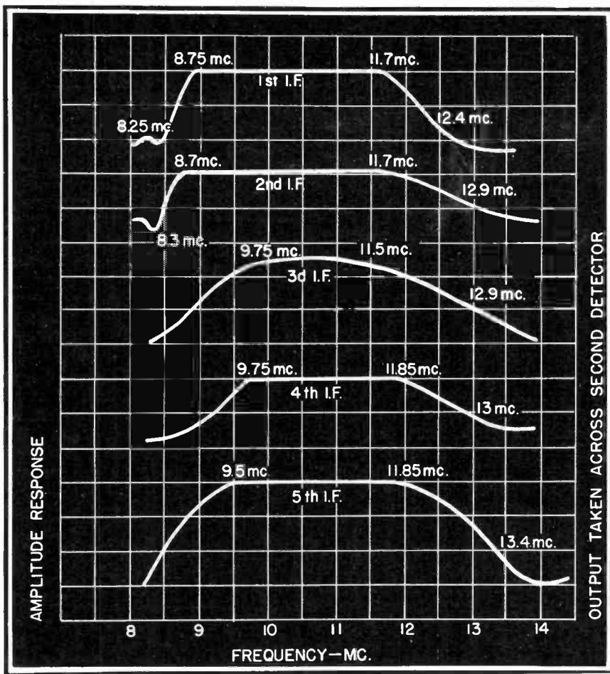
Fig. 14 The intermediate frequency response curves of a television receiver using five stages of intermediate amplification. Note the sound attenuation in the 1st and 2nd stages.
