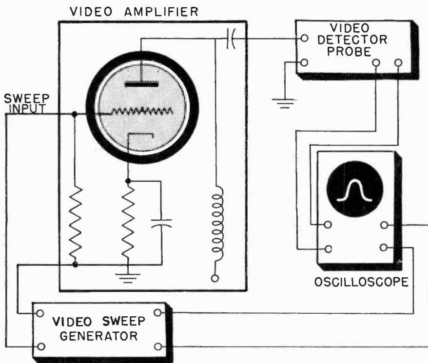
Fig. 8 A typical test set-up for testing the video amplifier response using the sweep generator method.
