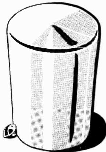
Fig. 2 Using a self-threading screw to ground an electrolytic.
