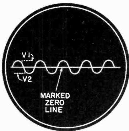
Fig. 5 The DC Voltage is indicated on calibrator voltmeter. The RMS value of the hum is equal to  $V_2$  minus  $V_1$  divided by 2.828.
