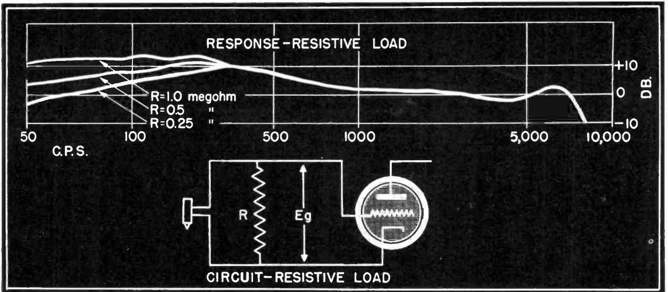
Fig. 5 Method used to connect a crystal pickup to an input stage. The curve above shows the effects upon the response of changes in the value of R. Decreasing the resistance decreases the low frequency response.
