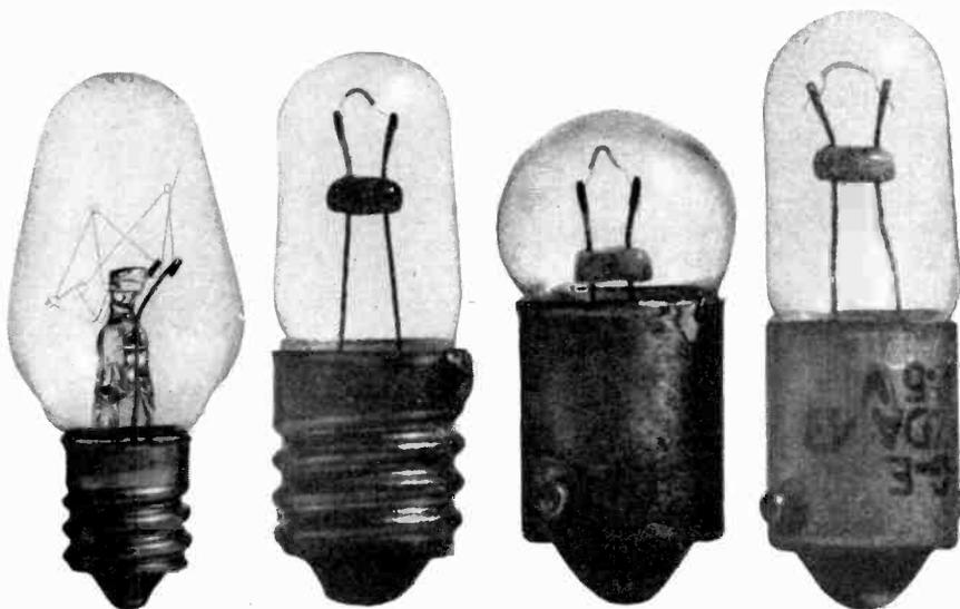
Fig. 1 The four common types of lamp construction. From left to right: The C-7 bulb with miniature screw base; the T-3 bulb with miniature screw base; the G-3 bulb with miniature bayonet base; the T-3 bulb with miniature bayonet base.
