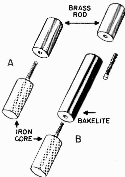
Fig. 1 Two types of wand can be made. The one with the bakelite center is more useful.
