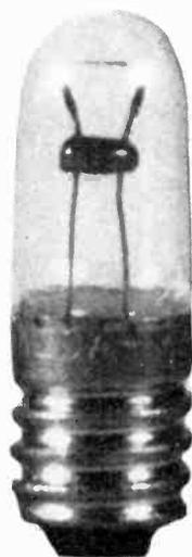
Fig. 7 The new lamp construction which eliminates the effects of vibration. Note the change in the bead position in relation to the filament.
