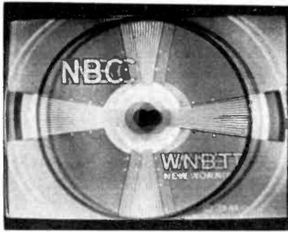
Fig. 17 Ghosts in a picture produced by reflections from structures in the neighborhood of the receiver.
