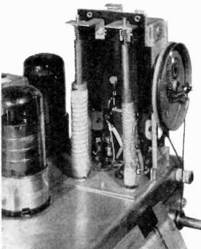
as the Vario-Tuner. The unit is designed to replace the coil and condenser combinations used in conventional broadcast receiver mixer and oscillator stages. It is more efficient, smaller in size, and easier to install than the older gang tuning condenser systems.
