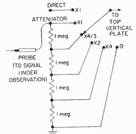
Fig. 3 A simple attenuator used to extend the measuring range of the oscilloscope. The attenuator should be mounted on a small box or chassis.
