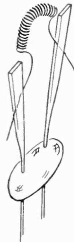
Fig. 3 New type lamp construction which eliminates noise interference.
