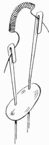
Fig. 2 Old type lamp construction which resulted in noise interference when subjected to vibration.
