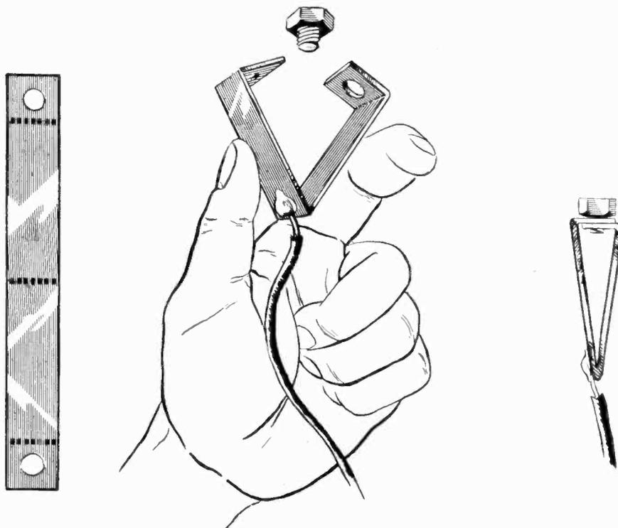
Fig. 3 This clamp is useful when making connections to automobile ammeters. It is made from a small strip of brass.
