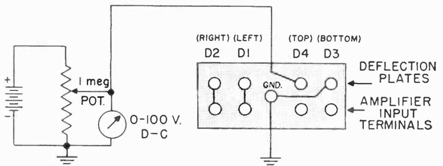
Fig. 1 Connections used when calibrating the oscilloscope. The terminal block shown is that used on the DuMont 208B but the same method can be used with other oscilloscopes.
