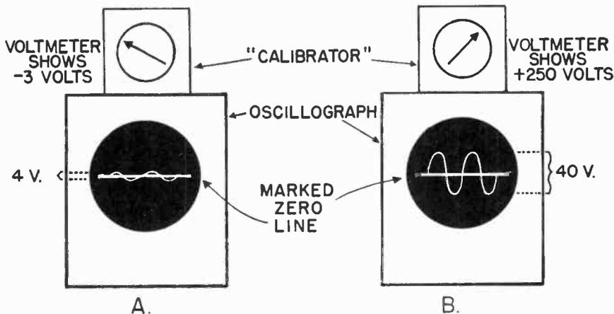
Fig. 6 A shows the pattern obtained at the input of the stage while B shows the pattern obtained at the output. This makes possible measurement of the gain of the stage.
