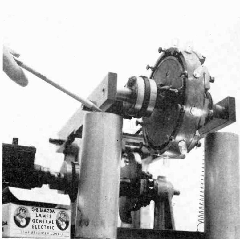
Fig. 9 This gadget is used to check the shock resisting qualities of panel lamps.
