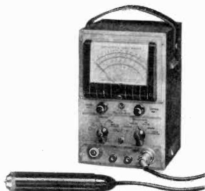
ures voltages up to 1000 volts and resistances of from zero to 1,000 megohms.
