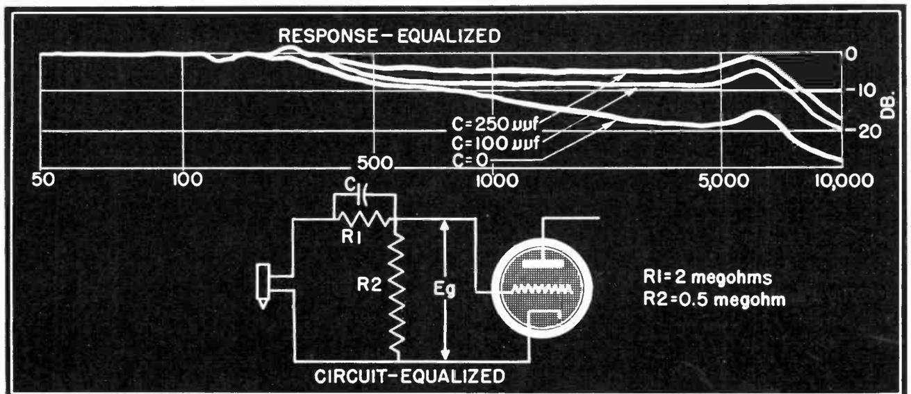
Fig. 6 In this circuit an equalizer has been added. The capacitance C affects the high frequencies while the resistances R-1 and R-2 primarily affect the bass response. The curve shows the effect of various values at C.
