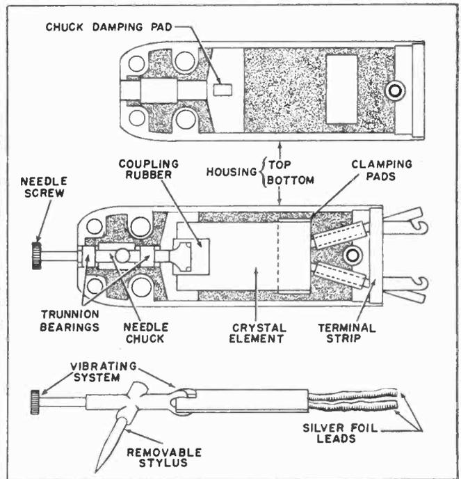
REPLACEABLE NEEDLE CARTRIDGE
