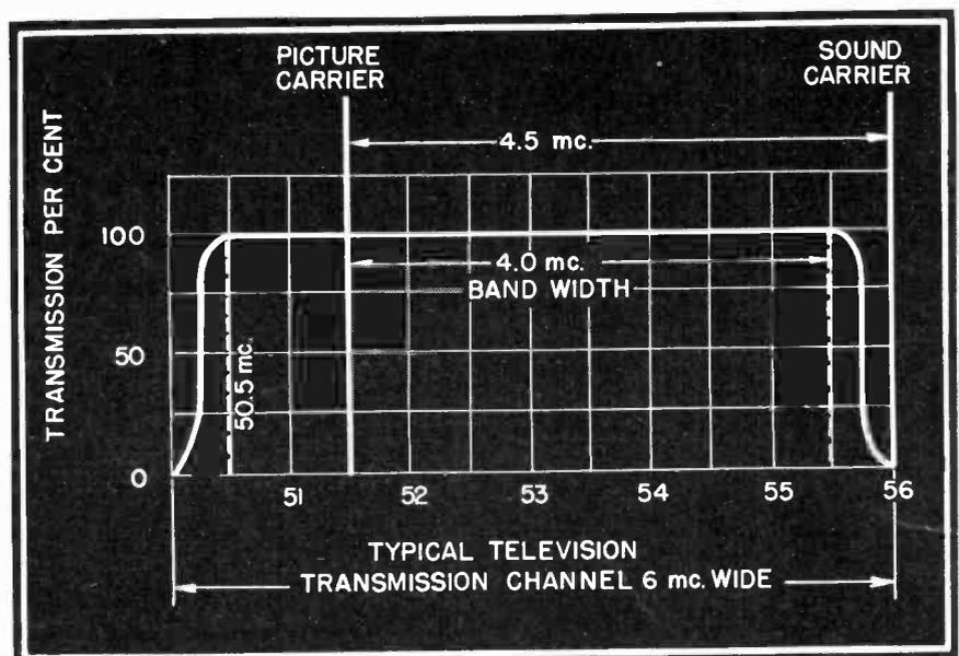
Fig. 4 A typical 6 Mc television channel.
