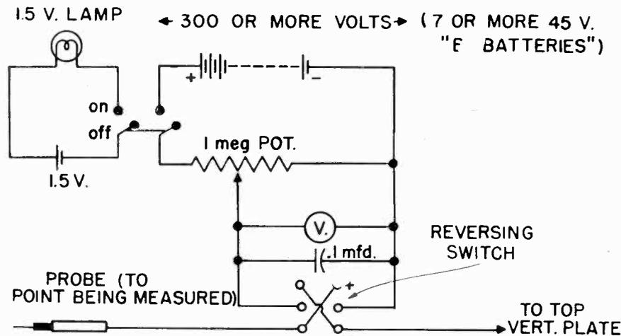
Fig. 4 The above arrangement is used as a calibrator. It is particularly useful when studying complex waveforms.
