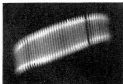
Fig. 8 When the new lamp is subject to vibration, the filament moves back and forth but it does not bend.
