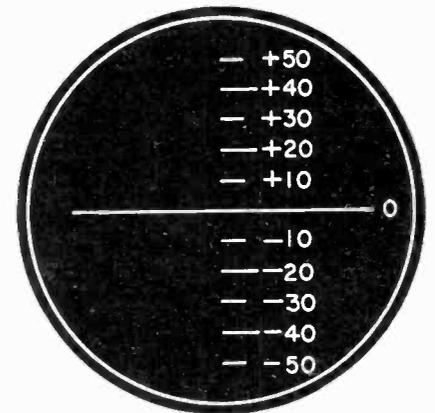
Fig. 2 An Oscilloscope screen calibrated by the method explained in the text. The markings are made with a soft red or blue china marking pencil.
