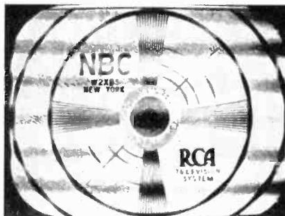
Fig. 3 A test pattern showing sound modulation in the picture caused by improper alignment of the sound traps.
