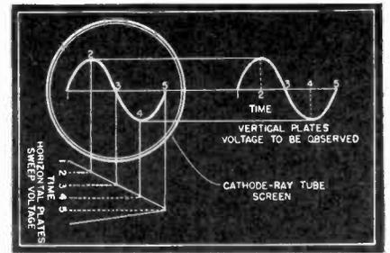
**Fig. 3** A graphic illustration of the relation of the vertical signal and the horizontal sweep voltages.
