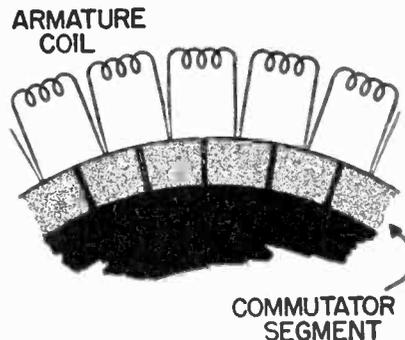
Fig. 4 Armature connections used in some types of phono motors.
