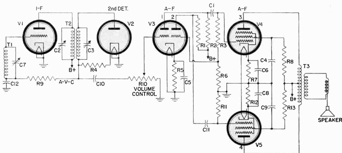
Fig. 3 Partial diagram of a superhet receiver using a phase inverter and push-pull output.
