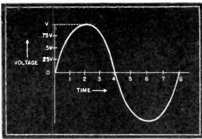
**Fig. 1** Voltage units plotted against units of time give a graph as shown above when the voltage is varying in sine wave fashion.
