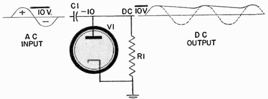
Fig. 2 The AC input is rectified by the diode and fed to the meter circuit.
