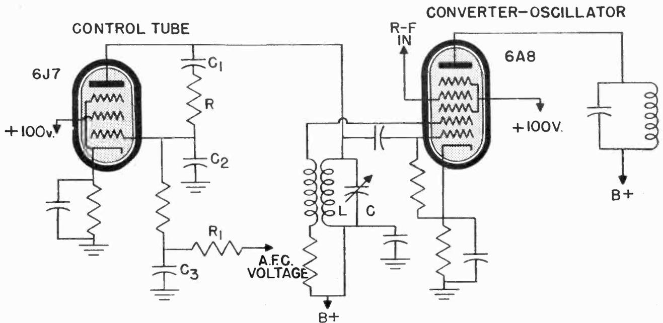
Fig. 5 Simplified diagram of the control tube circuit and the converter-oscillator circuit in a receiver using automatic frequency control.
