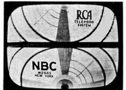
Fig. 12 A test pattern with the vertical synchronization control incorrectly set—the picture moves continually, giving a rolling effect.
