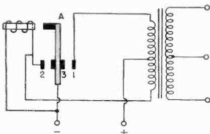
Fig. 6 The primary circuit of a vibrator supply.
