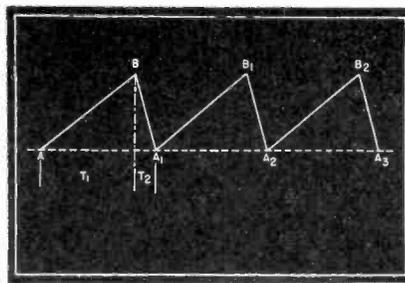
**Fig. 2** A saw-tooth voltage of the type shown graphically above is required to form the time base on the face of the cathode-ray tube.
