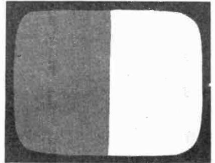
Fig. 19 The pattern produced in the horizontal scanning amplitude test with a 15,750 cps signal on the grid.
