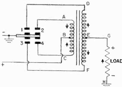
Fig. 9 A circuit diagram for a synchronous type vibrator supply.
