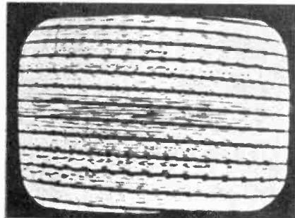
Fig. 17 A test pattern with the horizontal frequency control incorrectly set.
