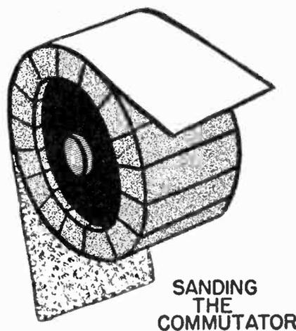
Fig. 2 Method used to smooth the commutator with sandpaper.
