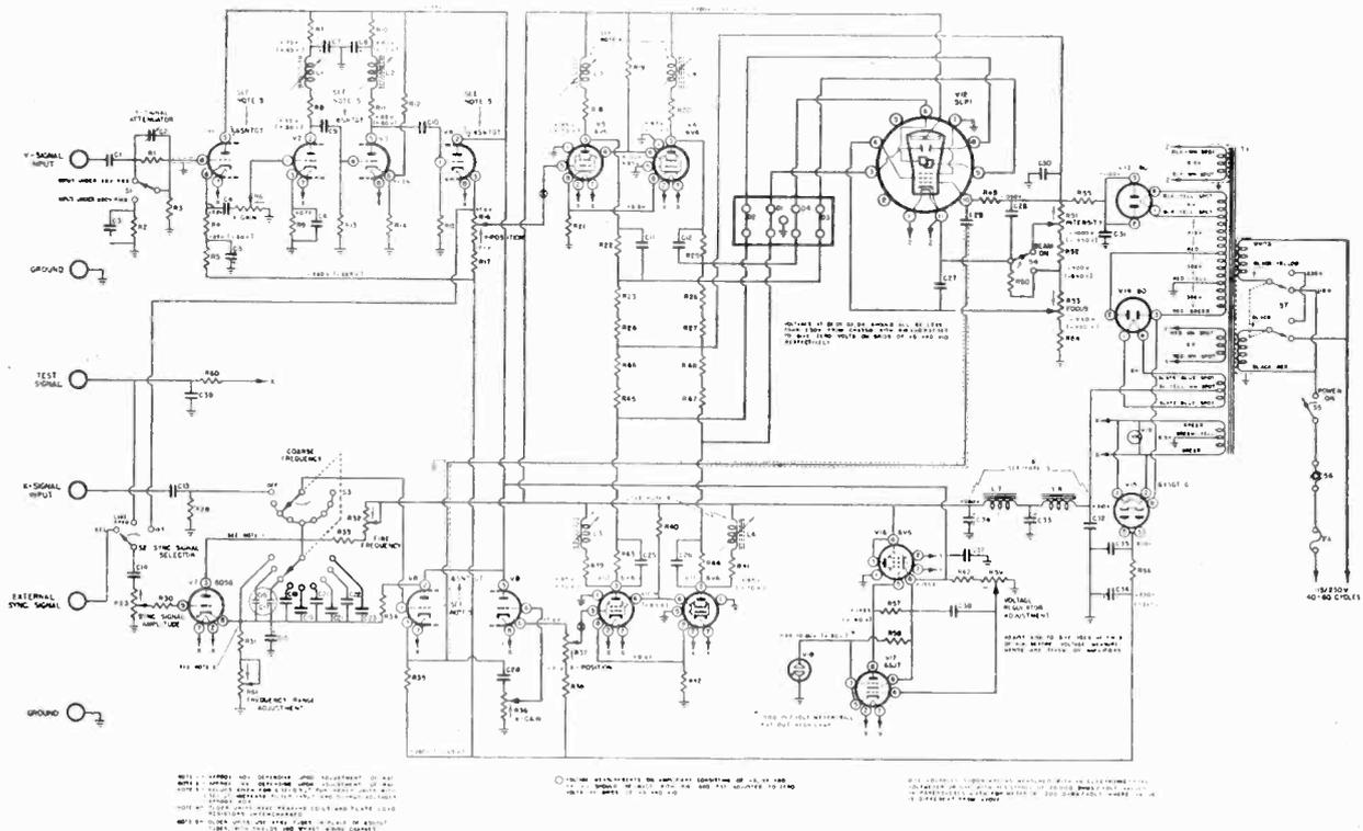
Fig. 5 The complete circuit diagram of the DuMont 208B oscillograph.
