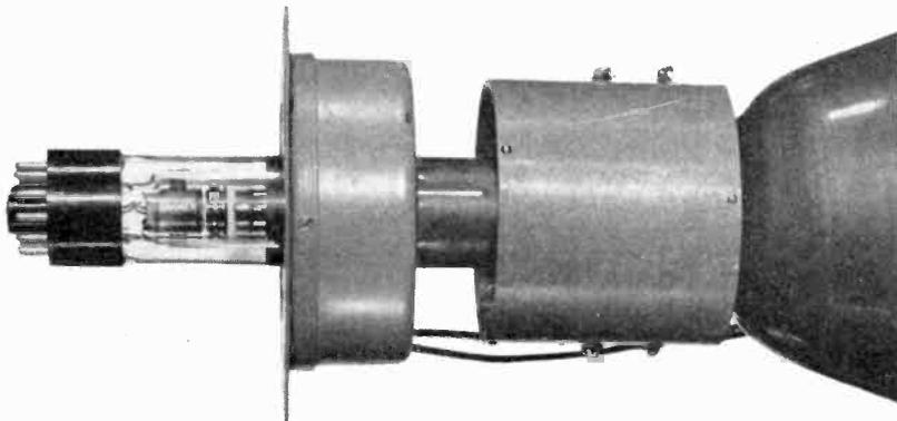
Fig. 5 The arrangement of the focus coil and the deflection yoke on a magnetically focused and deflected tube.
