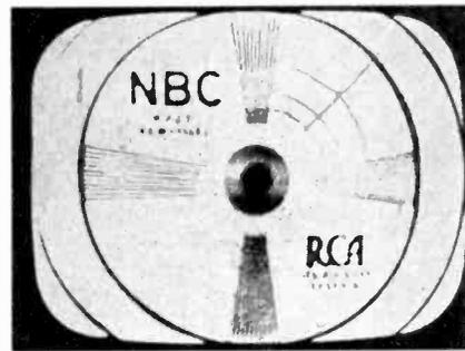
Fig. 3 Test pattern with focus control incorrectly set.
