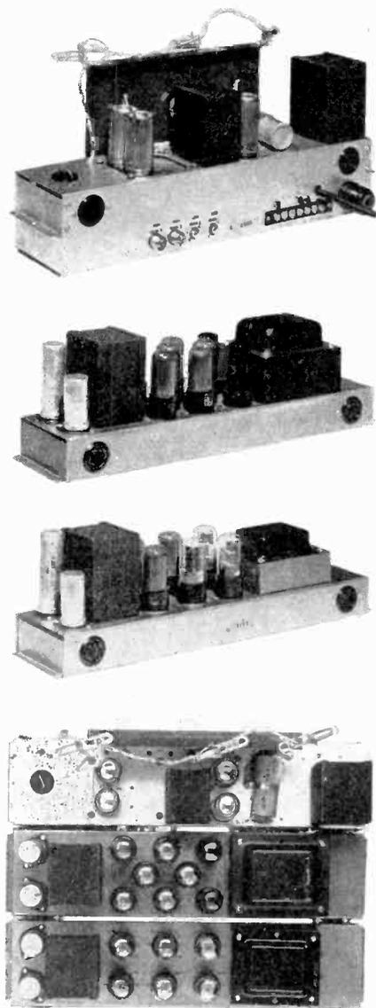
**Fig. 1** The three upper units, a four-channel input unit, a 30-watt amplifier stage, and a 40-watt amplifier stage are plugged together as shown by the photo at the bottom to make a complete 75-watt amplifier.
