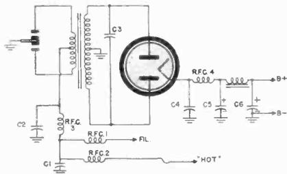
Fig. 11 Complete Power Supply.
