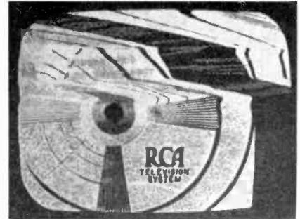
Fig. 18 A test pattern showing the picture tearing due to unstable horizontal synchronization.
