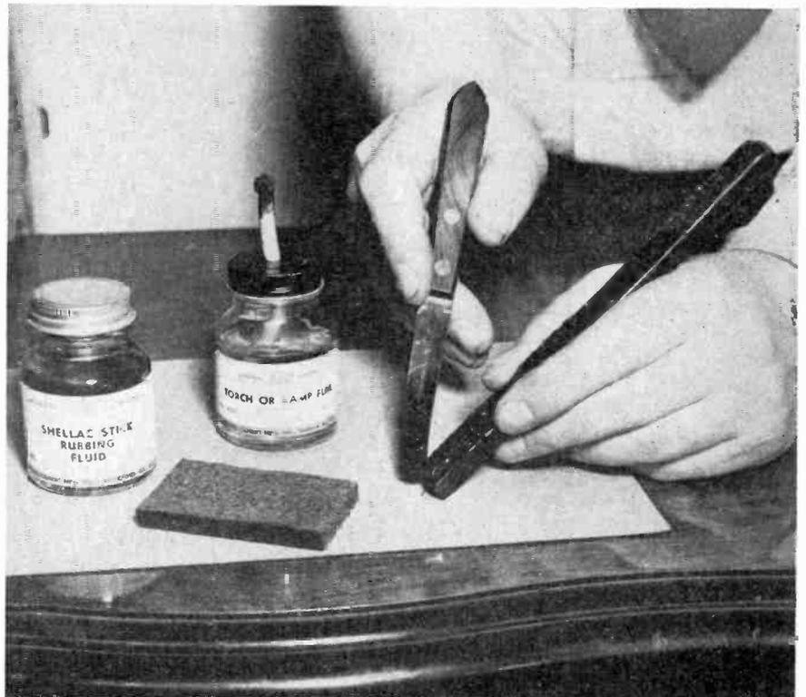
Fig. 4 Melt a portion of the shellac stick onto the hot spatula.
