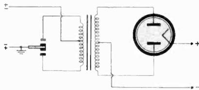
Fig. 8 A rectifier tube is connected to the secondary to rectify the voltage stepped-up by the transformer, thus giving high DC potential in the output.
