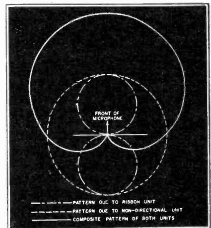
Fig. 3 Addition and subtraction of the sound energy received by the two sections of the uni-directional microphone produce the overall pattern known as a Cardioid.
