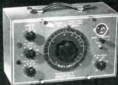
Model 904 Capacitance/Resistance Bridge.  $\frac{1}{4}$  mfd./ohm thru 1,000 mfd./megohms; 0-50% power factor; 0-500 volt adjustable internal polarizing voltage; 0-10 and 0-100 ma. electron-ray leakage current meter; measures resistance, capacitance under actual operating voltages! Only \$49.90.
