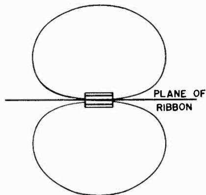
Fig. 4 Directivity curves for velocity or ribbon microphones.
