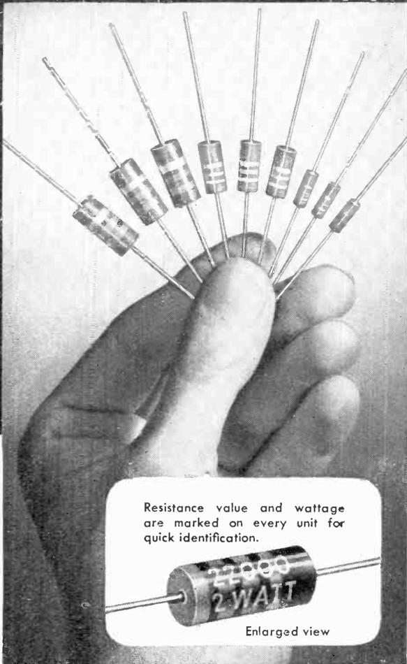
Resistance value and wattage are marked on every unit for quick identification.
