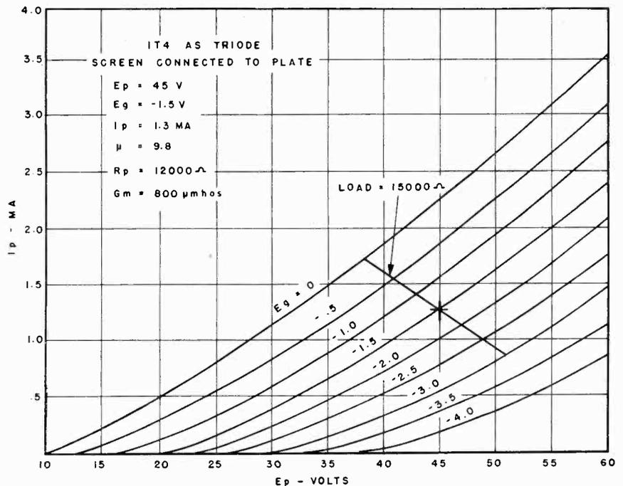
Fig. 3 Plate family for 1T4 connected as a triode.
