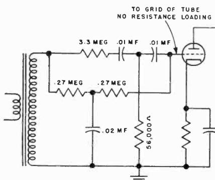
Fig. 1 R-C network in grid circuit of input stage to compensate for droop in low-frequency response of magnetic pickups.
