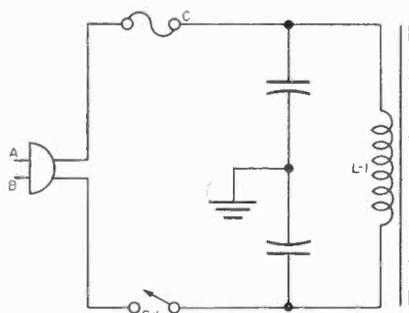
Fig. 1. Typical line power circuit for A-C receiver.
