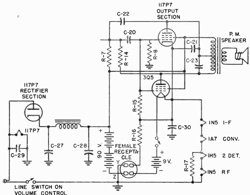
Fig. 1. Output system and method of securing filament current for R-F, converter, I-F and 2nd detector — first audio tubes.
