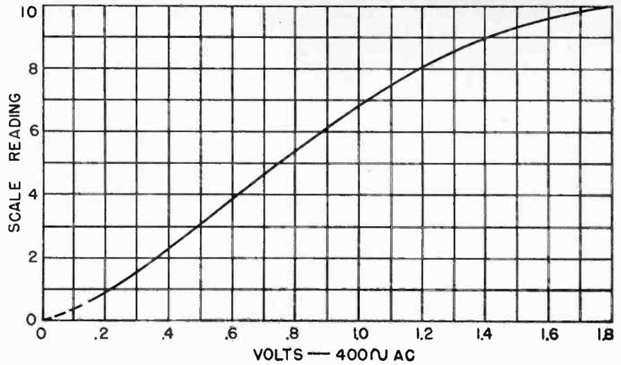
Fig. 2. Curve showing sensitivity of signal tracer, with input volts plotted against arbitrary units with which meter dial is calibrated.
