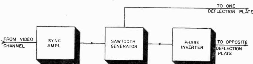
Fig. 4. Block diagram of elements of a typical sweep generator.
