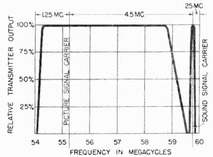
Fig. 1.—Frequency division of typical television channel.
