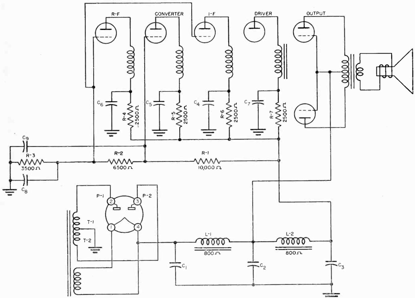
Fig. 3. D-C power distribution throughout 7-tube super-heterodyne.
