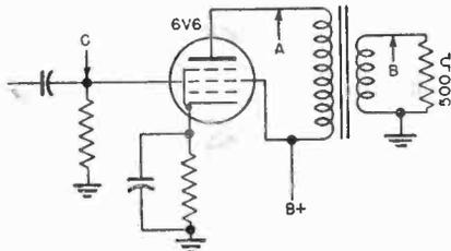
Fig. 5. Typical circuit of 6V6 output tube, used in determination of transformer impedance ratio and gain of the stage.
