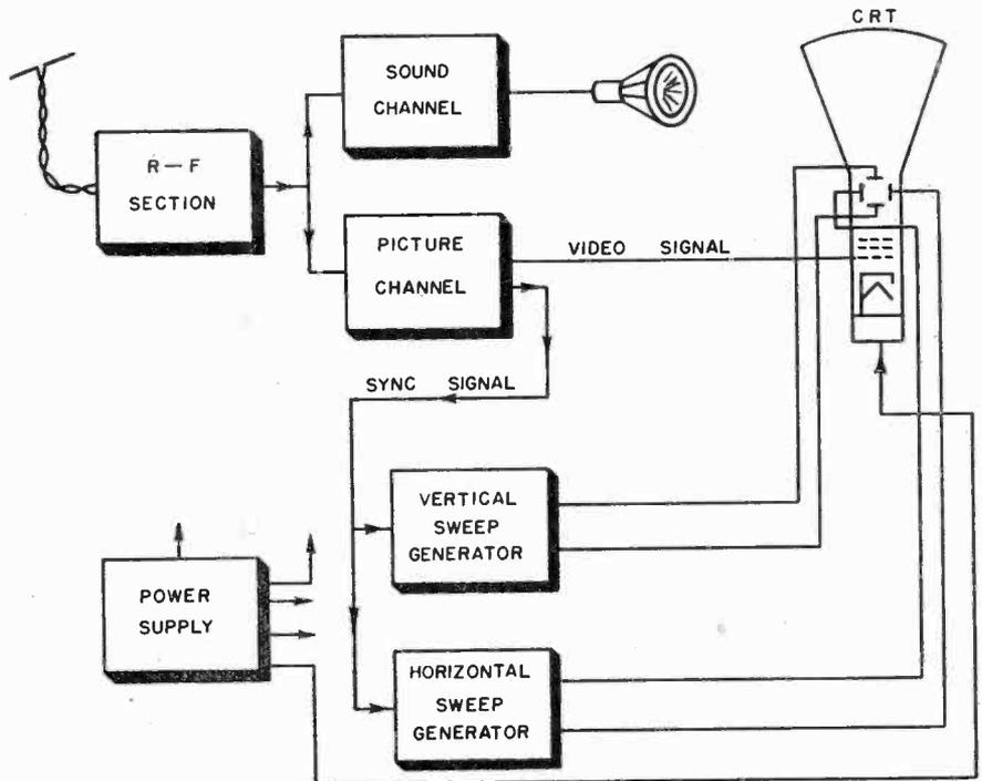
Fig. 2. Major sections of typical television receiver showing function of each portion of the circuit.
