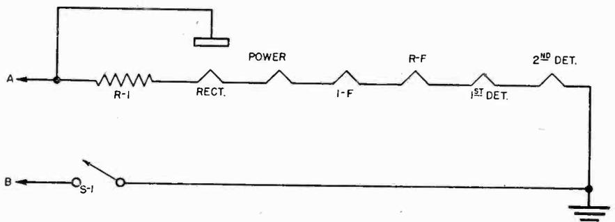
Fig. 2. Line power circuit for six-tube AC-DC set.
