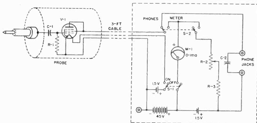
Fig. 1. Schematic of CA-11 Signal Tracer, applications of which are discussed in this article.
