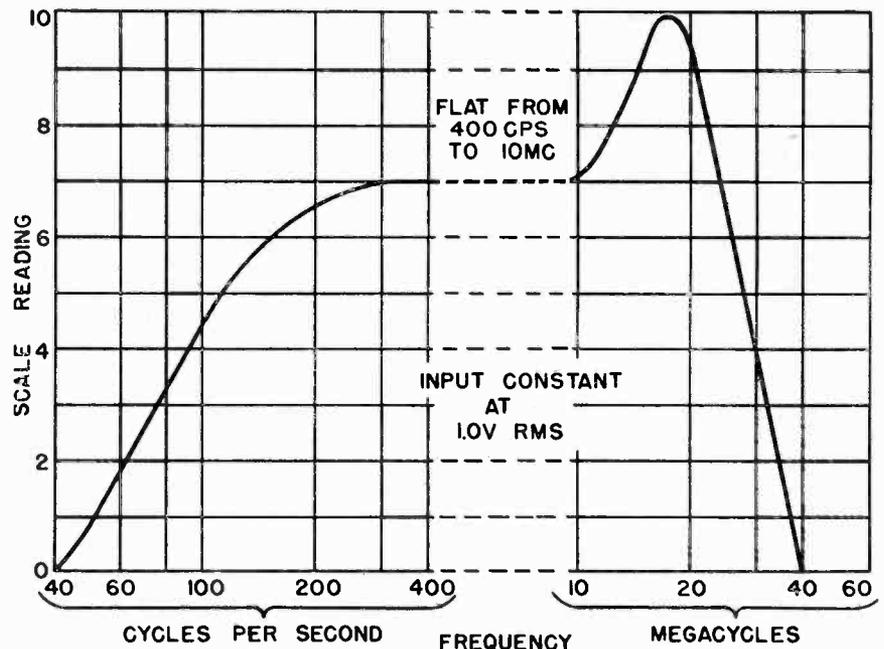
Fig. 3. Frequency response curve, flat over most useful range of frequencies, with reduction in sensitivity at low frequencies to reduce hum readings. Peak at 17 mc is caused by resonance in probe circuits.
