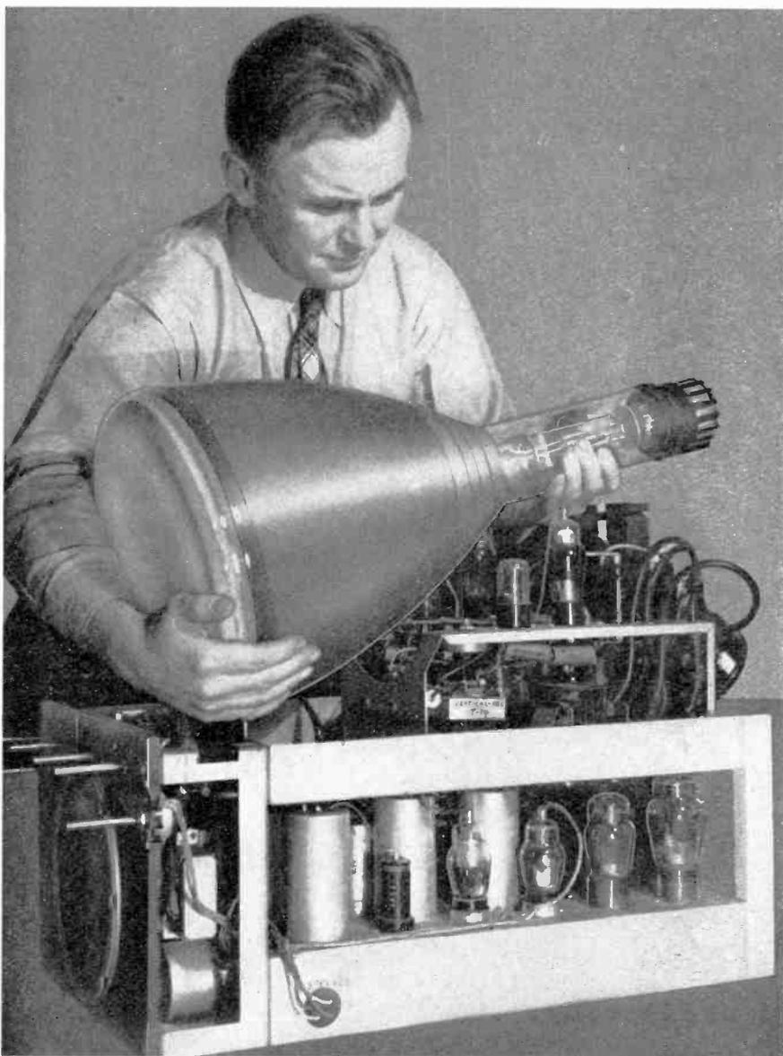
The author removing the cathode ray tube from a television receiver. Notice the way in which the tube is held while being removed.
