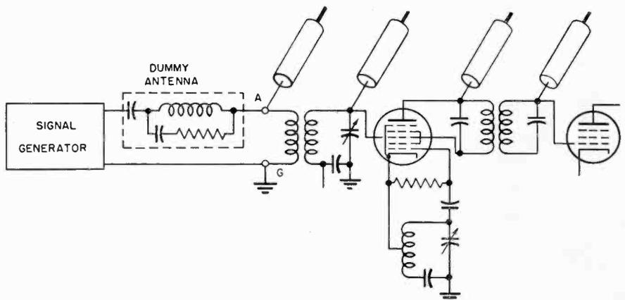
Fig. 4. Method of using tracer to follow passage of signal from stage to stage.
