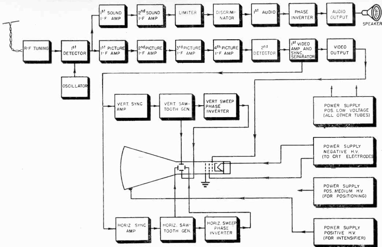
Fig. 3. Complete functional block diagram of the various stages in a large television receiver.
