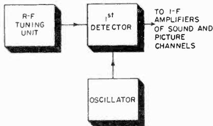
Fig. 5. R-F, first detector, and oscillator arrangement in R-F section of television receiver.
