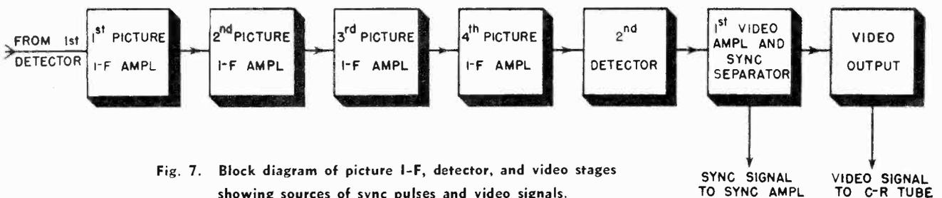
Fig. 7. Block diagram of picture I-F, detector, and video stages showing sources of sync pulses and video signals.
