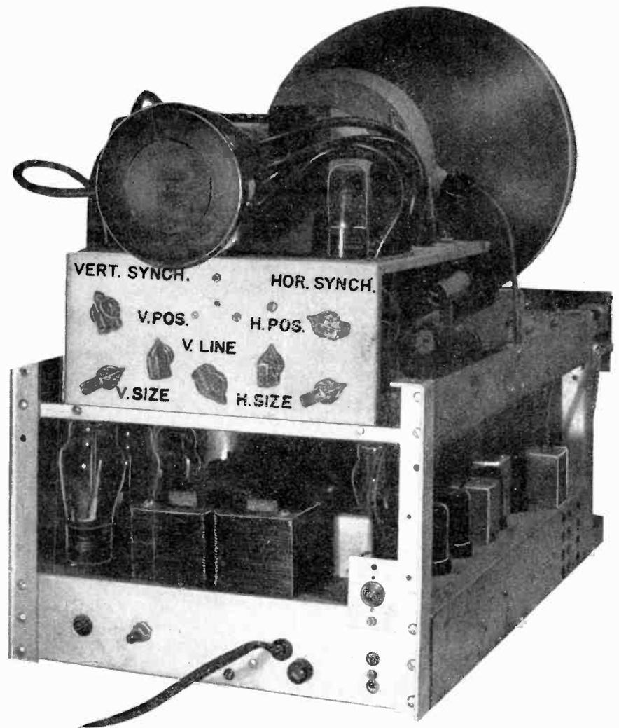
Rear view of a table model television receiver showing controls.
