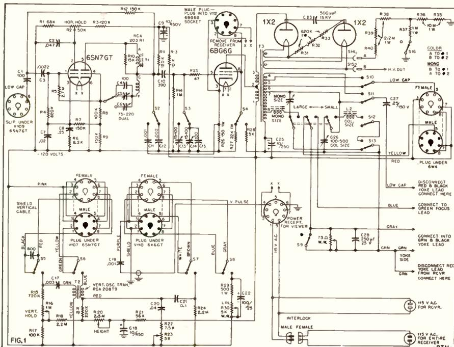
Adapter recommended by CBS for use with RCA 10-inch set, Model 9T246. It may be used with other sets with slight modifications.
