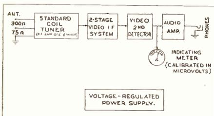
Block diagram of the Simpson Field Strength Meter. Tuner is Standard Coil unit identical with that found in TV receivers.
