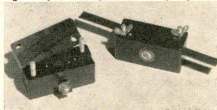
Lightning arrester which may be used for four-wire rotator control line or for standard 300-ohm twinlead.
