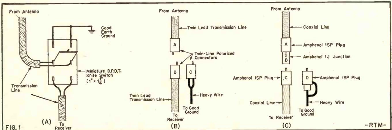
Methods of switching downleads to connect directly to ground during thunderstorms.
