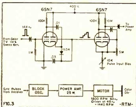
FIG. 3 Frequency divider and multivibrator for synchronizing motor speed with color signal. (top). Block diagram of hookup is shown at bottom.
