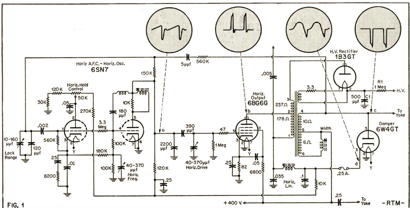
Test points and proper waveforms to be found when checking flyback HV supply.
