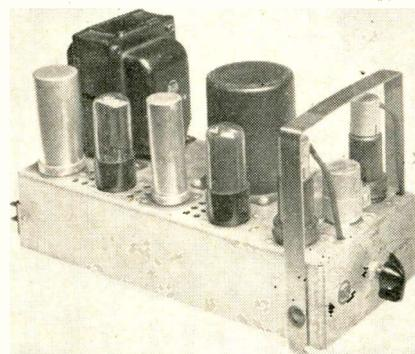
driver supplying voltage for power amplifiers, a monitor to supply audio power up to two watts for a speaker, and a bridging unit for a low impedance line.
