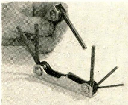
The wrenches fold into the handle of the device jack-knife fashion, so that the tool, when folded is small enough to fit the pocket, but provides good leverage when open.
