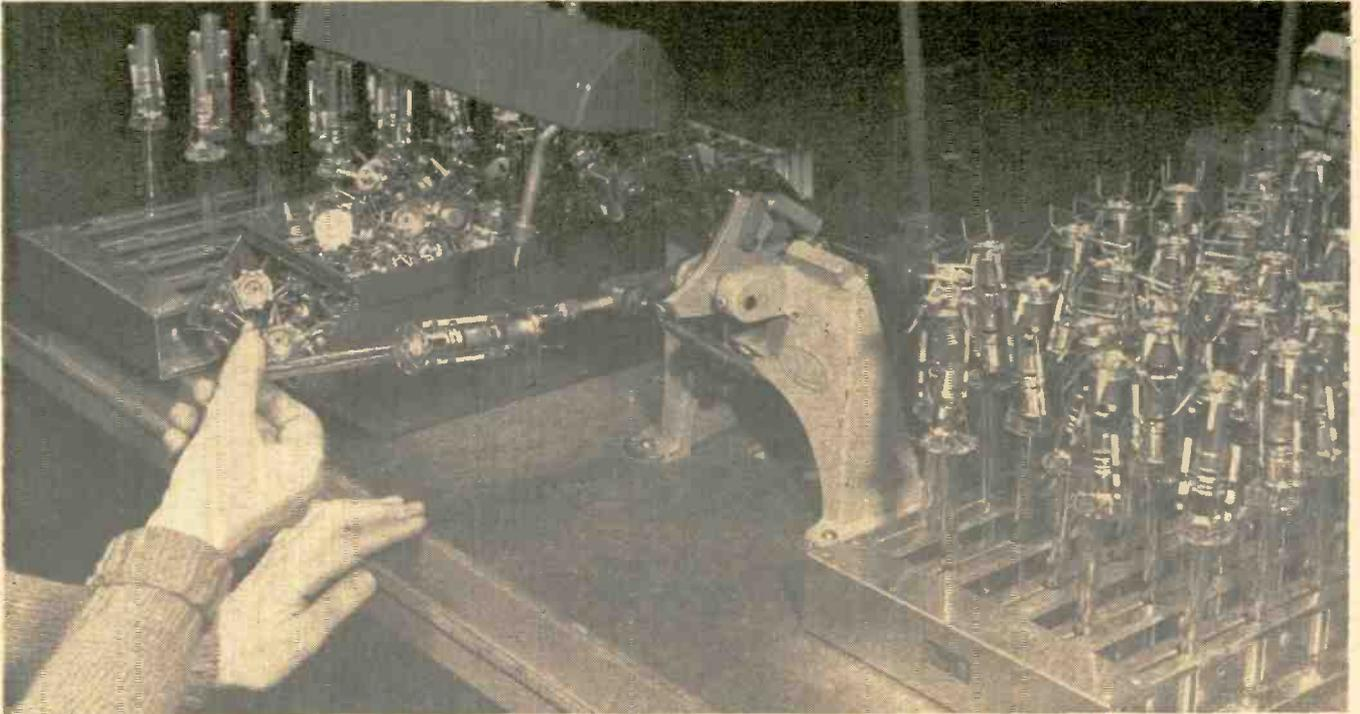
One of the many critical process in the manufacture of bent-gun assembly for Du Mont kinescope tubes is the welding of spacers to the body of the unit. Spacers keep the electron emitter in the precise position necessary to insure accurate sweep over the entire face of the tube,
