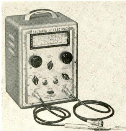
provides frequencies ranging from 15 to 240 Mc in four bands: 15-30 Mc; 30-60 Mc; 60-120 Mc, and 120-240 Mc. With an appropriate crystal inserted in the panel socket, oscillator will operate at any frequency between 2 to 20 Mc, and will provide useful harmonic output up to the sixth for all band calibration.
