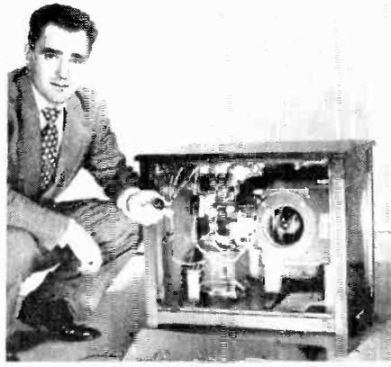
Rear view of the projection unit installed in its cabinet. Lens at right directs picture to movie screen set up behind the unit. Table-model TV receiver is mounted on the top surface. Controls and selector switch are on the front of the cabinet.
