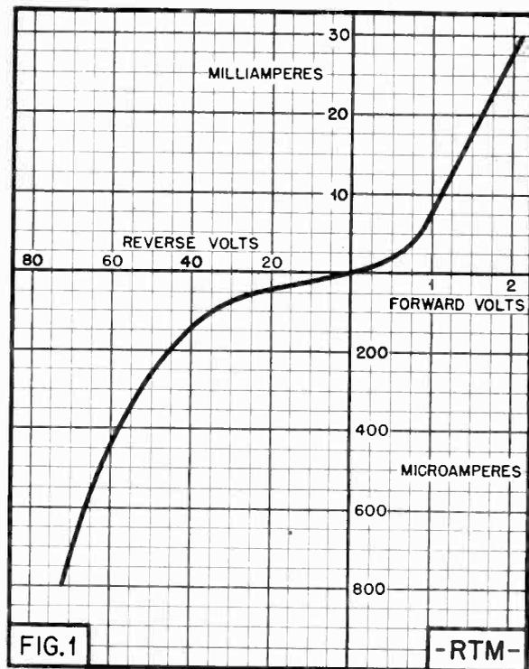
Current-Voltage characteristic of 1N34 diode.
