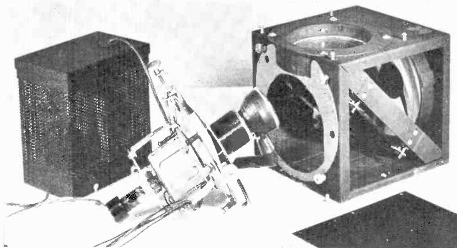
View of power supply, 2-1/2 inch picture tube and optical assembly of Duo-Vue projection unit. Unit with its cabinet serves as a table when used with a table-model direct view receiver. Projection unit contains only projection tube, optical system, power supply, and auxiliary chassis with extra video amplification.
