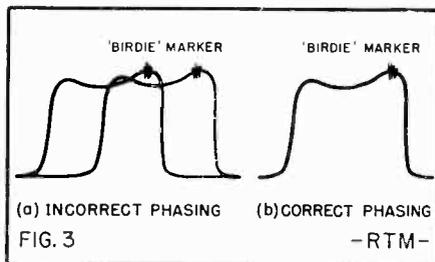
marker oscillator is a separate oscillator such as a Hartley, whose frequency is adjustable over the full range of center and deviation frequencies. The output of the marker oscillator is impressed upon the final amplifier tube of the sweep frequency circuit. When the wobbulator output is rectified and examined on an oscillograph, a "birdie" is visible at the point where the instantaneous frequency of the wobbulator and
