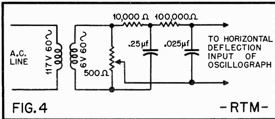
Network used to bring sweep voltage into phase with wobbulator deviation. Correct adjustment results in in-phase trace shown above in Fig. 3(b).
