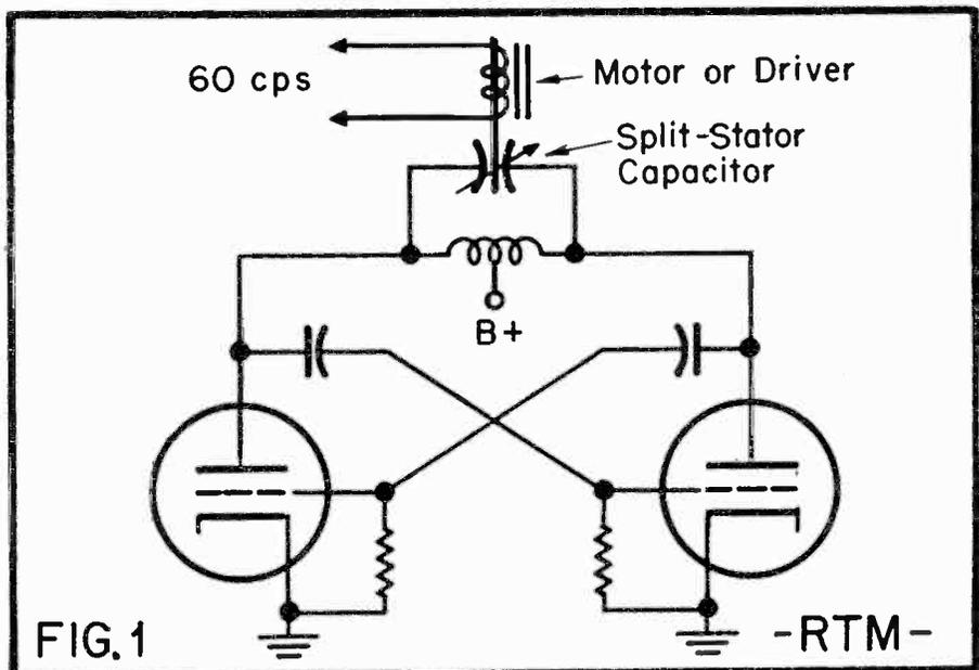
Rotating capacitor method of varying oscillator frequency. The motor, an 1800 or 3600 rpm synchronous type, drives the rotor of a continuously variable condenser. Capacitance varying constantly from minimum to maximum modulates oscillator frequency at 60 cycles.
