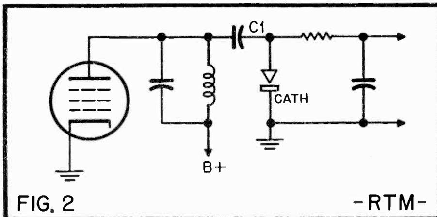
Shunt detector circuit, illustrating possible surge-current overload of germanium diode. In initial application of power, charging of C may be large enough to damage the germanium unit.
