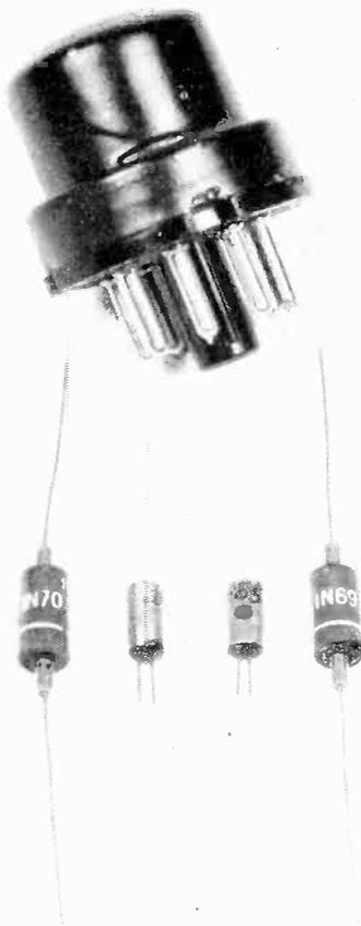
The 1N70 has a working voltage rating of 100 volts, peak current of 90 milliamperes, average current of 30 milliamperes, surge current of 350 milliamperes and maximum operating temperature of 70 degrees centigrade.
