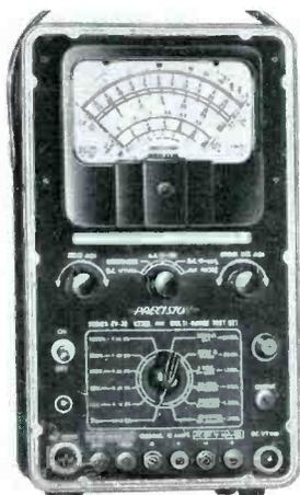
meg, 12 amp, plus 64 db, and d-c vtvm ranges to 12,000 and 30,000 volts. Features all zero-center vtvm and shielded connectors. The ohmmeter uses two 1.5 volt flashlight cells, easily replaceable from the rear of the cabinet. For additional info write to Precision Apparatus Co., 92-27 Horace Harding Blvd., Elmhurst, L. I., N. Y.
