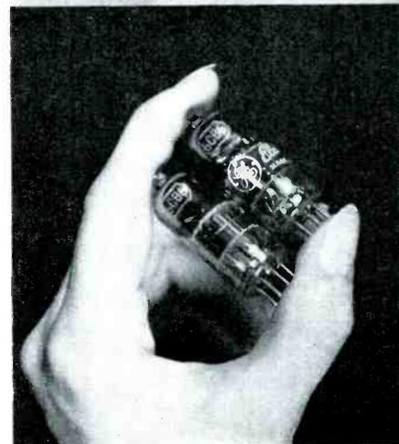
Top: Sylvania's new subminiatures. They are both suitable for Class A amplifier application. Bottom: Two new scanning tubes from G-E. They are capable of operating from a power supply of 120 volts
