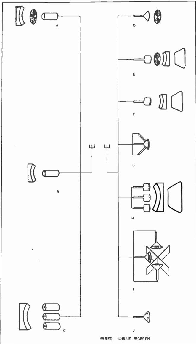
Fig. 1 A—CBS single tube camera, lens, color disc; B—CTI camera; C—RCA 3-tube camera; D—CBS direct view receiver, disc; E—CBS projection set & disc; F—CBS electronic projection; G—Greer tube; H—RCA projection set. I—RCA direct-view receiver; J—Single gun-direct view: to be developed
