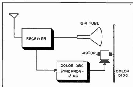
Fig. 6 Block diagram of a CBS-type color television receiver. Observe simplicity, but note also mechanical feature of system
