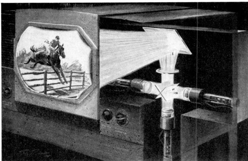
Fig. 5 RCA's color television converter, using small projection picture tubes and refractive optics. This as well as the arrangement shown in Fig. 4 are strictly experimental. They are only two examples of a number of such models
