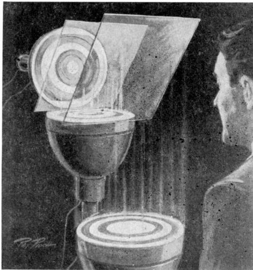
Fig. 4 RCA's direct-view picture reproducing system uses 3 tubes, mirrors which reflect only some colors, let others pass
