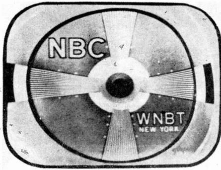
Fig. 1 Horizontal non-linearity, as indicated by non-circular circles
