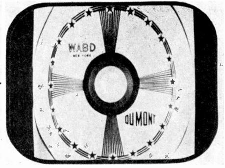
Fig. 3 Elliptical pattern—shows incorrect size rather than non-linearity
