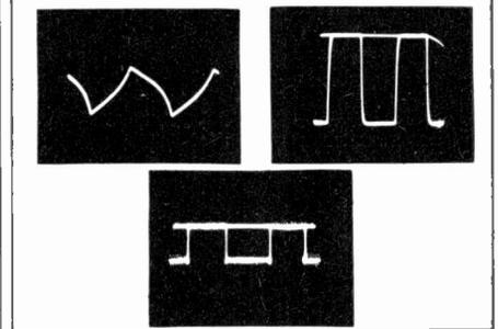
Square and modified square wave patterns appear in chapters on Audio Frequency Circuits and TV Receiver servicing. Book covers square wave testing in detail
