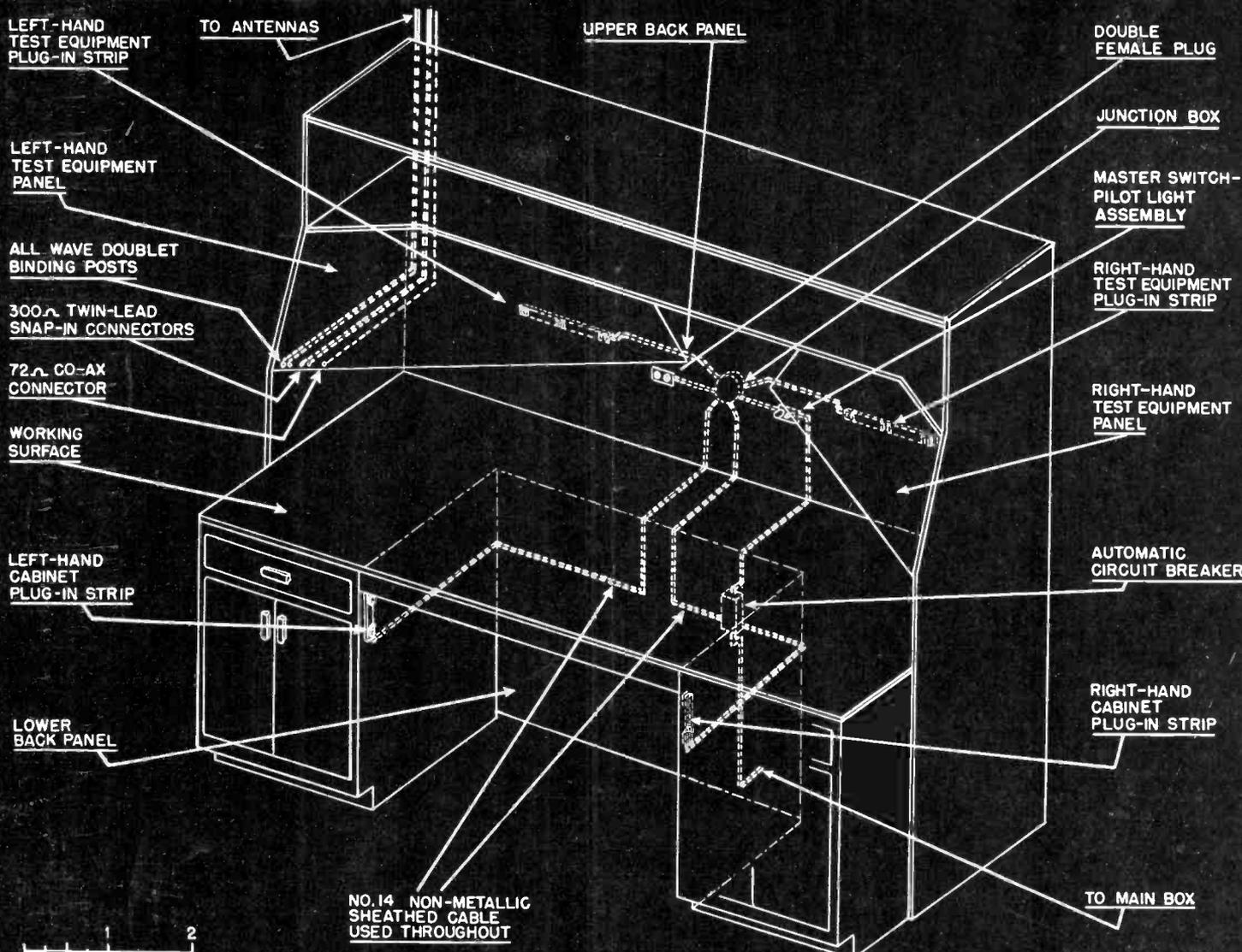
WIRING DIAGRAM OF BENCH
