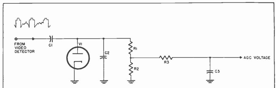
Fig. 1 Simplified diagram of a-g-c circuit. V1 conducts when the positive peaks of the sync signals are applied to plate. Voltage across C2 remains constant
