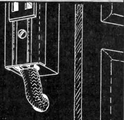
DETAIL OF RIGHT-HAND CABINET PLUG-IN STRIP. CABLE COMES THROUGH SIDE OF CABINET TO STRIP
