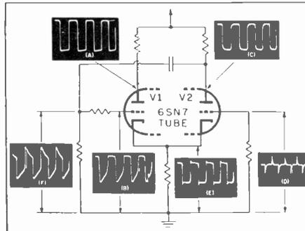
Photographs of plate, grid, and cathode waveform in typical cathode-coupled symmetrical multivibrator. This is taken from chapter on Linear Time Bases
