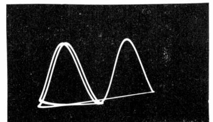
Top: Ionization potential (A) & relaxation oscillations (B) with normal sync. Ionization potential (C) & sawtooth signal (D) due to oversync. Bottom oscillogram of oversync sawtooth sweep (left), resultant sine wave distortion (right)
