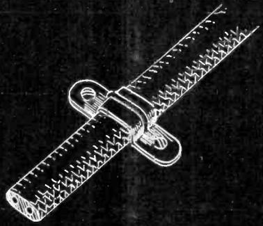
DETAIL ILLUSTRATING METAL STRAP USED TO MOUNT CABLES.
