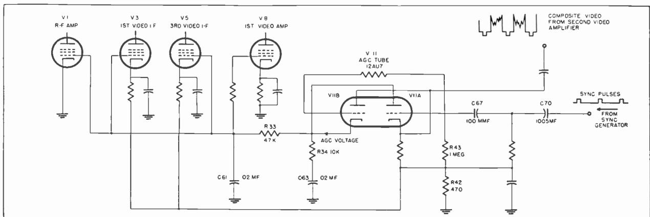
Fig. 4 Variation of keyed a-g-c in Motorola TS-16 and TS-30 chassis. Keying pulse is positive sync pulse from sync separator
