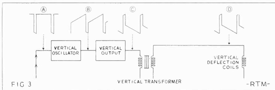
Test points and the proper waveforms to be found in the vertical deflection circuit.
