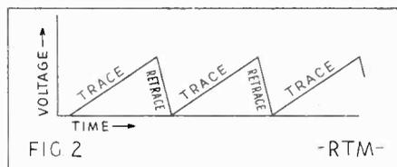
Approximate voltage waveform on one of a pair of the deflection plates of an electrostatic tube. Voltage on the opposing plate would be similar, but opposite in polarity.
