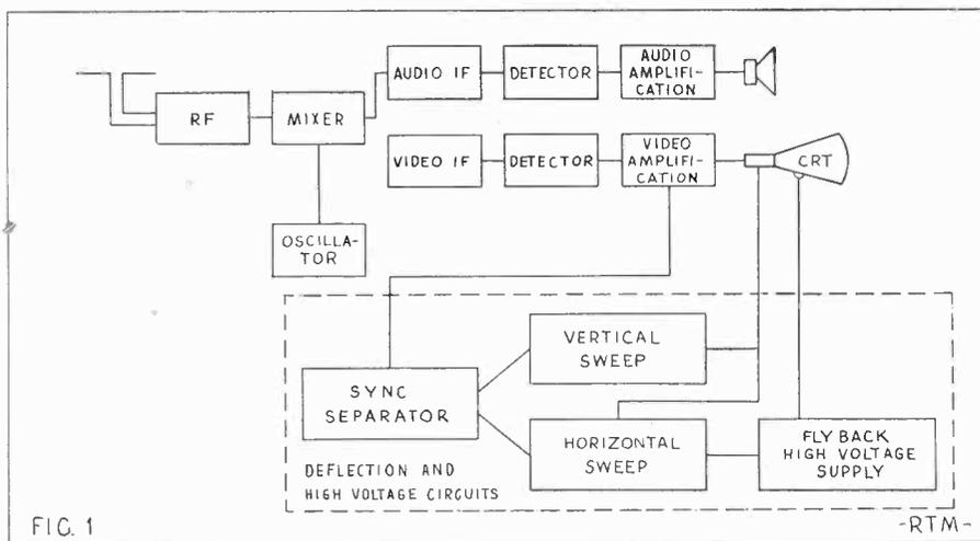
Block diagram of a typical TV receiver employing flyback for the second anode voltage. In this set, brightness of the picture depends on proper operation of the horizontal sweep circuit.
