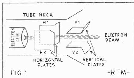
Deflection-plate arrangement in a typical electrostatic-deflection CR tube.
