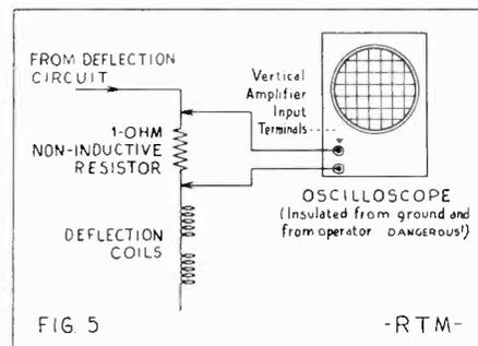
FIG 5 Setup for display of current waveform in analysis of electromagnetically-deflected receiver. Current appears as IR drop across one-ohm resistor.
