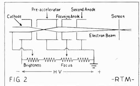
Connections for the "zero-first-anode-current" electron gun, commonly found in the newer tubes using electrostatic focusing.
