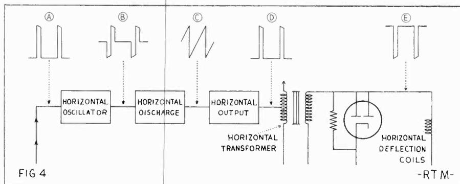
FIG 4 Test points and waveforms in signal tracing of horizontal circuit. Waves shown are "ideal," and may correspond only approximately to those found in actual practice. Settings on the scope are the same as for test of vertical circuit, except for sweep frequency adjustment.
