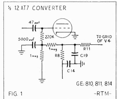
Circuit change in the front end of a typical receiver design, to eliminate 60 cycle buzz (see text).
