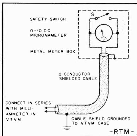
Circuit connections for adapting the VTVM for millivolt measurements. When warmed up, the DC microammeter used by the author drifted from calibration less than 1/50 of the full scale.
