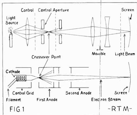
Comparison between the electrostatic focusing system and an optical system. Electrons are focused similarly to light rays, using charged electrodes in place of lenses.
