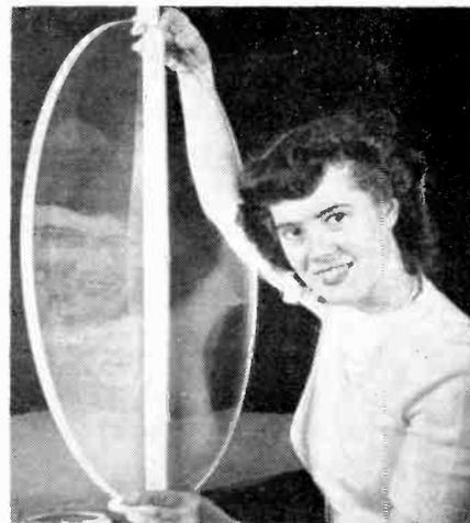
to perfect focus on the photographic plate. The theater TV system uses the same principle in reverse, to project a television image from a spherical mirror without distortion or imperfect focus around the edges.
