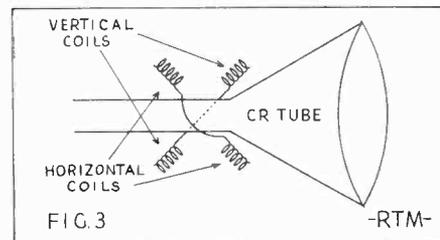
Schematic representation of deflection coils on the neck of a magnetic-deflection picture tube.
