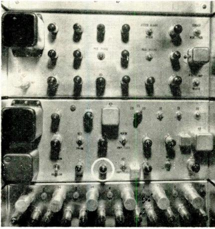
Part of the Phonevision coder at the transmitter. The "heart" of the system, the random-noise tube, is circled.
