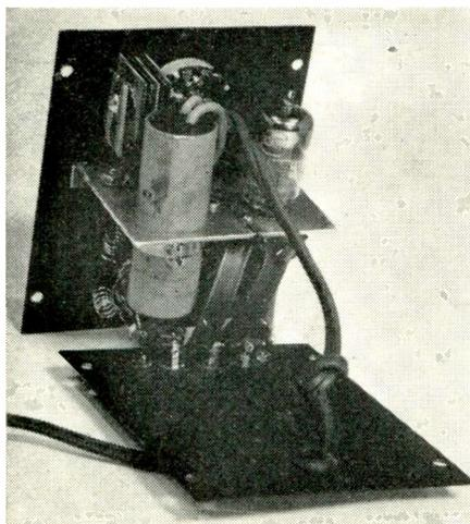
Parts arrangement in a typical all-channel TV booster. Note selenium rectifier and use of a single tube, a duo-triode used for two-stage amplification.
