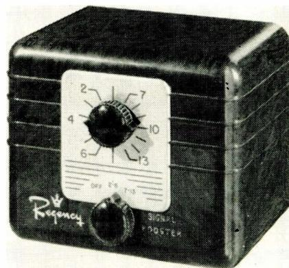
The unit contains contra-wound bifilar coils with push-pull triode connections for balanced output. Internal impedance match accommodates either 300-ohm twinlead or 72-ohm coaxial line. Bandwidth, according to the maker, I. D. E. A., Inc., is sufficiently wide for satisfactory operation on 12 channels.
