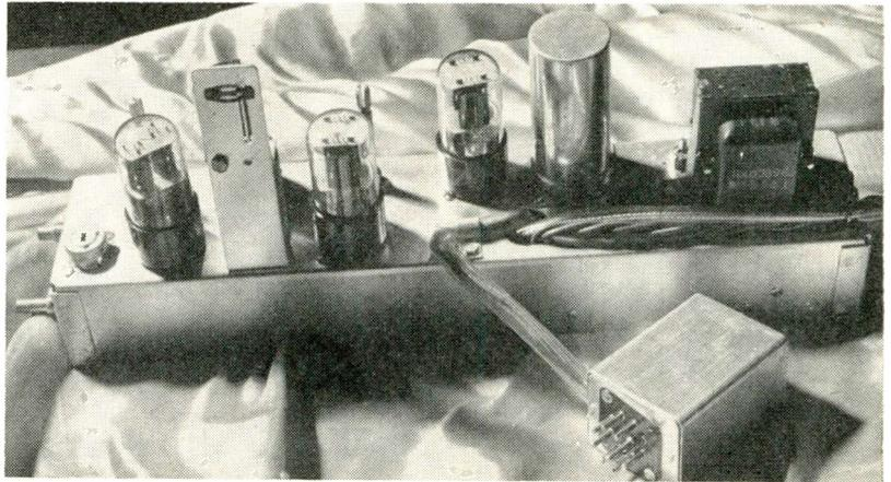
The Phonevision decoder unit, which is attached to the chassis of the subscriber's TV set. This supplementary unit is shown as part of the receiver block diagram below.
