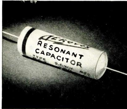
425-485 Kc range, is achieved by winding sections of the foil so that inductance is increased. With a certain placement of the tabs, the resonance is controlled to fall in the IF band.
