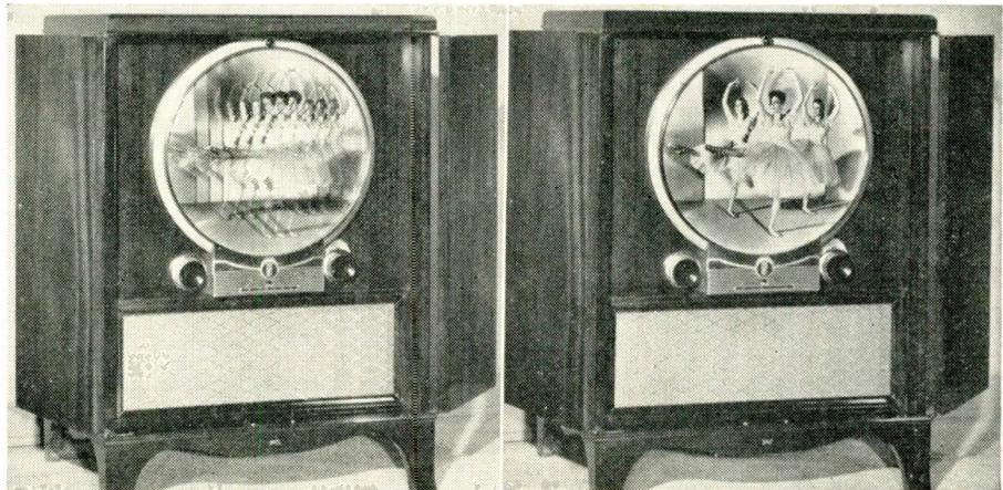
The scrambled TV picture as it is received without the decoding signal is shown at left. Video information and horizontal sweep are out of phase part of the time, producing a picture which shifts back and forth horizontally. Right, normal picture when the decoder is operating.
