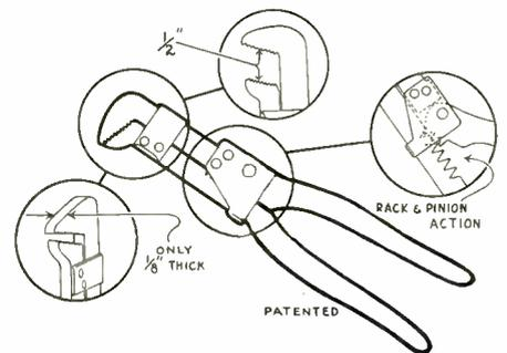
nated the "Power-Grip," the tool has an angle head, to afford heavy pressure in ordinarily inaccessible spots. Thickness of the head is ⅛ inch, while the wrench's overall length is 5¼ inches. The jaw opening ranges from zero to more than ½ inch.
