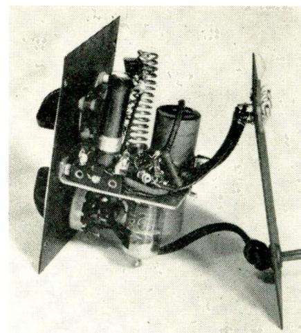
Under-chassis view of the booster. Twelve-position selector switch can be seen, with coils attached. Short connecting leads are particularly important in replacing any parts of TV boosters, since losses and noise are easily introduced.
