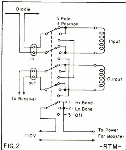
second wafer has two poles and three positions. All the wiring necessary for these switching operations is likely to result in more losses. In spite of this, however, the amplifiers will still have useful gain.
