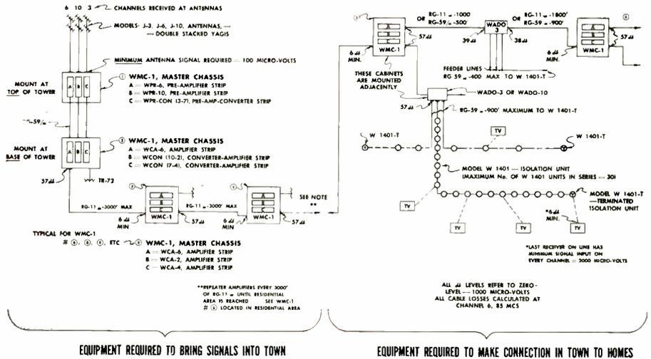
Block diagram of the Jerrold Antenna system installation for a town. At present, the system delivers a maximum of three channels, with an individual amplifier strip for each channel in each repeater-amplifier unit.
