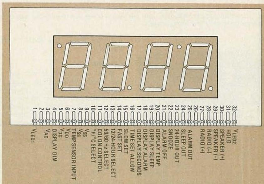
FIG. 1—THE COMPLETE PIN-OUT for the National MA1026 clock module is shown here.
