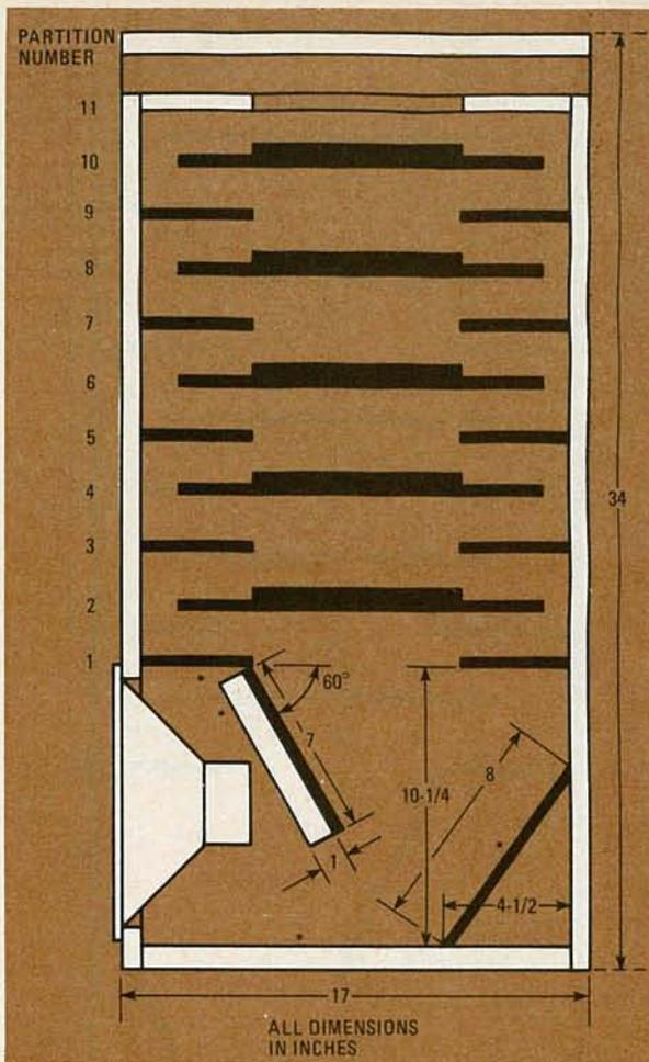
FIG. 6—SIMPLIFIED CUTAWAY VIEW of enclosure showing mounting details of first and second behind-the-speaker partitions.
