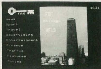
FIG. 17—THE ALPHA-PHOTOGRAPHIC mode allows photographs to be included as part of the videotex material. The picture shown took about two seconds to transmit.
