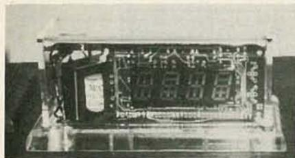
FIG. 4—THIS IS HOW the project will look when it is finished. The clear case—an acrylic butter dish—makes the clock more interesting visually.
