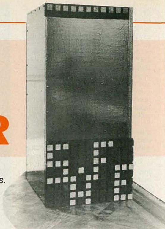
IN THE DECEMBER 1981 ISSUE, **RADIO-ELECTRONICS** PUBLISHED plans for constructing a speaker that used the SAFE (Symmetrical Air Friction Enclosure) principle (U.S. patent no. 4,168,761, other patents pending) to obtain good sound from a small enclosure. This article dealt with a companion subwoofer using the SAFE principle that provides extended bass response from a relatively small enclosure.
