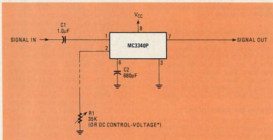
\*ATTENUATION PROPORTIONAL TO VOLTAGE AT PIN 2 WHEN  $3.5\text{VDC} < V_C < 6.0\text{VDC}$ , OR PROPORTIONAL TO RESISTANCE FROM 0 TO 33K OHMS
