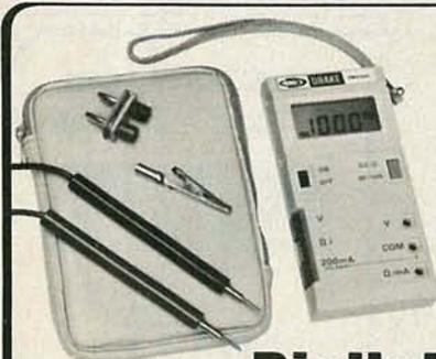
The Drake DM2350 Digital Multimeter is a convenient, small handheld liquid crystal display meter ideal for the serviceman or hobbyist. This 3 1/2 digit meter is auto-ranging, auto-zeroing, has polarity indication, and an over-range warning signal. Battery life is greater than 300 hours with a "low battery" indicator. A continuity test sounds a signal when circuit resistance is less than 20 ohms. Dc accuracy is a basic 0.8%.
