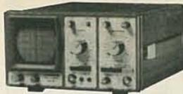
The HM307 is a compact light weight single trace oscilloscope which has been specially designed to meet the requirements of both the service technician and advanced amateur. A principal feature of the HM307 is the built-in component tester. It allows both passive and active components to be tested while still in-circuit for more cost effective servicing.
