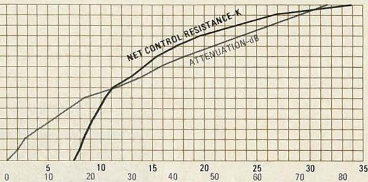
FIG. 3—NET CONTROL RESISTANCE and calculated attenuation plotted against four-bit control signals. Note that the calculated attenuation curve is nearly, but not quite, linear.
