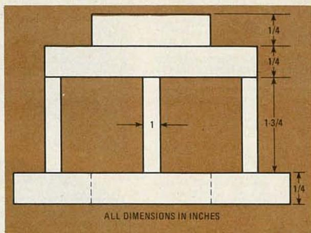
FIG. 11—SIDE VIEW of even-numbered partition mounted atop odd-numbered partition using partition mounting strips. Each strip is located as shown in Fig. 10 and measures  $1 \times 1 \times 1/4$  inches.
