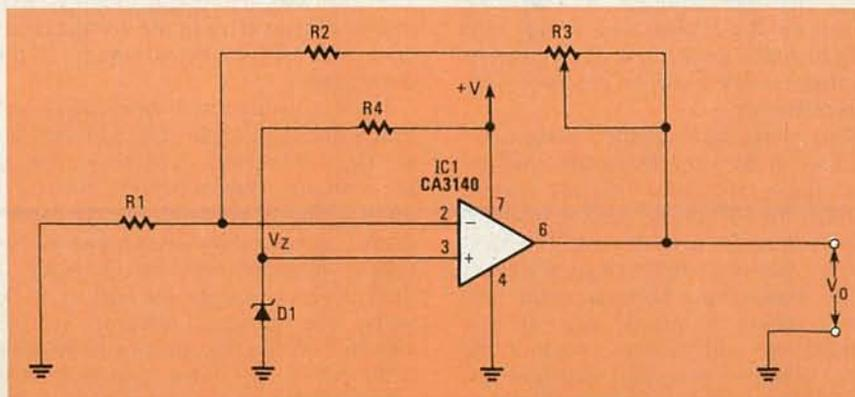
FIG. 4—AN OPERATIONAL AMPLIFIER can be used to scale the voltage from the Zener diode to whatever value is needed.
