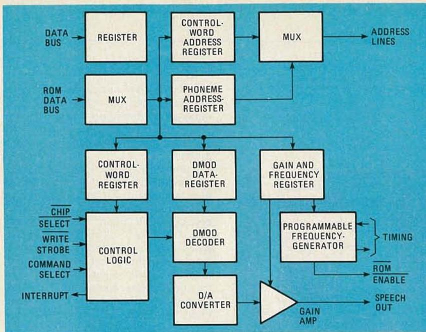
FIG. 2—NATIONAL SEMICONDUCTOR'S DIGITAL TALKER has a fixed vocabulary in ROM; several different ROM's are available. Programmable frequency-generator (lower right) is used to add inflection to speech.
