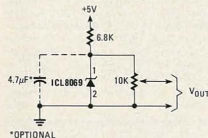
FIG. 7—A 1.2-VOLT temperature-compensated voltage reference, the Intersil ICL8069 used in this circuit is well suited to high-speed A/D and D/A converter projects.
