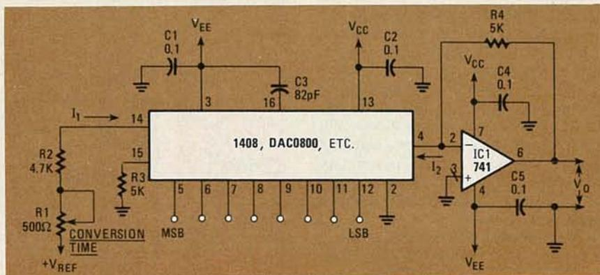
FIG. 12—A DIGITALLY SELECTABLE voltage reference. Once the input current ( $I_1$ ) to the D/A converter is set, the output from the circuit ( $V_0$ ) is determined by digital input (pins 5-12) to the D/A converter.
