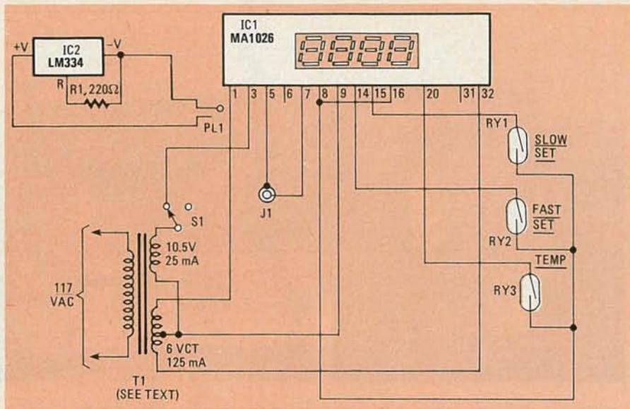
FIG. 2—SCHEMATIC DIAGRAM of the digital clock/thermometer and the temperature sensor. To make the temperature sensor, mount IC2 and R1 on a small piece of perforated construction board.
