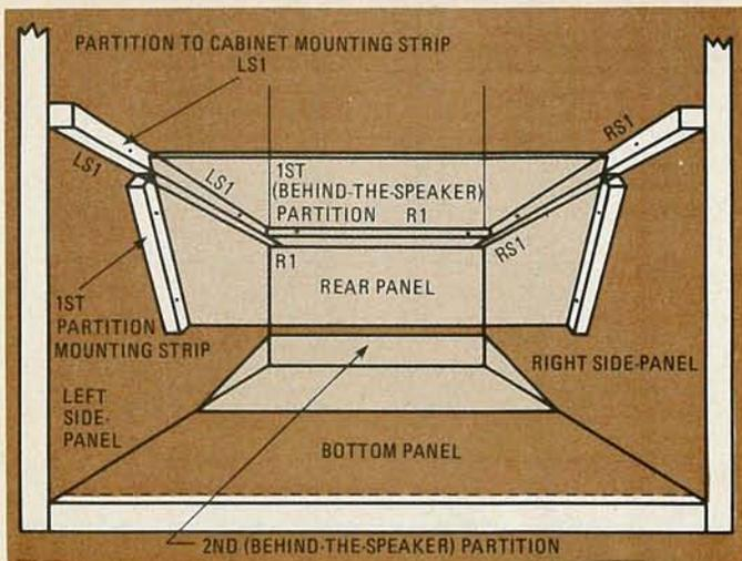
FIG. 4—EXAGGERATED PERSPECTIVE VIEW of first chamber. Note mountings of first and second behind-the-speaker partitions.
