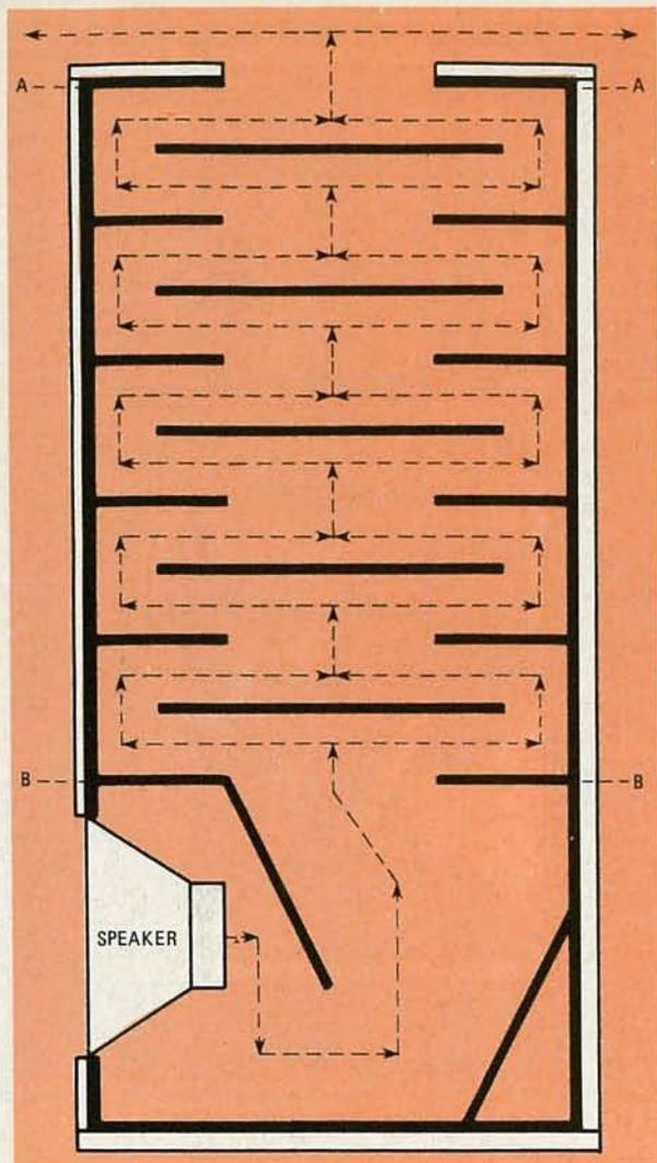
FIG. 1—SIDE VIEW OF SAFE ENCLOSURE showing speaker back-wave path. Path is symmetrical between points A and B.
