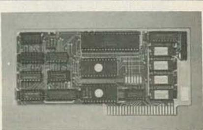
**The Microbuffer II** is an intelligent buffered parallel printer interface for the Apple II computer. Includes 16K of on-board RAM. Buffer memory size is user expandable to 32K. Compatible with Applesoft, CP/M, and Pascal. Includes advanced high resolution graphics print routines for the Epson MX-80 with Graphtrax, Anadex, IDS Paper Tiger, NEC Prowriter. Price: \$259. Contact Practical Peripherals, Inc., 31245 La Baya Dr., Westlake Village, Calif. 91362 (213) 706-0339.
