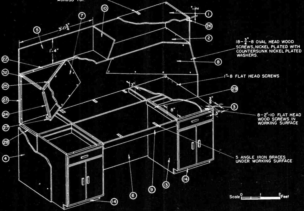
18- $\frac{3}{4}$ "-8 OVAL HEAD WOOD SCREWS, NICKEL PLATED WITH COUNTERSUNK NICKEL PLATED WASHERS.
