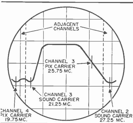
Fig. 2 Typical video i-f response curve
