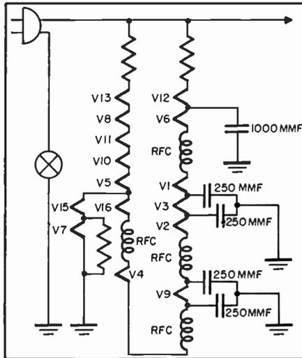
Fig. 3 Filament hook-up in the Motorola VT-71. Filaments are hooked up in series parallel circuit across line
