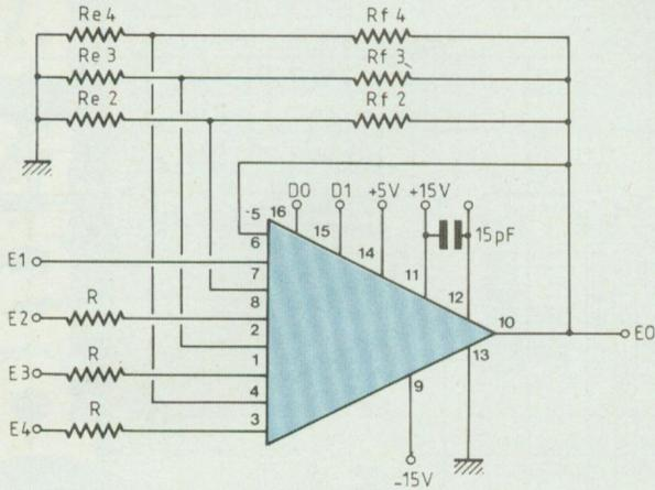
$$\text{Gain} = \frac{R_e + R_f}{R_e}$$
