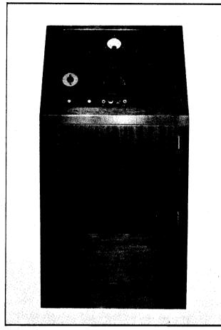
FIG. I—Front view of the experimental crystal-controlled diathermy unit. Apparatus on the panel includes, autotransformer control, PA plate meter, output tuning control, interval timer, PA plate tuning control, output jacks, output indicator lamp, oscillator and doubler tuning controls (screwdriver adjustment), power switches and pilot lamps.
