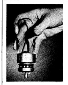
The Eimac 4X150 tube extractor may be used as pictured for inserting or extracting the 4X150A, 4X150D and 4X150G from normal or deep cavities. The prongs of the extractor are placed through the radiator of the tube and permit quick handling of tubes. The spring steel construction allows the tube to be gripped firmly without scoring the cavity walls. Only normal cavity wall clearance is required.
