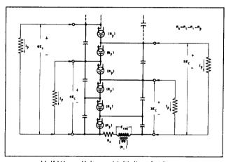
e. Half-Wave Voltage Multiplier (with common ground when  $R_s$  is inserted on the "high" side of  $E_{rms}\big)$
