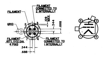
NOTE:—The grid terminal on the new 450TH and TL type tube is now .563" in diameter. To accommodate existing equipment which uses the 450TH or TL tubes with the old style .098" grid terminal, an adaptor pin is provided. This adaptor pin, if not needed, may be removed by unscrewing.
