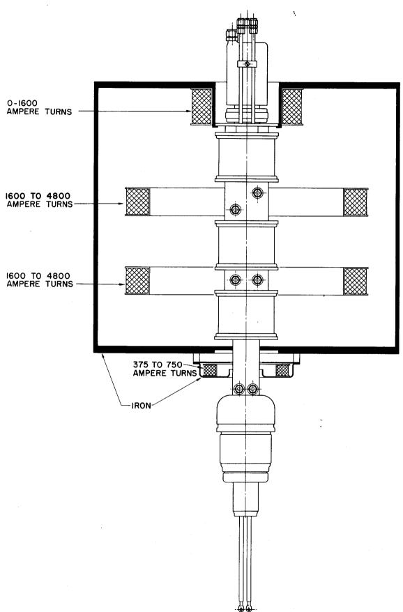
MAGNETIC CIRCUIT SCHEMATIC FOR 3K20,000LK
