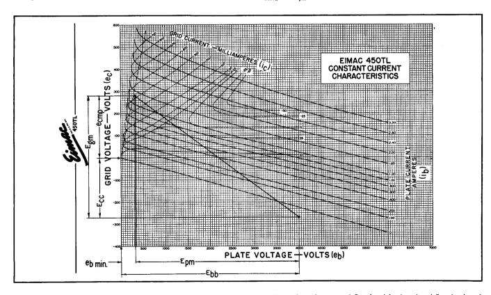
Figure 3. Method of determining  $\mathbf{e}_{emp}$  and  $\mathbf{i}_{e}$  on 450TL constant-current characteristics from values of  $\mathbf{e}_{bmin}$  and  $\mathbf{E}_{pm}$  found in steps 6 and 7 and value of  $\mathbf{i}_{b}$  found in step 10. The value of  $\mathbf{E}_{ee}$  and  $\mathbf{E}_{gm}$  from steps 13 and 14 and the operating line are also shown.
