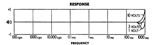
Input Impedance and Frequency Response of an Eimac 2-01C operating in a Hewlett-Packard Model 410B Vacuum Tube Voltmeter.
