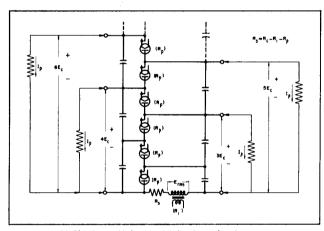
e. Half-Wave Voltage Multiplier (with common ground when  $R_s$  is inserted on the "high" side of  $E_{\rm rms})$
