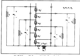
Half-Wave Voltage Multiplier (with common ground when R<sub>s</sub> is inserted on the "high" side of E<sub>rms</sub>)
