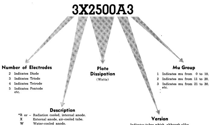
Indicates tubes which, although alike as to the number of elements and plate dissipation, are not necessarily interchangeable either electrically or physically.
