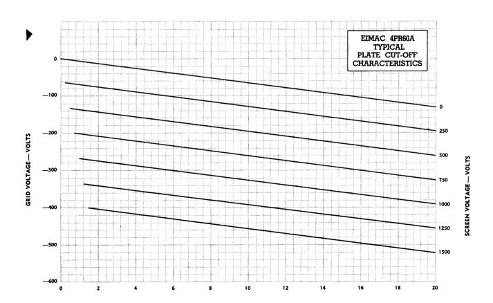
PLATE VOLTAGE --- KILOVOLTS
