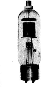
Temperatures in excess of 60° C limit the peak-inverse rating to 5,000 volts with a corresponding reduction in permissible RMS supply voltages to one-half those listed in the table.
