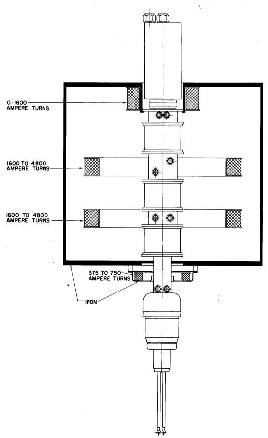
MAGNETIC CIRCUIT SCHEMATIC FOR 3K50,000LK
