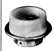
For chassis mounting, a 2¼" diameter hole should be cut into the deck and the socket secured by the three toe clamps provided.
