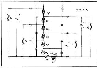
e. Half-Wave Voltage Multiplier (with common ground when Rs is inserted on the "high" side of E<sub>rms</sub>)
