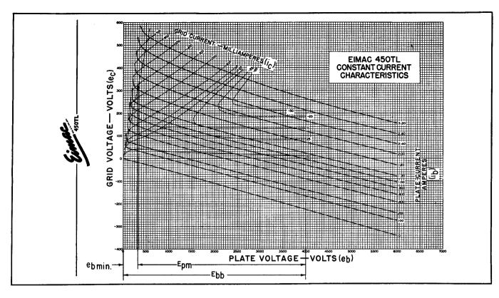
Figure 2. 450TL constant-current characteristics showing method of determining e<sub>bmin</sub> and E<sub>pm</sub> in steps 6 and 7 from value of i<sub>b</sub> obtained in step 5.
