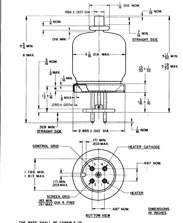
THE BASE SHALL BE CAPABLE OF ENTERING A GAUGE 1/4" THICK HAVING 4 HOLES WHOSE DIA'S ARE 214" AND WHICH ARE LOCATED ON 11/16" CENTERS AND A CENTER HOLE OF .250" DIA.
