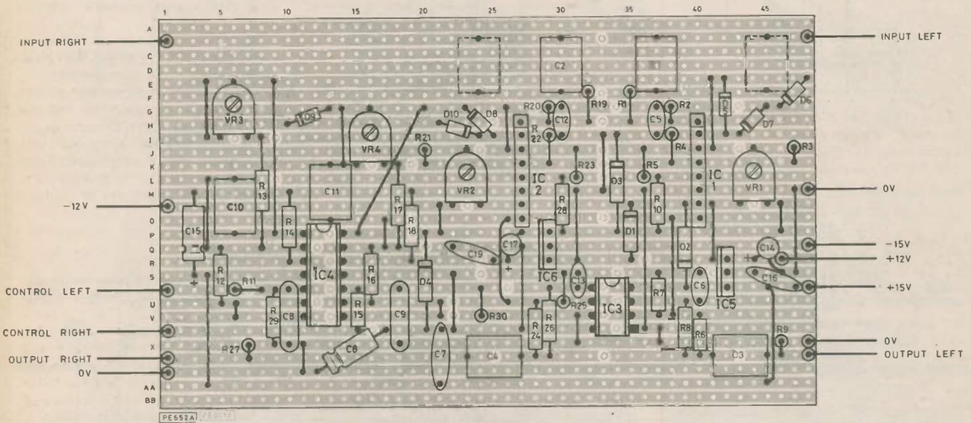
Fig. 10 Stripboard layout of the VCA system
