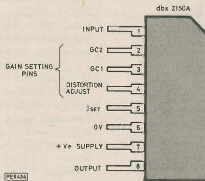
Fig. 1. Pin-out of the VCA
