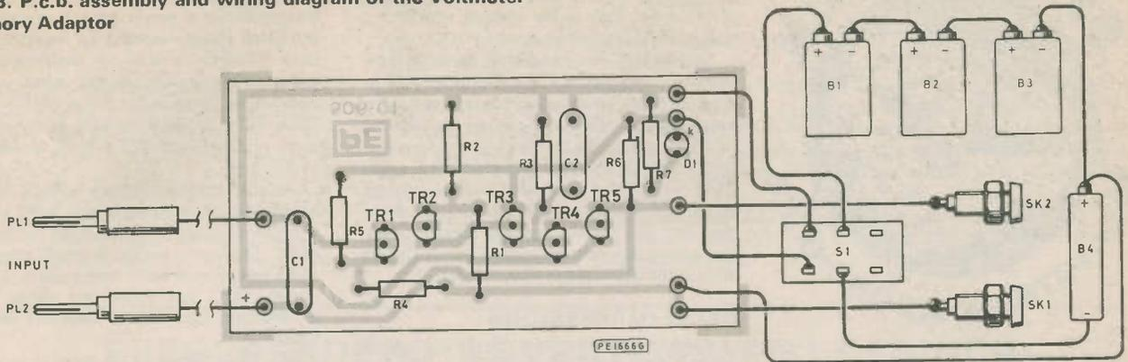
slight misjudgements could cause a problem. The 9V batteries were held in place by suitably adapted P-clips which proved to be satisfactory and the AA size battery was held in place by a purpose made holder.
