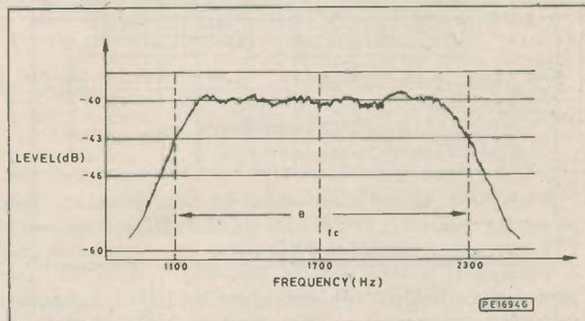
Fig. 12. V.23 spectrum at 1200 Baud
