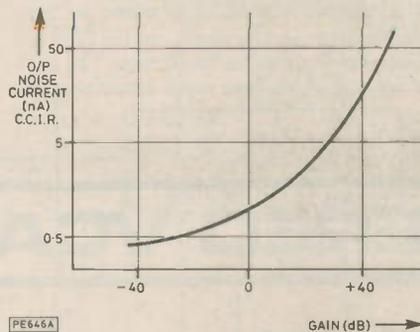
Fig. 5. Effect of gain on output noise current
