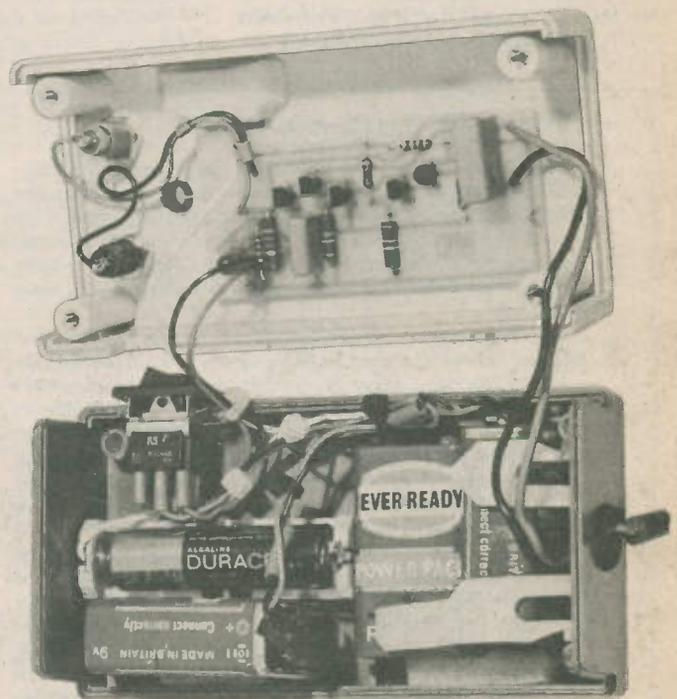
Photo illustrating the internal view of the Voltmeter Memory Adaptor
