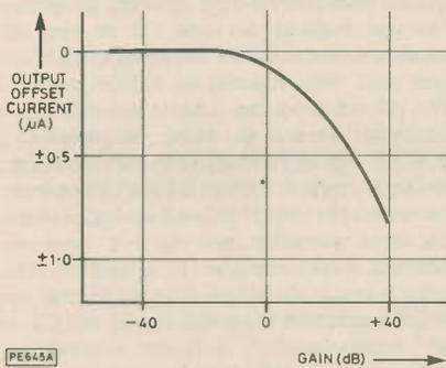
Fig. 4. Effect of gain on output offset current
