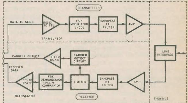
Fig. 2. Basic modem elements
