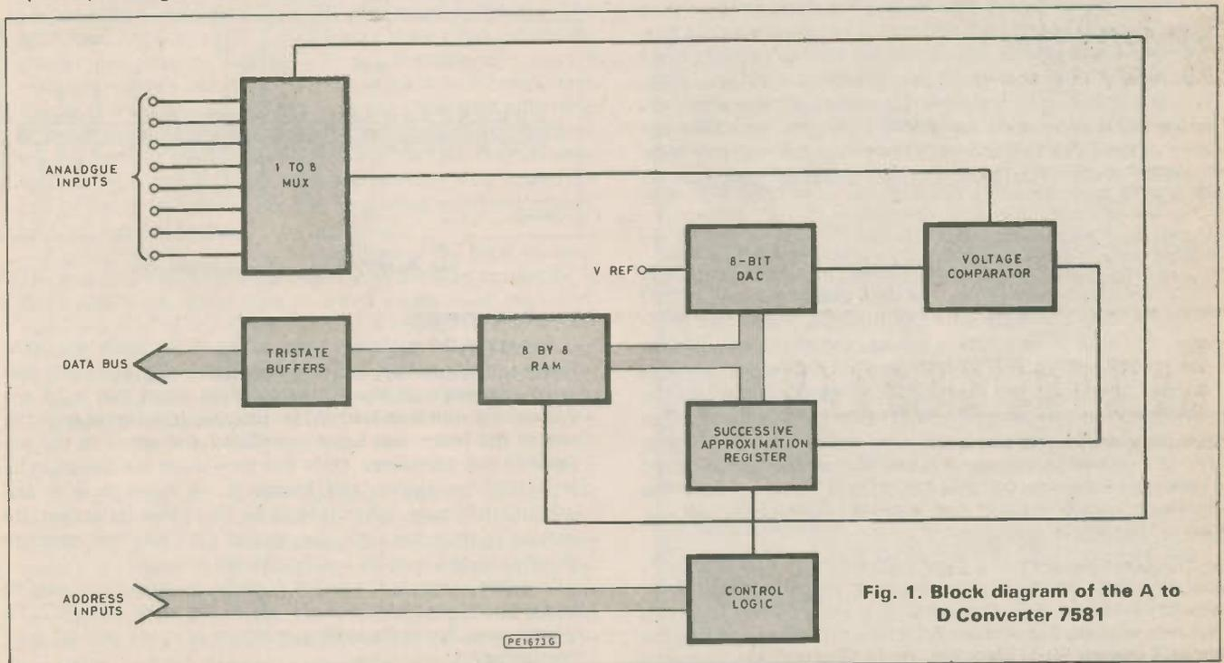
Fig. 1. Block diagram of the A to D Converter 7581
