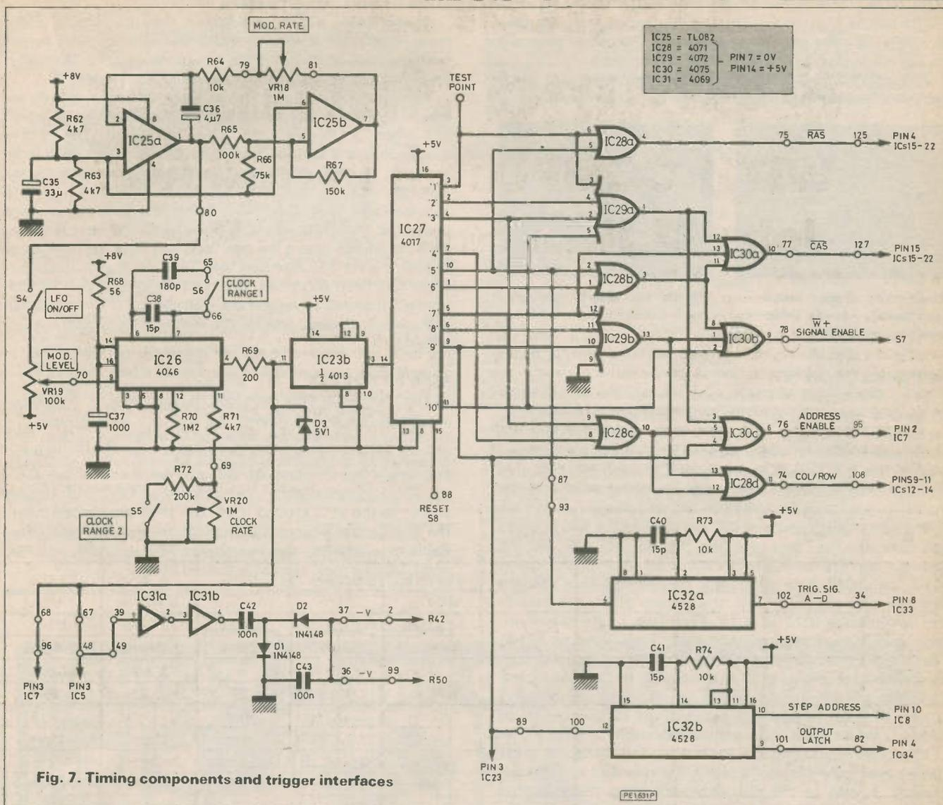
Fig. 7. Timing components and trigger interfaces
