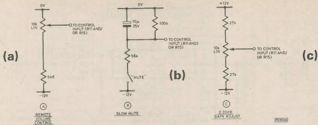
Fig. 9. Examples of simple control inputs. (a) Remote Volume Control, (b) Slow Mute, (c)  $\pm 20\text{dB}$  Gain Adjust
