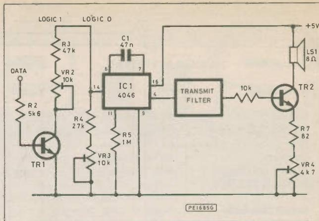
Fig. 4. VCO transmitter section
