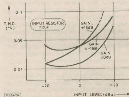
Fig. 6. Distortion vs. input level for different gains (worst case)
