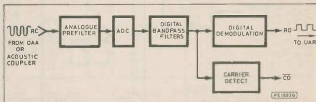
Fig. 10. Am7910 receiver block diagram
