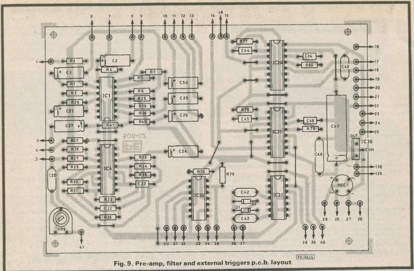
Fig. 9. Pre-amp, filter and external triggers p.c.b. layout
