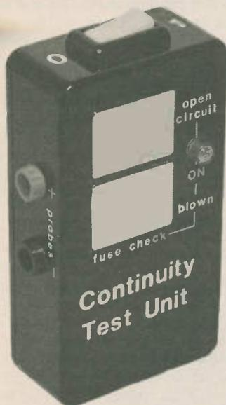
This unit incorporates a buzzer so that short circuits can be easily and quickly detected. Diodes and the majority of electrolytic capacitors can also be checked.
