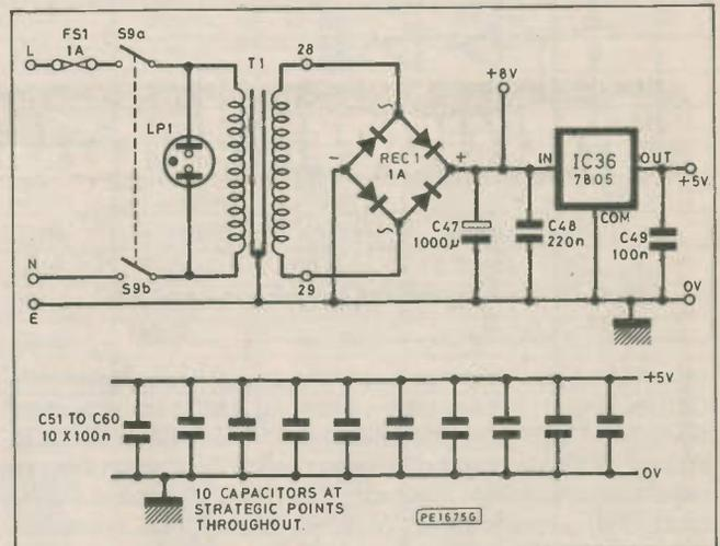
Fig. 8. Circuit diagram of the p.s.u.
