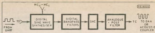
Fig. 9. Am7910 transmitter block diagram
