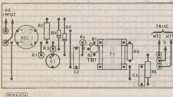
Fig. 5: Layout of components on Veroboard, shown actual size. The triac is mounted separately
