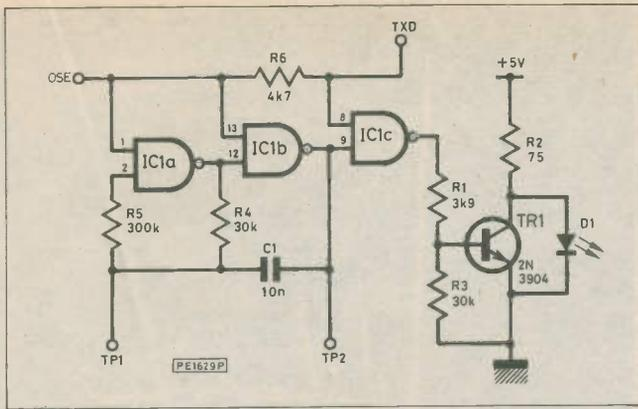
Fig. 1. The transmitter circuit diagram
