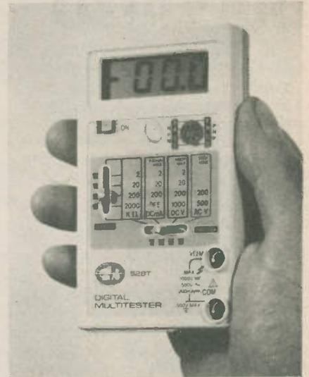
The availability of a very handy,  $3\frac{1}{2}$  digit multimeter has been announced by SSI Ltd. The 528T has a built-in transistor tester and measures just  $115 \times 65 \times 24$ mm. Automatic zero and polarity adjustment are featured along with overload circuit protection.
