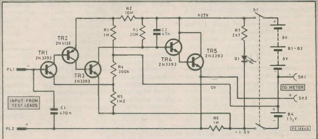
Fig. 2. Full circuit diagram of the Voltmeter Memory Adaptor
