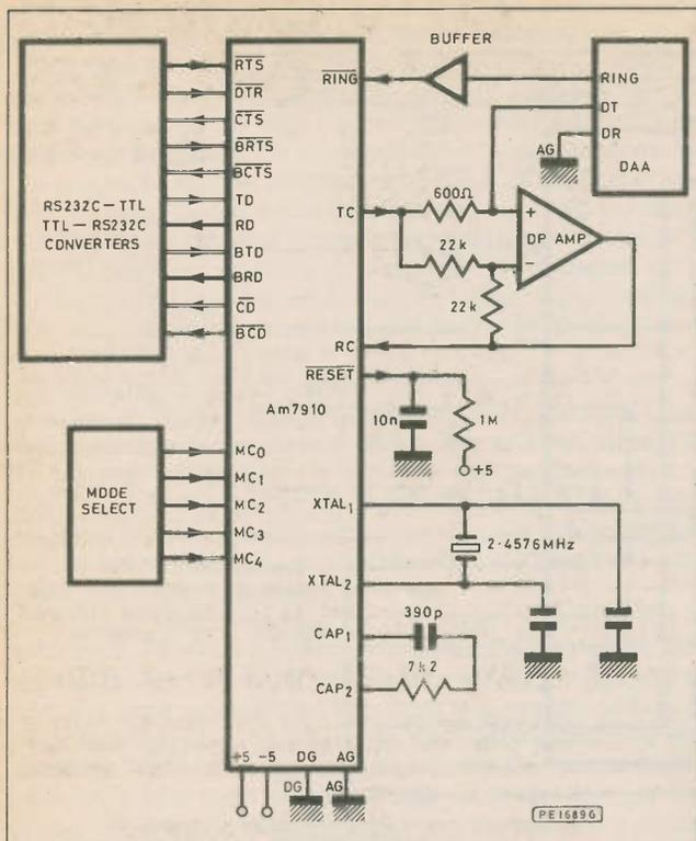
Fig. 8. Multi-mode modem schematic
