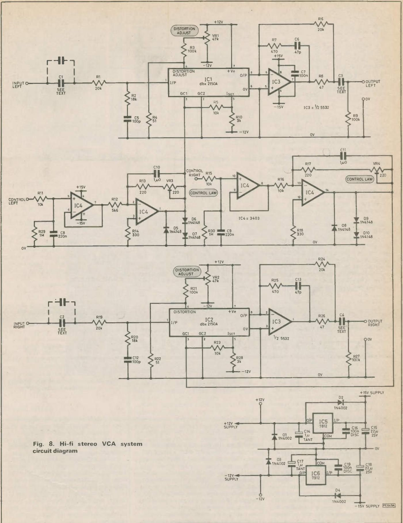
Fig. 8. Hi-fi stereo VCA system circuit diagram
