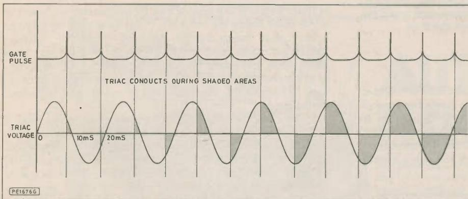
Fig. 2. Representation of the controlled increase in lamp current after switch-on
