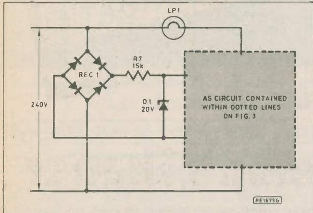
Fig. 4. Alternative additional circuitry for operating 240V a.c. mains lamps. The resistor R7 must be adequately rated for the power dissipation required, and so must the triac
