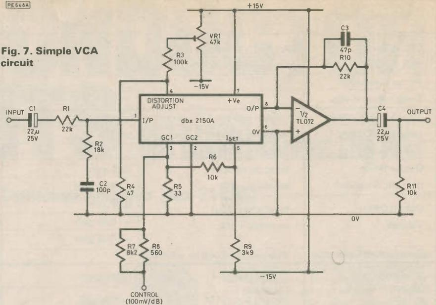
decoupling capacitors, and by the op-amp's feedback capacitor. Also note that the control law is linear volts per dB of gain; in other words, linear control voltage changes produce logarithmic gain changes. Since only 5.9mV of control change is necessary to produce 1dB's worth of level variation, then care must be taken to prevent noise or interference from getting into the control pin. Such effects would immediately manifest themselves as audio noise or distortion.
