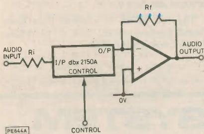
Fig. 3. Basic principle of operation
