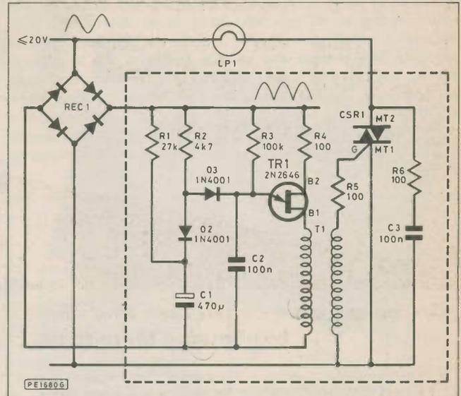
Fig. 3. The circuit for increasing lamp life
