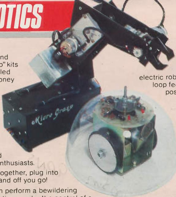
MicroGrasp is a fully programmable electric robot arm with closed loop feedback for positive positioning. The robot can be driven from virtually all micros.
