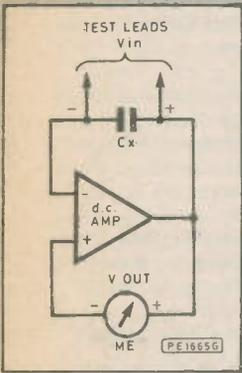
Fig. 1. Block diagram of the Voltmeter Memory Adaptor
